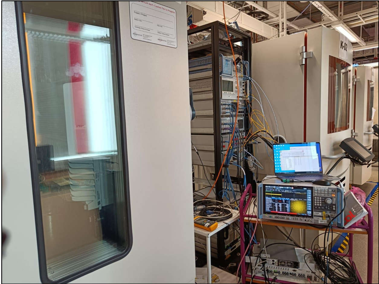
Conducted Test Set Up – Frequency Stability
