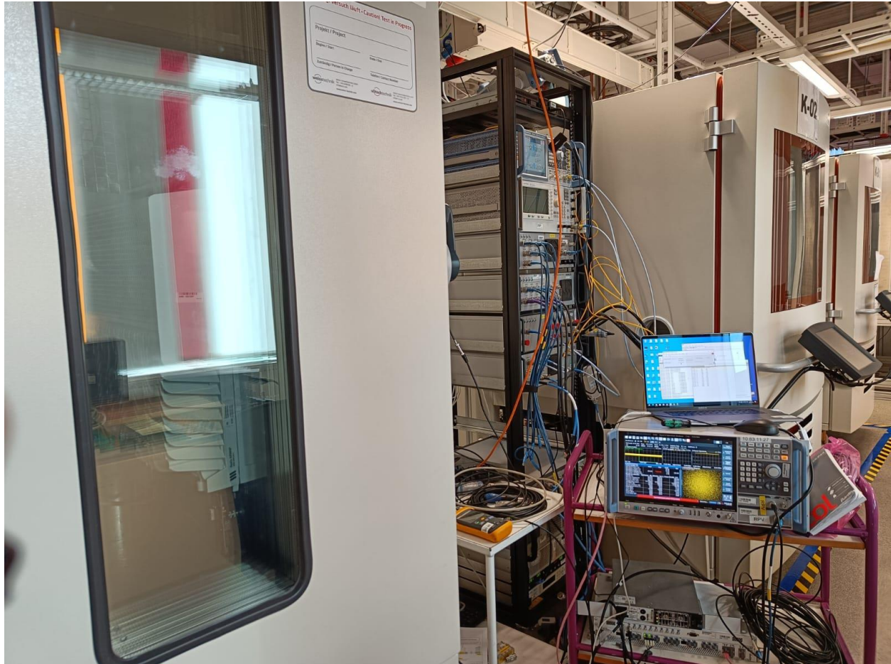
Conducted Test Set Up – Frequency Stability
