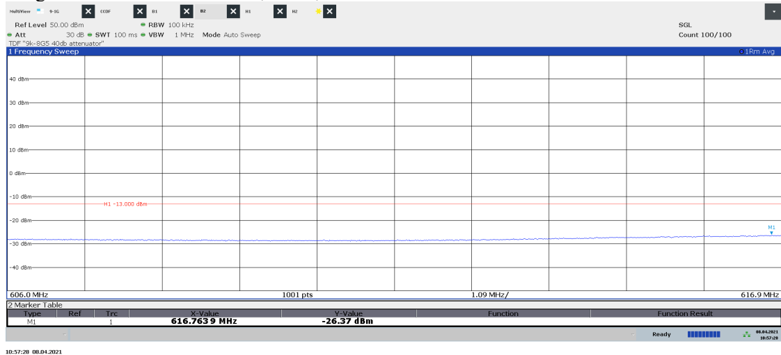
Diagram 2.3b NR: RF1-TM1.1, B 15NR , Port B:
