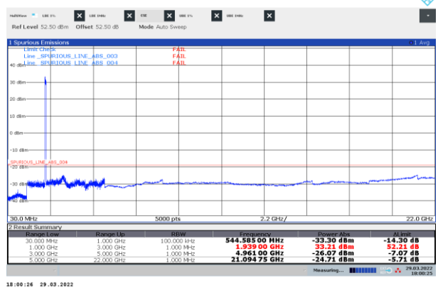
Figure 8.5-16: Conducted spurious emissions of NR 40 MHz two-carrier operation (1 x NR 40 MHz + 1 x NR 25 MHz), top
