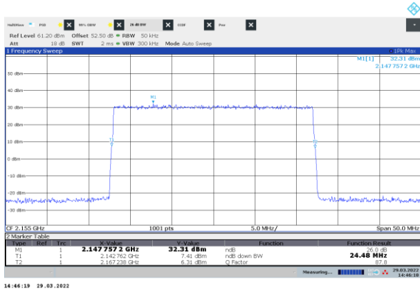
Figure 8.6-1: 26 dB Occupied bandwidth sample plot for NR 25 MHz channel
