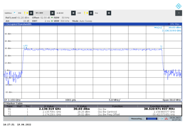
Figure 8.6-6: 99% Occupied bandwidth sample plot for NR 40 MHz channel
