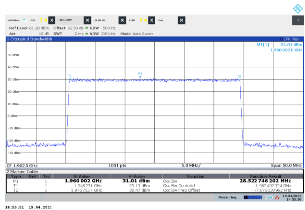
Figure 8.7-4: 99% Occupied bandwidth sample plot for NR 30 MHz channel
