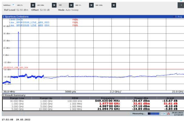
Figure 8.5-13: Conducted spurious emissions of NR 30 MHz two-carrier operation, bottom
