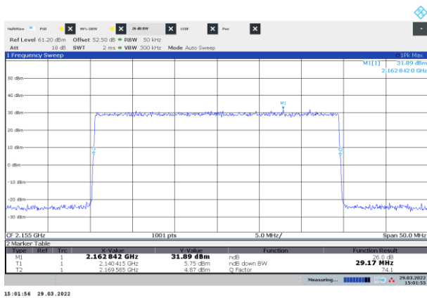
Figure 8.6-3: 26 dB Occupied bandwidth sample plot for NR 30 MHz channel
