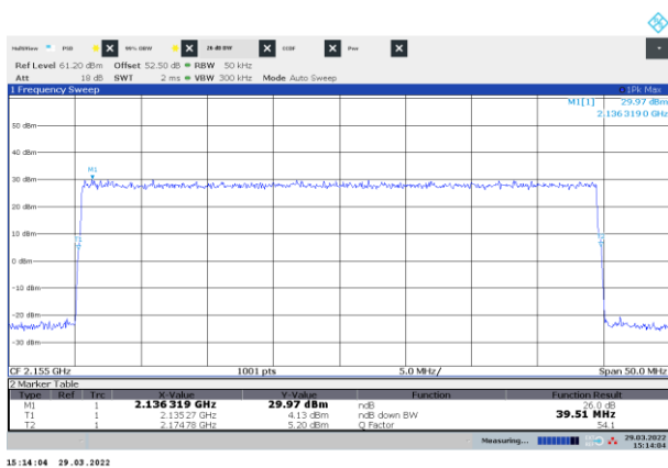
Figure 8.6-5: 26 dB Occupied bandwidth sample plot for NR 40 MHz channel
