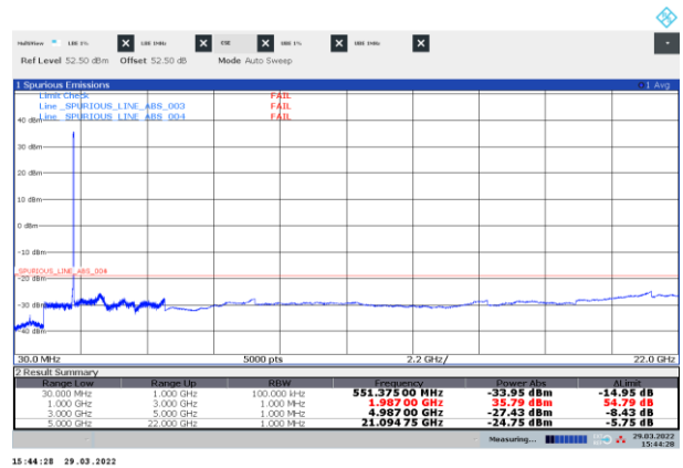
Figure 8.5-6: Conducted spurious emissions of NR 30 MHz top channel, single carrier operation
