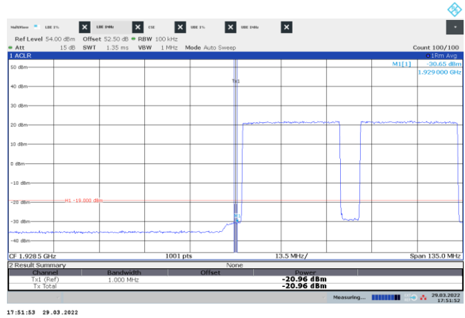
Figure 8.5-41: Conducted emission 1 MHz away from the lower band edge
