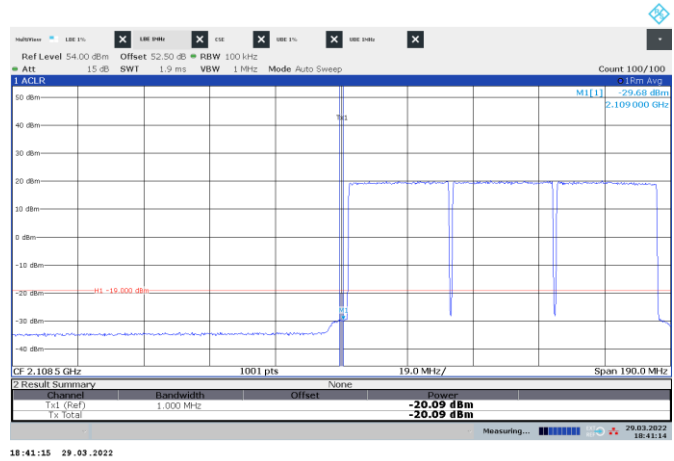
Figure 8.3-56: Conducted emission 1 MHz away from the lower band edge
