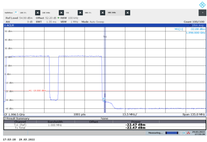
Figure 8.5-43: Conducted emission 1 MHz away from the upper band edge
