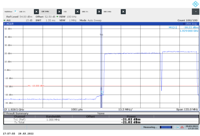
Figure 8.5-45: Conducted emission 1 MHz away from the lower band edge
