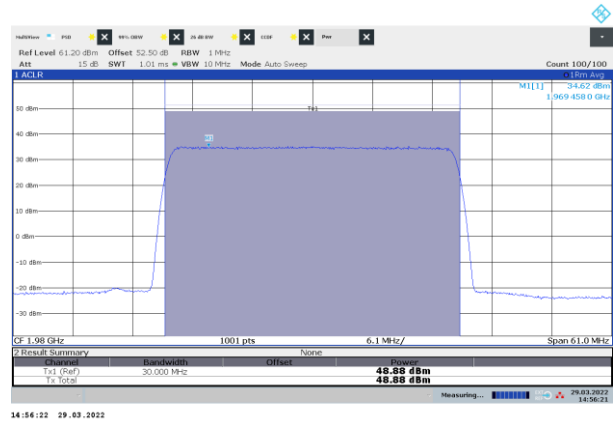
Figure 8.2-18: Power of NR 30 MHz channel bandwidth, single carrier operation, sample plot, top channel
