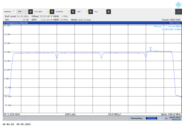
Figure 8.1-12: PSD of NR 25 MHz and 15 MHz channel bandwidth, four-carrier operation (3x 25 MHz + 1x15 MHz), sample plot, mid channel
