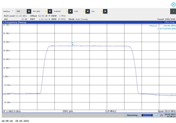
Figure 8.2-3: PSD of NR 25 MHz channel bandwidth, single carrier operation, sample plot, top channel
