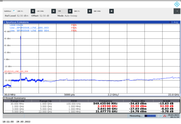
Figure 8.3-12: Conducted spurious emissions of NR 25 MHz two-carrier operation, top
