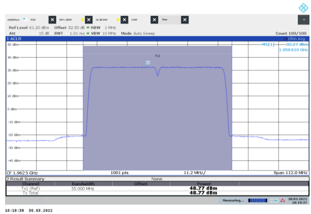
Figure 8.2-22: Power of NR 25 MHz channel bandwidth, two-carrier operation, sample plot, middle channels
