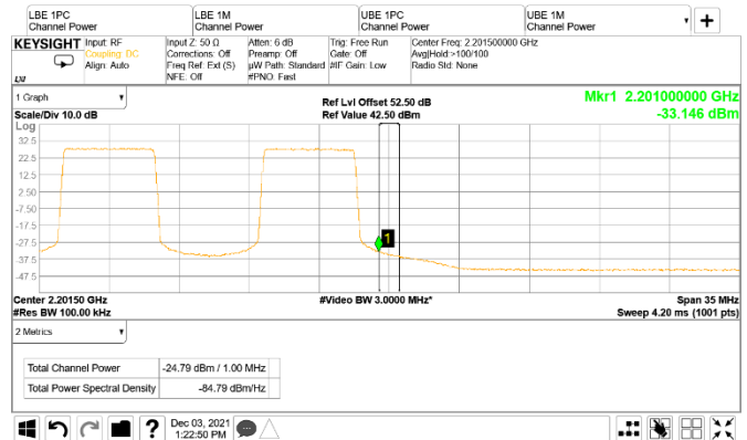
Figure 8.3-49: Conducted emission 1 MHz away from the upper band edge
