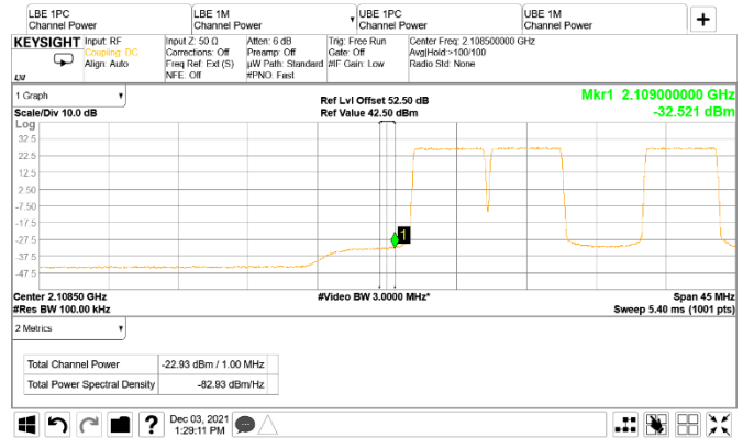
Figure 8.3-51: Conducted emission 1 MHz away from the lower band edge
