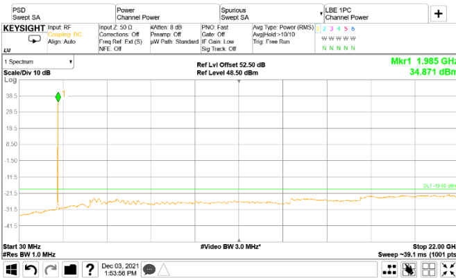
Figure 8.5-15: Conducted spurious emissions of LTE 5 MHz three-carrier operation, top
