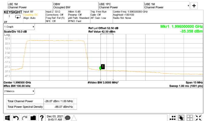
Figure 8.5-54: Conducted emission 1 MHz away from the upper band edge
