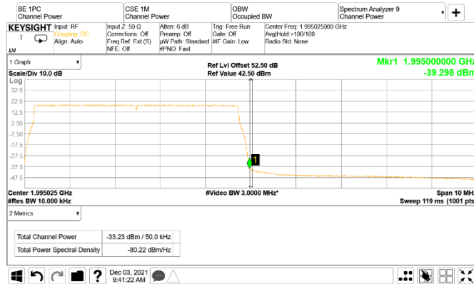
Figure 8.5-33: Conducted emission at the upper band edge
