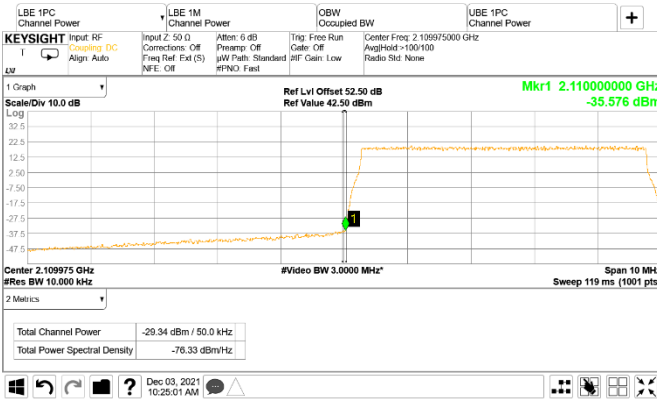
Figure 8.3-54: Conducted emission at the lower band edge
