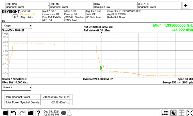
Figure 8.5-41: Conducted emission at the upper band edge
