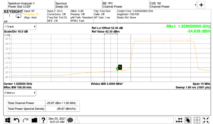
Figure 8.5-32: Conducted emission 1 MHz away from the lower band edge
