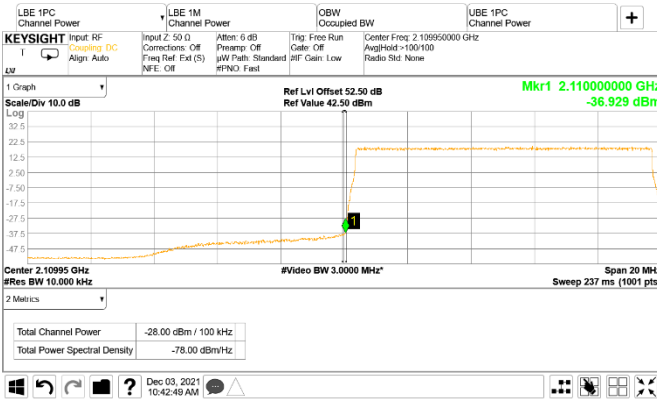
Figure 8.3-58: Conducted emission at the lower band edge
