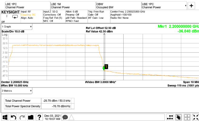
Figure 8.3-56: Conducted emission at the upper band edge
