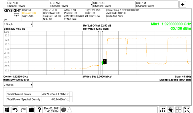
Figure 8.5-48: Conducted emission 1 MHz away from the lower band edge
