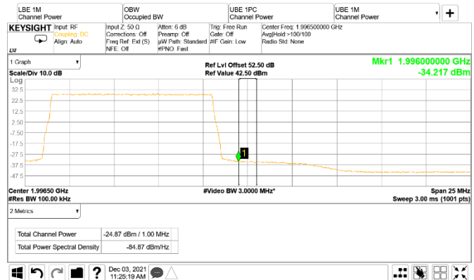
Figure 8.5-38: Conducted emission 1 MHz away from the upper band edge
