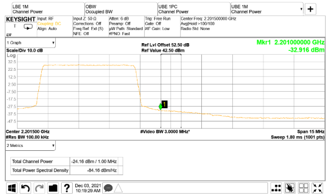
Figure 8.3-57: Conducted emission 1 MHz away from the upper band edge
