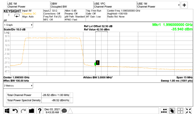
Figure 8.5-34: Conducted emission 1 MHz away from the upper band edge
