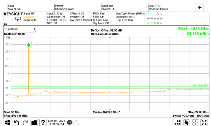
Figure 8.5-12: Conducted spurious emissions of LTE 5 MHz two-carrier operation, top
