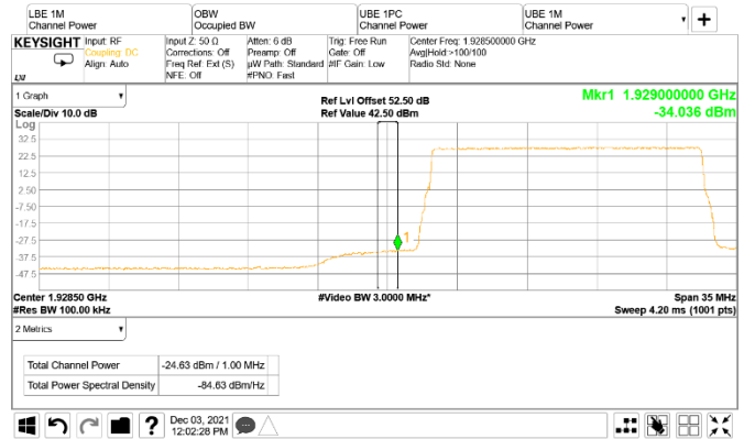
Figure 8.5-40: Conducted emission 1 MHz away from the lower band edge
