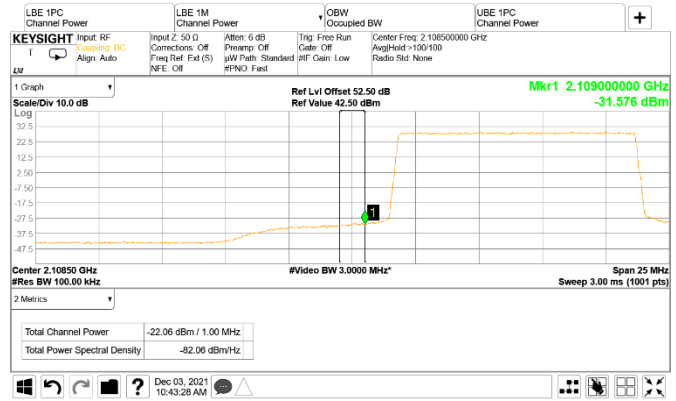
Figure 8.3-59: Conducted emission 1 MHz away from the lower band edge
