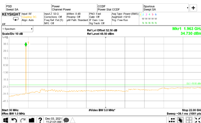
Figure 8.5-5: Conducted spurious emissions of LTE 10 MHz mid channel, single carrier operation
