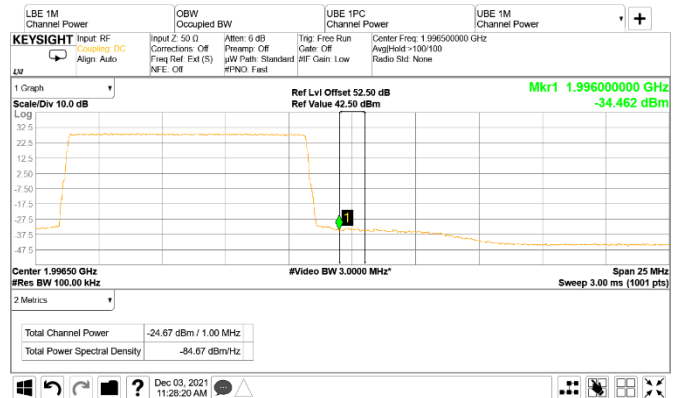
Figure 8.5-58: Conducted emission 1 MHz away from the upper band edge
