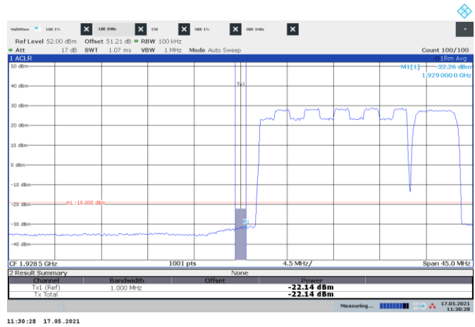
Figure 8.5-330: Conducted emission 1 MHz away from the lower band edge
