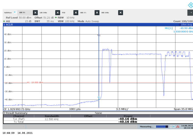
Figure 8.5-355: Conducted emission at the lower band edge
