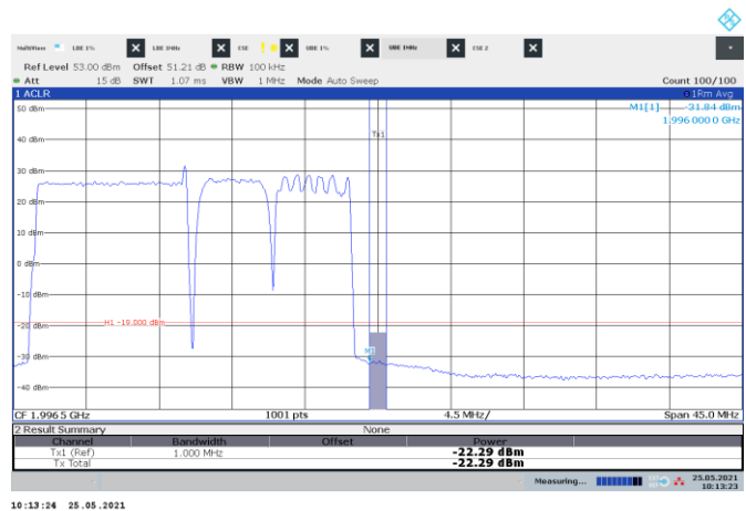
Figure 8.5-376: Conducted emission 1 MHz away from the upper band edge
