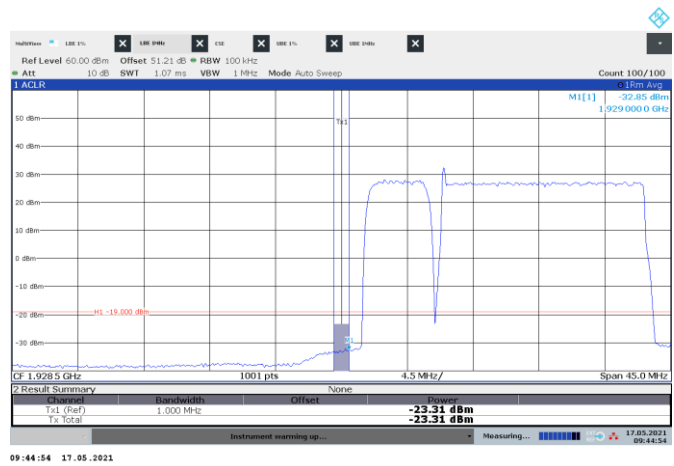
Figure 8.5-350: Conducted emission 1 MHz away from the lower band edge
