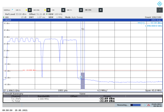
Figure 8.5-368: Conducted emission 1 MHz away from the upper band edge
