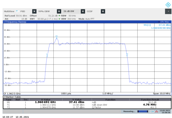
Figure 8.10-2: 26 dB bandwidth sample plot for LTE 5 MHz channel
