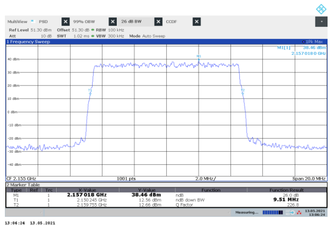
Figure 8.9-4: 26 dB bandwidth sample plot for LTE 10 MHz channel
