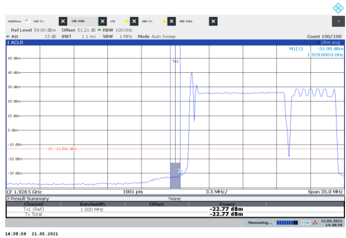
Figure 8.5-358: Conducted emission 1 MHz away from the lower band edge
