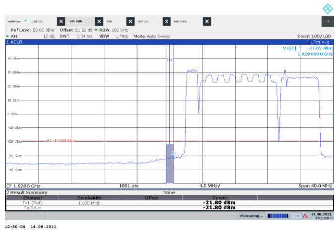
Figure 8.5-360: Conducted emission 1 MHz away from the lower band edge
