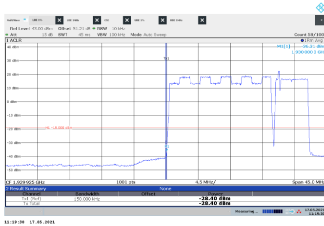
Figure 8.5-309: Conducted emission at the lower band edge
