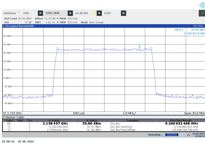
Figure 8.9-11: 99% Occupied bandwidth sample plot for NR 10 MHz channel
