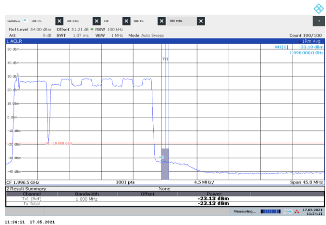
Figure 8.5-312: Conducted emission 1 MHz away from the upper band edge
