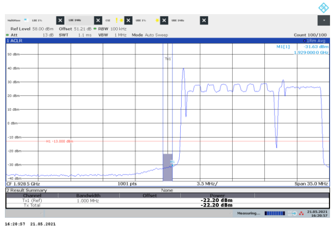
Figure 8.5-354: Conducted emission 1 MHz away from the lower band edge
