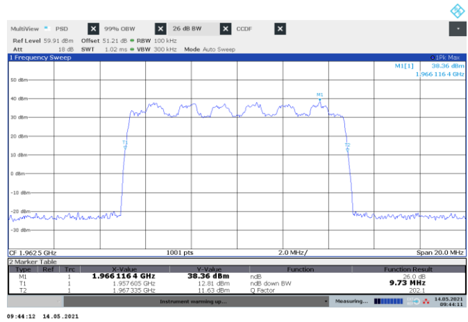
Figure 8.10-12: 26 dB bandwidth sample plot for NR 10 MHz channel
