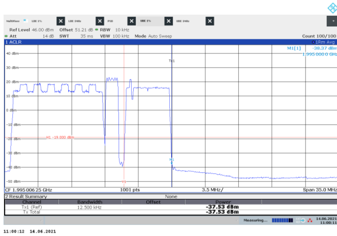
Figure 8.5-365: Conducted emission at the upper band edge
