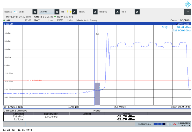
Figure 8.5-348: Conducted emission 1 MHz away from the lower band edge
