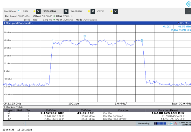
Figure 8.9-13: 99% Occupied bandwidth sample plot for NR 15 MHz channel
