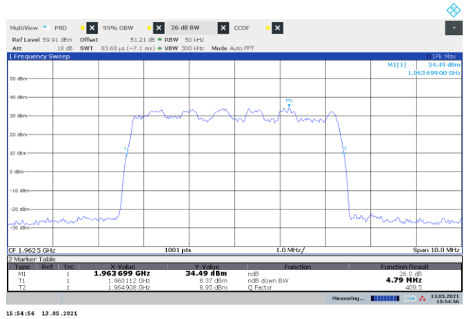
Figure 8.10-10: 26 dB bandwidth sample plot for NR 5 MHz channel
