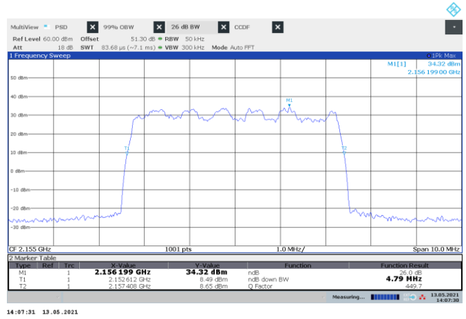
Figure 8.9-10: 26 dB bandwidth sample plot for NR 5 MHz channel
