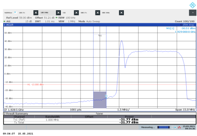
Figure 8.5-338: Conducted emission 1 MHz away from the lower band edge
