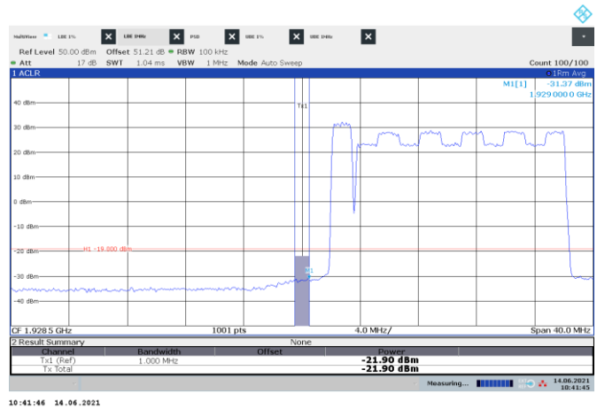
Figure 8.5-254: Conducted emission 1 MHz away from the lower band edge
