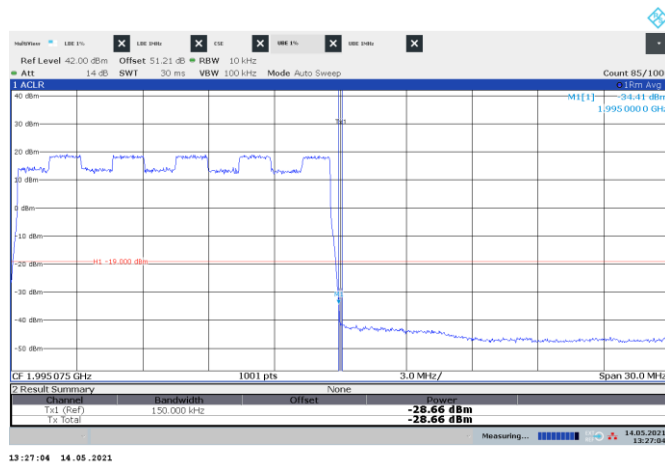
Figure 8.5-215: Conducted emission at the upper band edge
