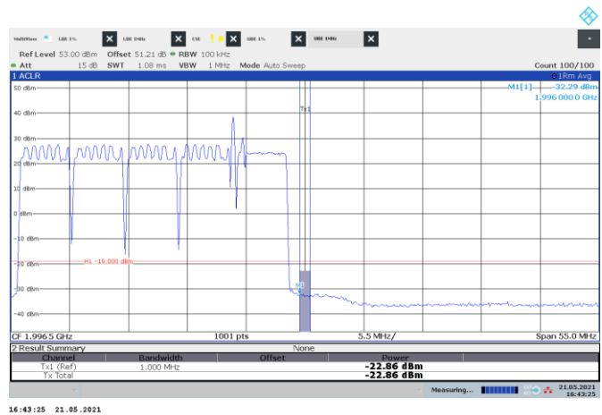
Figure 8.5-276: Conducted emission 1 MHz away from the upper band edge
