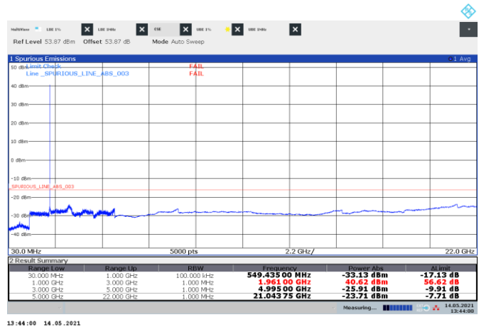
Figure 8.5-52: Conducted spurious emissions of CDMA mid channel, single carrier operation
