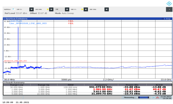
Figure 8.5-175: Conducted spurious emissions of NR 15 MHz + GSM contiguous mid channels, multi-RAT carrier operation
