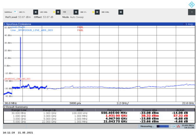
Figure 8.5-93: Conducted spurious emissions of GSM + LTE 5 MHz + 4xNR 5 MHz contiguous top channels, multi-RAT carrier operation
