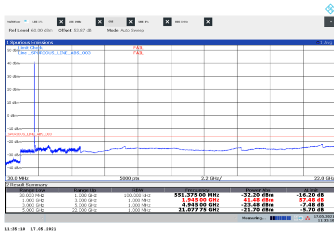
Figure 8.5-170: Conducted spurious emissions of NR 15 MHz + WCDMA contiguous bottom channels, multi-RAT carrier operation
