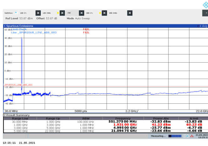
Figure 8.5-152: Conducted spurious emissions of LTE 15 MHz + GSM contiguous bottom channels, multi-RAT carrier operation
