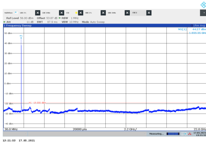
Figure 8.5-126: Conducted spurious emissions of LTE 5 MHz + GSM + 4x NR 5 MHz contiguous bottom channels, multi-RAT carrier operation
