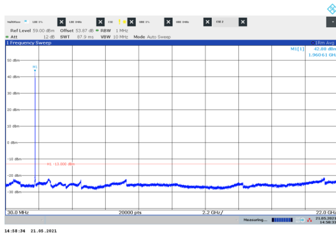
Figure 8.5-80: Conducted spurious emissions of GSM + LTE 5 MHz + NR 10 MHz contiguous mid channels, multi-RAT carrier operation
