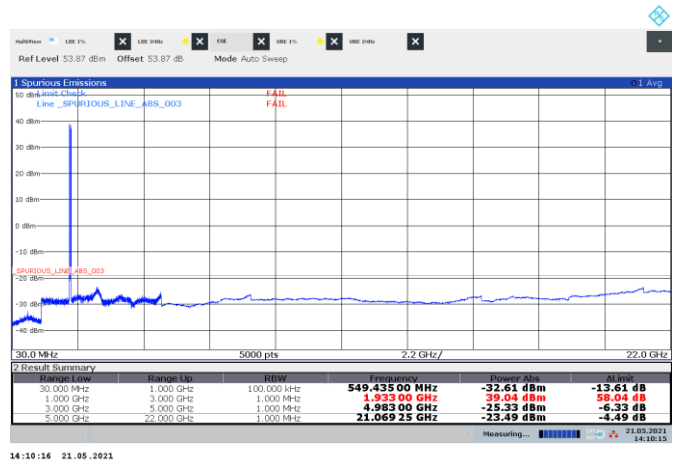
Figure 8.5-73: Conducted spurious emissions of CDMA and LTE 5 MHz and NR 15 MHz non-contiguous channels, multi-RAT carrier operation
