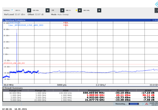
Figure 8.5-53: Conducted spurious emissions of CDMA top channel, single carrier operation
