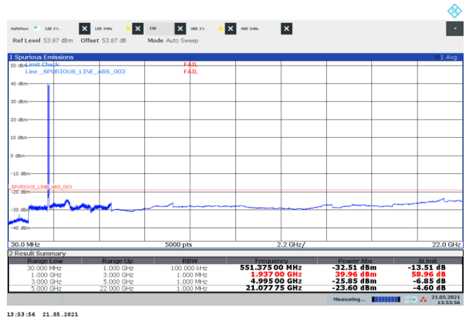
Figure 8.5-169: Conducted spurious emissions of NR 10 MHz and WCDMA + LTE 5 MHz non-contiguous channels, multi-RAT carrier operation
