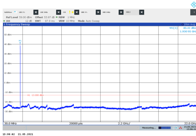
Figure 8.5-122: Conducted spurious emissions of GSM + 4× NR 5 MHz + LTE 5 MHz contiguous bottom channels, multi-RAT carrier operation
