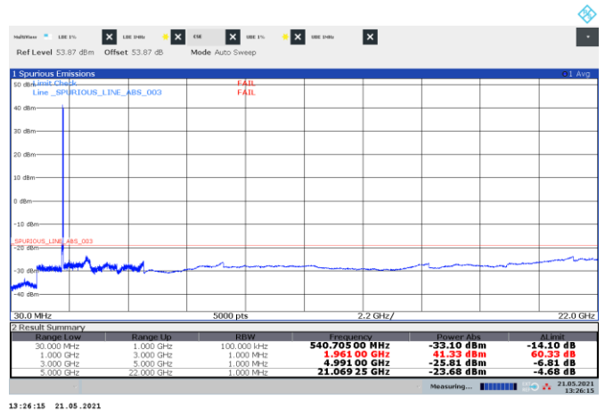
Figure 8.5-153: Conducted spurious emissions of LTE 15 MHz + GSM contiguous mid channels, multi-RAT carrier operation
