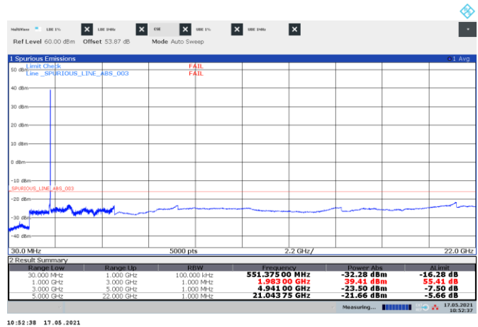
Figure 8.5-151: Conducted spurious emissions of LTE 15 MHz + WCDMA contiguous top channels, multi-RAT carrier operation
