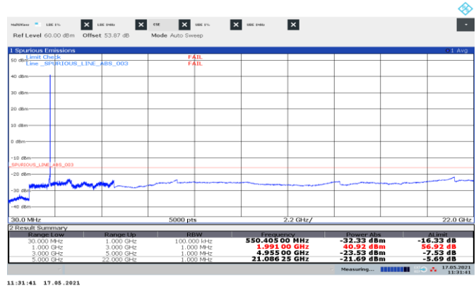
Figure 8.5-173: Conducted spurious emissions of NR 15 MHz + WCDMA contiguous top channels, multi-RAT carrier operation
