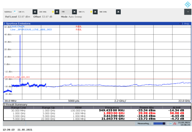
Figure 8.5-113: Conducted spurious emissions of WCDMA and LTE 15 MHz non-contiguous channels, multi-RAT carrier operation
