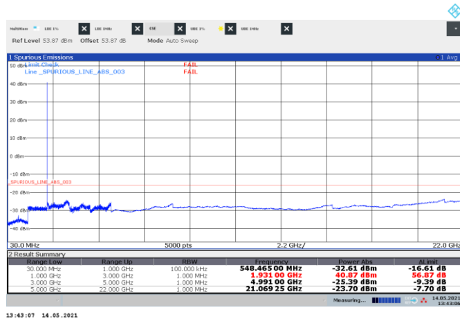
Figure 8.5-51: Conducted spurious emissions of CDMA low channel, single carrier operation
