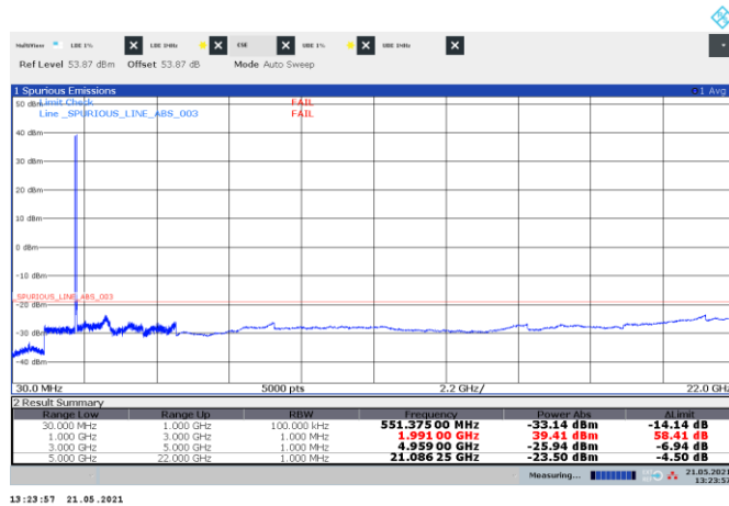
Figure 8.5-154: Conducted spurious emissions of LTE 15 MHz + GSM contiguous top channels, multi-RAT carrier operation
