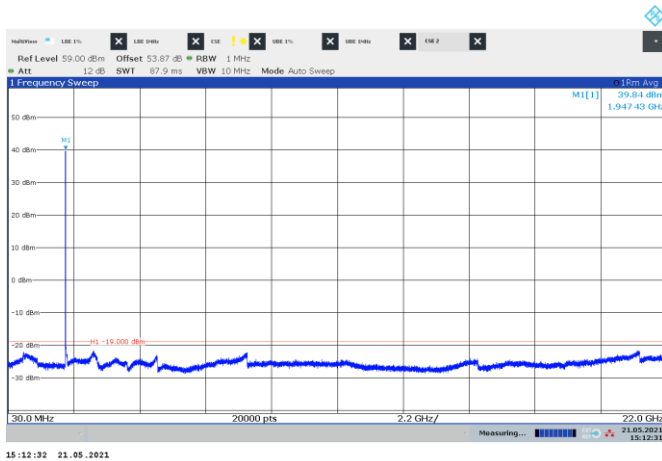
Figure 8.5-102: Conducted spurious emissions of WCDMA + LTE 10 MHz + NR 5 MHz contiguous bottom channels, multi-RAT carrier operation
