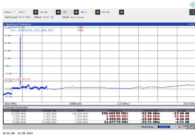
Figure 8.5-138: Conducted spurious emissions of LTE 10 MHz and CDMA + NR 5 MHz non-contiguous channels, multi-RAT carrier operation
