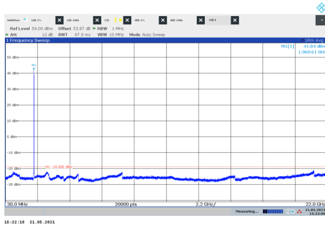
Figure 8.5-72: Conducted spurious emissions of CDMA + NR 10 MHz + LTE 5 MHz contiguous mid channels, multi-RAT carrier operation
