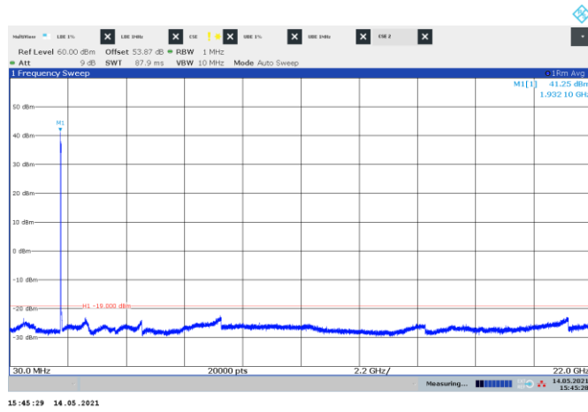
Figure 8.5-60: Conducted spurious emissions of CDMA + 4xNR 5 MHz + LTE 5 MHz contiguous bottom channels, multi-RAT carrier operation
