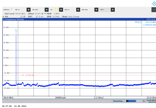
Figure 8.5-134: Conducted spurious emissions of LTE 10 MHz + GSM + NR 5 MHz contiguous bottom channels, multi-RAT carrier operation
