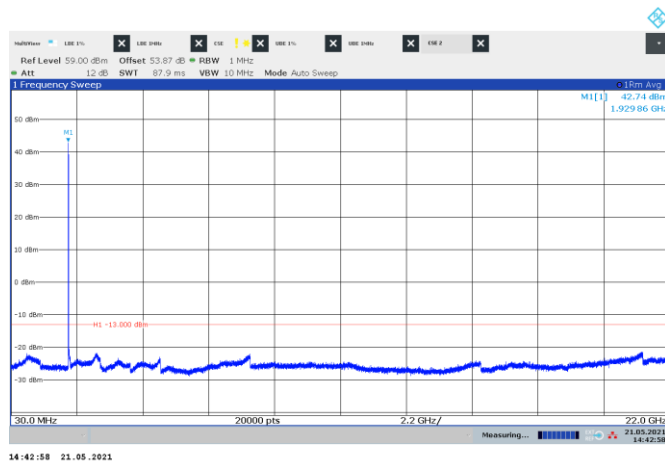
Figure 8.5-82: Conducted spurious emissions of GSM + LTE 10 MHz + NR 5 MHz contiguous mid channels, multi-RAT carrier operation
