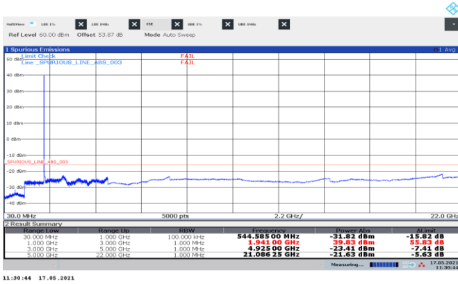
Figure 8.5-172: Conducted spurious emissions of NR 15 MHz + WCDMA contiguous bottom channels, multi-RAT carrier operation
