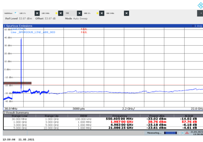
Figure 8.5-140: Conducted spurious emissions of LTE 10 MHz and WCDMA + NR 5 MHz non-contiguous channels, multi-RAT carrier operation
