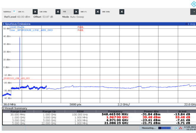
Figure 8.5-156: Conducted spurious emissions of NR 15 MHz + LTE 5 MHz contiguous mid channels, multi-RAT carrier operation
