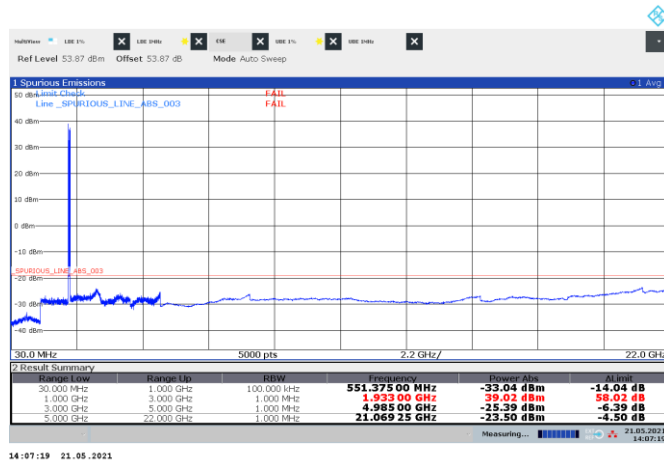
Figure 8.5-76: Conducted spurious emissions of CDMA + LTE 15 MHz and NR 5 MHz and NR 10 MHz + LTE 5 MHz + NR 5 MHz, multi-RAT carrier operation
