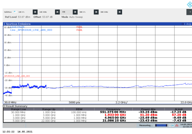
Figure 8.5-54: Conducted spurious emissions of WCDMA low channel, single carrier operation
