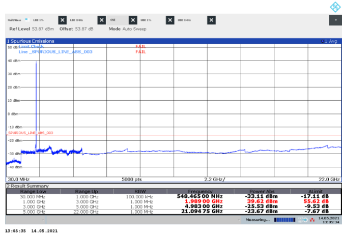
Figure 8.5-31: Conducted spurious emissions of NR 10 MHz top channel, single carrier operation
