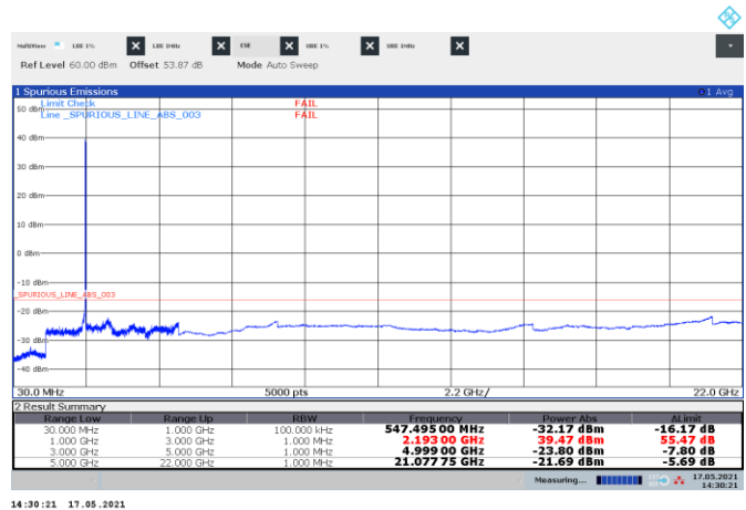
Figure 8.3-39: Conducted spurious emissions of NR 20 MHz top channel, single-carrier operation
