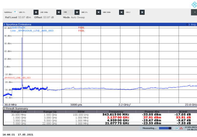
Figure 8.3-25: Conducted spurious emissions of LTE 10 MHz three contiguous bottom channels, three-carrier operation
