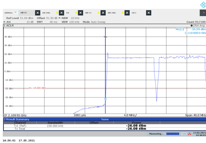
Figure 8.3-105: Conducted emission at the lower band edge
