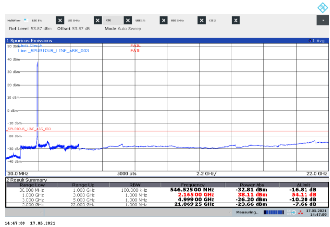
Figure 8.3-26: Conducted spurious emissions of LTE 10 MHz three contiguous mid channels, three-carrier operation
