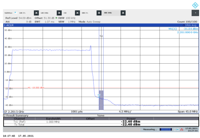
Figure 8.3-104: Conducted emission 1 MHz away from the upper band edge
