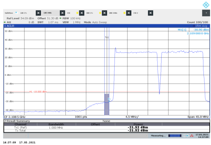
Figure 8.3-106: Conducted emission 1 MHz away from the lower band edge
