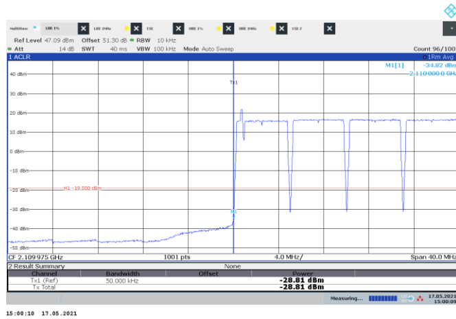
Figure 8.3-113: Conducted emission at the lower band edge
