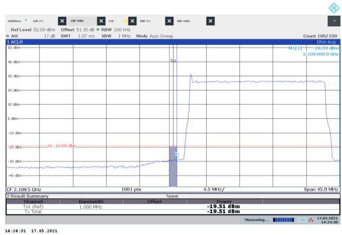
Figure 8.3-102: Conducted emission 1 MHz away from the lower band edge
