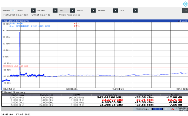
Figure 8.3-50: Conducted spurious emissions of NR 10 MHz three contiguous bottom channels, three-carrier operation
