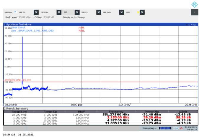
Figure 8.3-62: Conducted spurious emissions of multi-RAT operation, LTE 10 MHz and NR 5 MHz and WCDMA (top)
