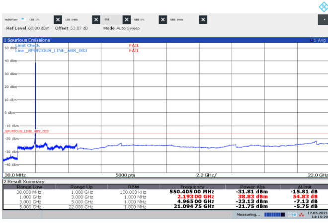
Figure 8.3-9: Conducted spurious emissions of LTE 15 MHz top channel, single carrier operation
