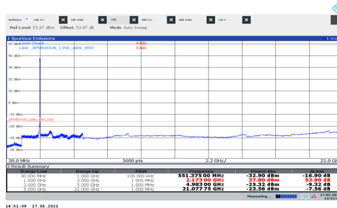
Figure 8.3-52: Conducted spurious emissions of NR 10 MHz three contiguous top channels, three-carrier operation
