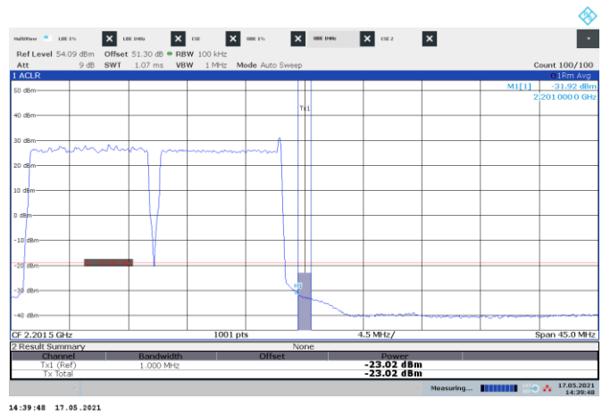
Figure 8.3-108: Conducted emission 1 MHz away from the upper band edge
