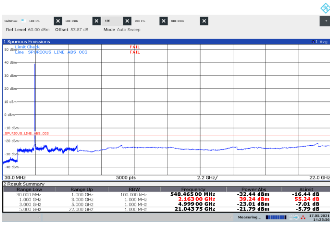
Figure 8.3-11: Conducted spurious emissions of LTE 20 MHz mid channel, single carrier operation
