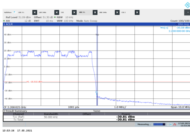
Figure 8.3-119: Conducted emission at the upper band edge
