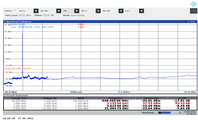
Figure 8.3-51: Conducted spurious emissions of NR 10 MHz three contiguous mid channels, three-carrier operation
