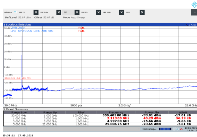
Figure 8.3-87: Conducted spurious emissions of multi-RAT operation, WCDMA and NR 15 MHz (contiguous)
