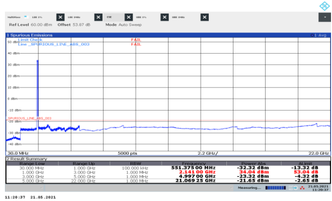
Figure 8.3-49: Conducted spurious emissions of NR 20 MHz two non-contiguous channels, two-carrier operation
