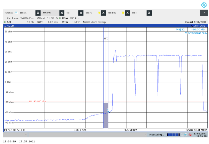
Figure 8.3-114: Conducted emission 1 MHz away from the lower band edge
