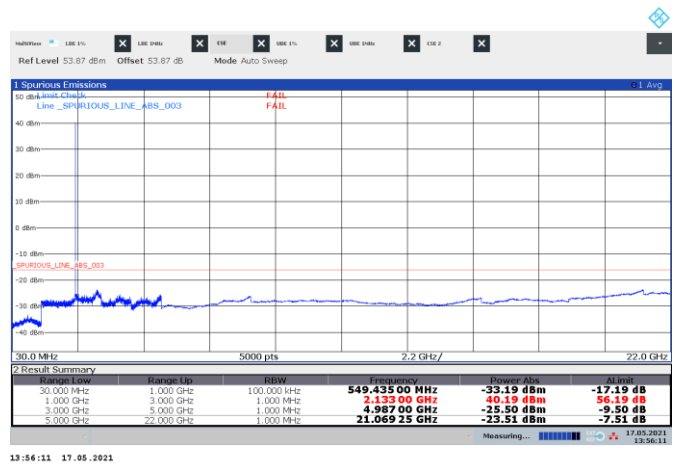
Figure 8.3-54: Conducted spurious emissions of WCDMA mid channel, single-carrier operation
