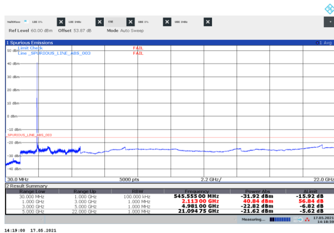
Figure 8.3-34: Conducted spurious emissions of NR 15 MHz low channel, single-carrier operation
