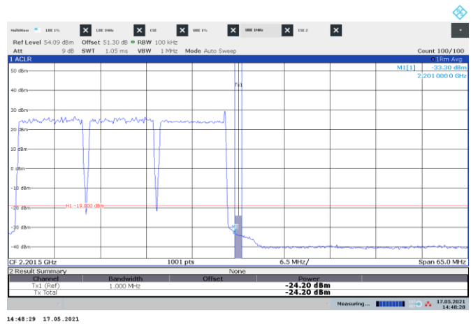
Figure 8.3-112: Conducted emission 1 MHz away from the upper band edge
