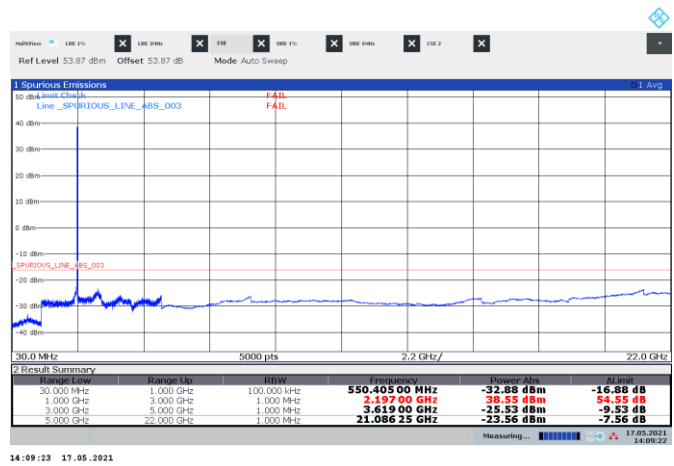
Figure 8.3-33: Conducted spurious emissions of NR 10 MHz top channel, single-carrier operation
