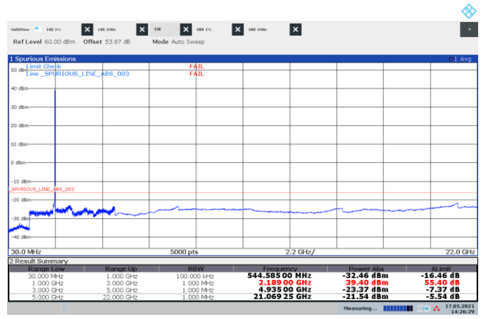
Figure 8.3-12: Conducted spurious emissions of LTE 20 MHz top channel, single carrier operation
