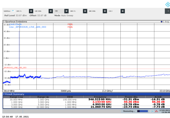
Figure 8.3-55: Conducted spurious emissions of WCDMA top channel, single-carrier operation
