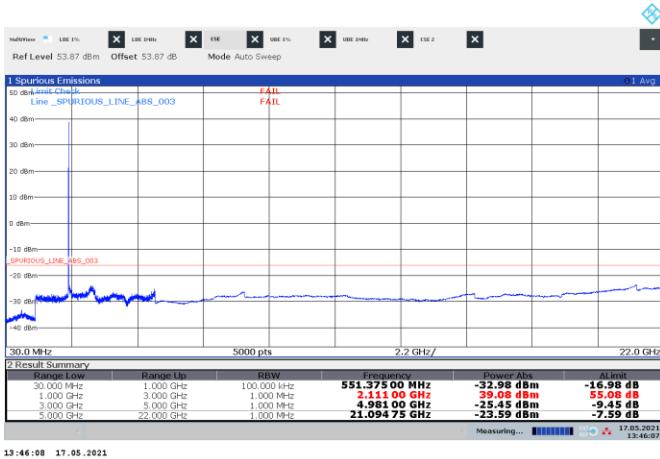
Figure 8.3-1: Conducted spurious emissions of LTE 5 MHz low channel, single carrier operation
