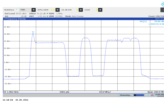
Figure 8.2-53: PSD of multi-RAT operation, GSM + LTE 20 MHz and NR 5 MHz and NR 10 MHz + LTE 5 MHz + NR 5 MHz
