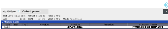
Figure 8.2-5: Output channel power of LTE 15 MHz channel bandwidth, single carrier operation, sample plot
