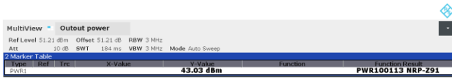
Figure 8.2-1: Output channel power of LTE 5 MHz channel bandwidth, single carrier operation, sample plot
