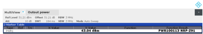
Figure 8.2-2: Output channel power of NR 5 MHz channel bandwidth, single carrier operation, sample plot
