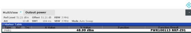
Figure 8.2-7: Output channel power of LTE 20 MHz channel bandwidth, single carrier operation, sample plot
