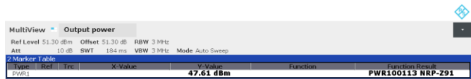
Figure 8.1-6: Output channel power of NR 15 MHz channel bandwidth, single carrier operation, sample plot
