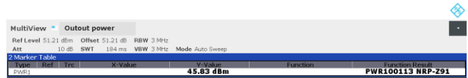
Figure 8.2-4: Output channel power of NR 10 MHz channel bandwidth, single carrier operation, sample plot
