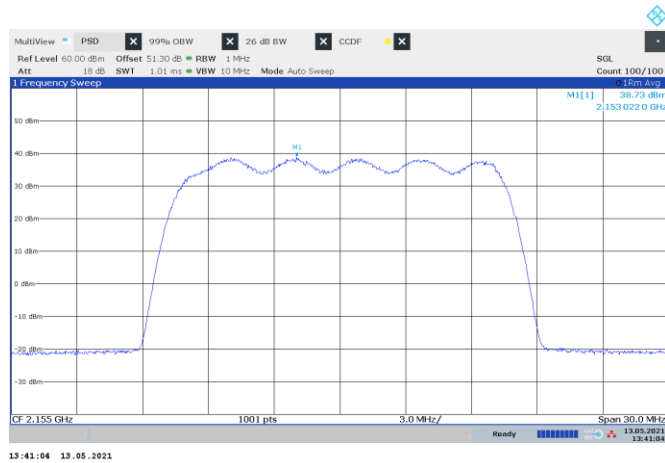
Figure 8.1-25: PSD of NR 15 MHz channel bandwidth, single carrier operation, sample plot
