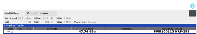
Figure 8.2-6: Output channel power of NR 15 MHz channel bandwidth, single carrier operation, sample plot
