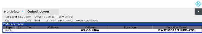
Figure 8.1-4: Output channel power of NR 10 MHz channel bandwidth, single carrier operation, sample plot
