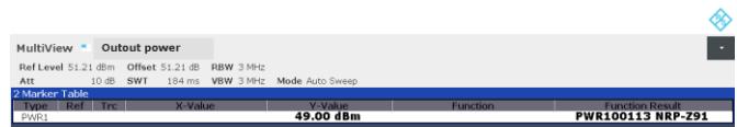
Figure 8.2-8: Output channel power of NR 20 MHz channel bandwidth, single carrier operation, sample plot
