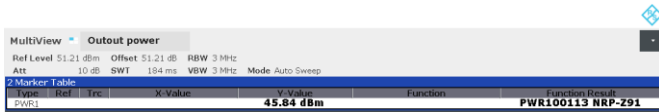
Figure 8.2-3: Output channel power of LTE 10 MHz channel bandwidth, single carrier operation, sample plot
