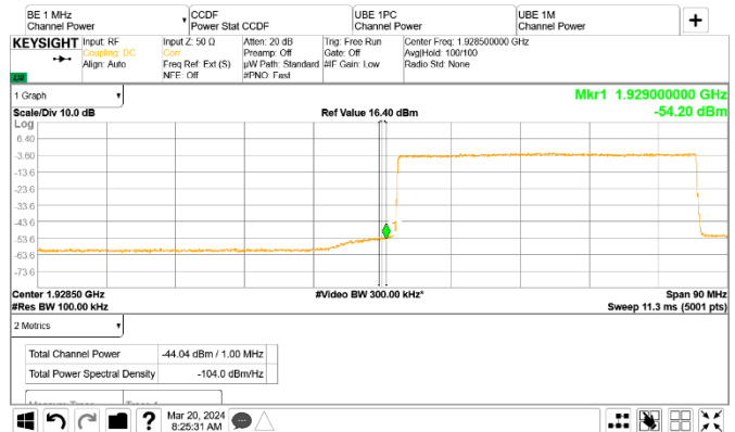
Figure 8.2-29: Conducted emission 1 MHz away from the lower band edge
