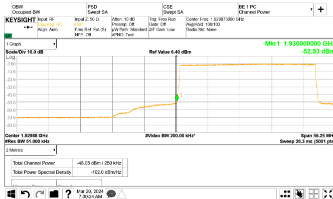
Figure 8.2-16: Conducted emission at the lower band edge
