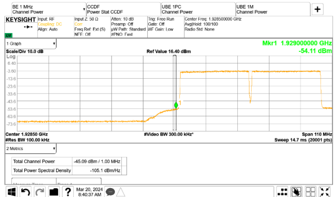
Figure 8.2-33: Conducted emission 1 MHz away from the lower band edge
