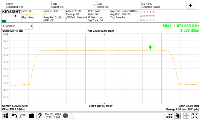
Figure 8.1-1: PSD of NR 25 MHz channel bandwidth, single carrier operation, sample plot
