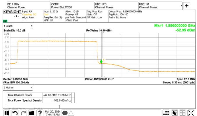
Figure 8.2-23: Conducted emission 1 MHz away from the upper band edge
