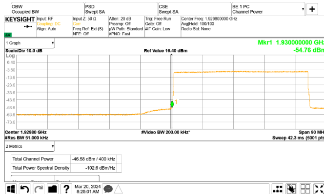
Figure 8.2-28: Conducted emission at the lower band edge
