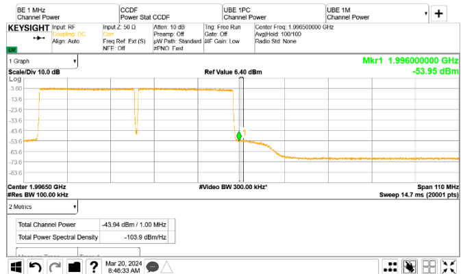
Figure 8.2-35: Conducted emission 1 MHz away from the upper band edge
