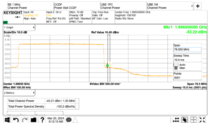
Figure 8.2-27: Conducted emission 1 MHz away from the upper band edge
