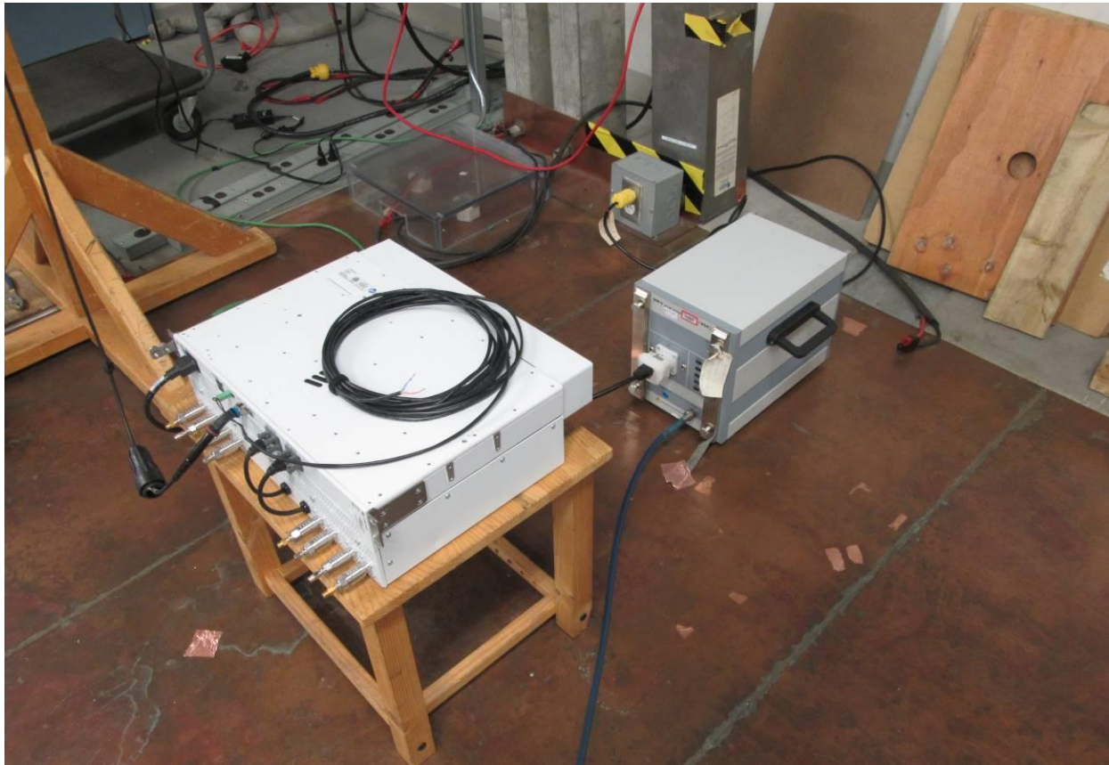
Figure 47: Setup for CE tests on AC power cables
