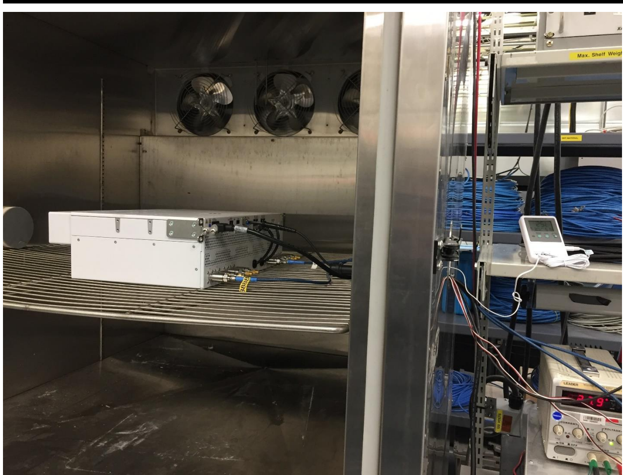
Figure 4: EUT test fixture in a thermal test chamber
