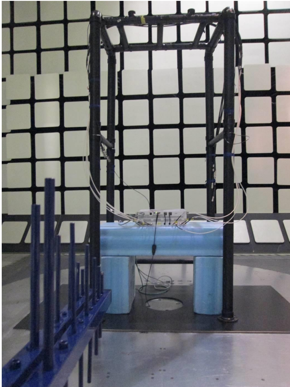
Figure 44: Setup for RE tests at 30 MHz to 1 GHz with NR (Single & Multi Carrier)
