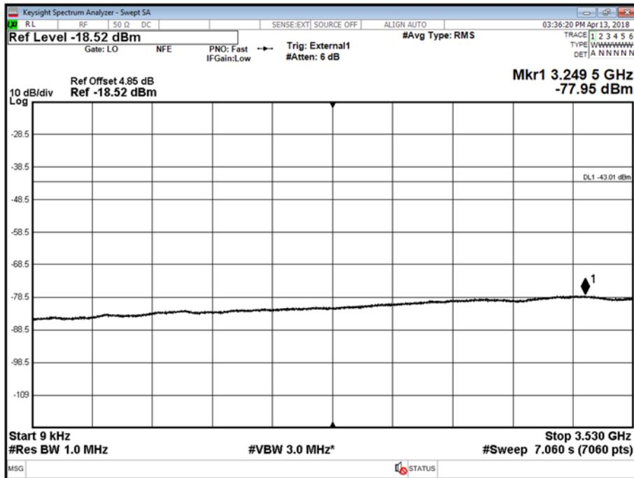
Antenna A - LTE Modulation 64QAM - LTE Carrier Bandwidth 20.0 MHz - Channel Position T - Band mask\_low - Range Low
