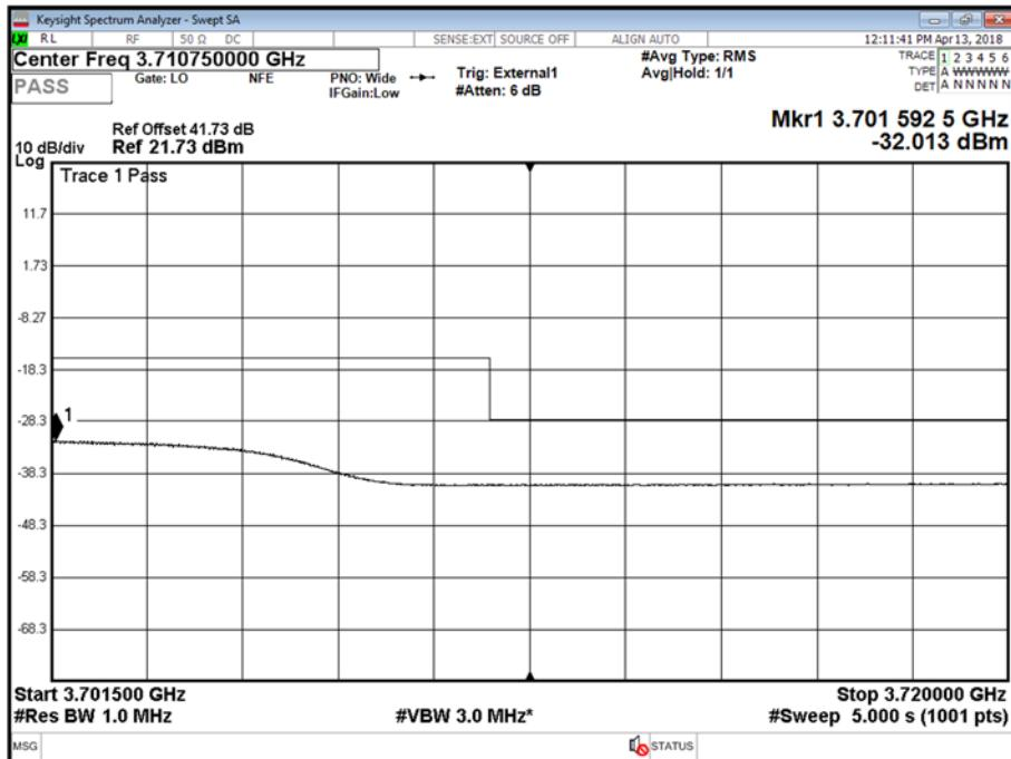
Antenna B - LTE Modulation 64QAM - LTE Carrier Bandwidth 20.0 MHz - Channel Position T - Band 2 - Range 3720 to 5000 MHz
