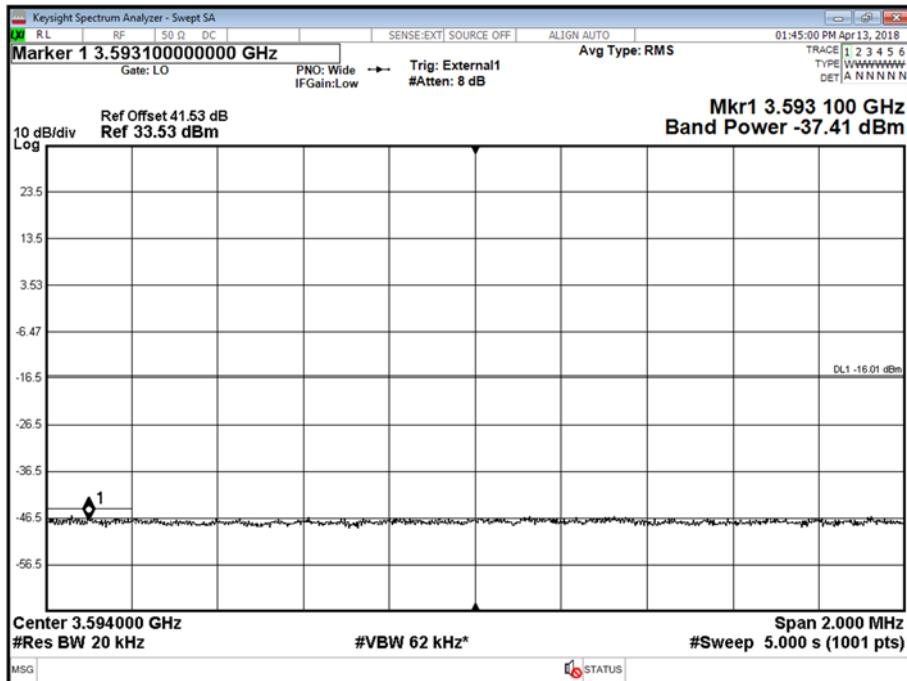
Antenna B - LTE Modulation 64QAM - LTE Carrier Bandwidth 20.0 MHz - Channel Position M - Band edge - Range high edge high
