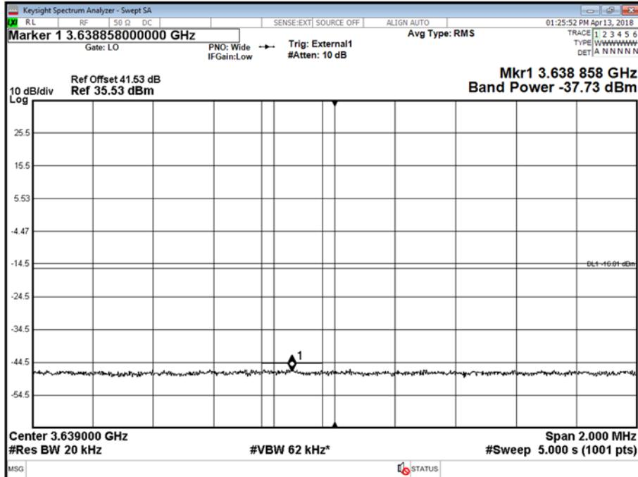
Antenna B - LTE Modulation 64QAM - LTE Carrier Bandwidth 20.0 MHz - Channel Position T - Band edge - Range high edge high
