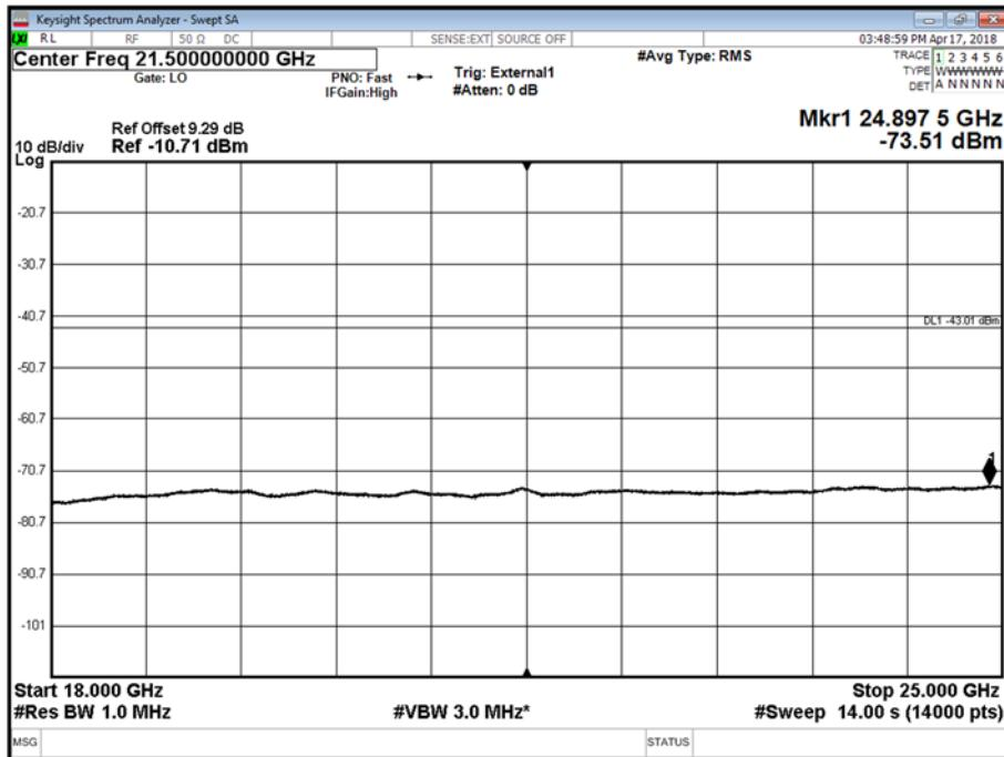
Antenna B - LTE Modulation 64QAM - LTE Carrier Bandwidth 20.0 MHz - Channel Position T - Band 6 - Range 25000 to 37000 MHz
