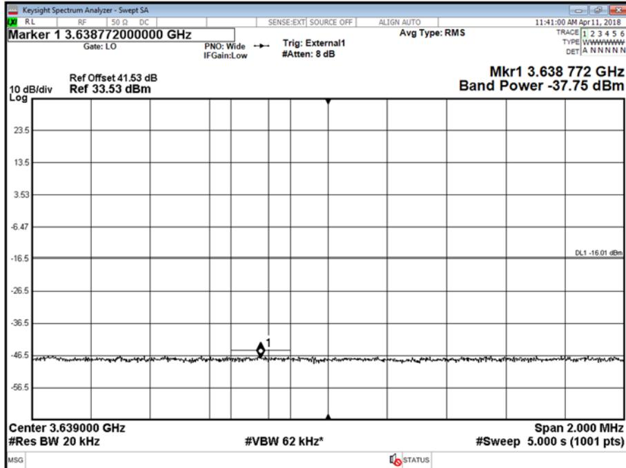
Antenna A - LTE Modulation 64QAM - LTE Carrier Bandwidth 20.0 MHz - Channel Position T - Band edge - Range high edge high
