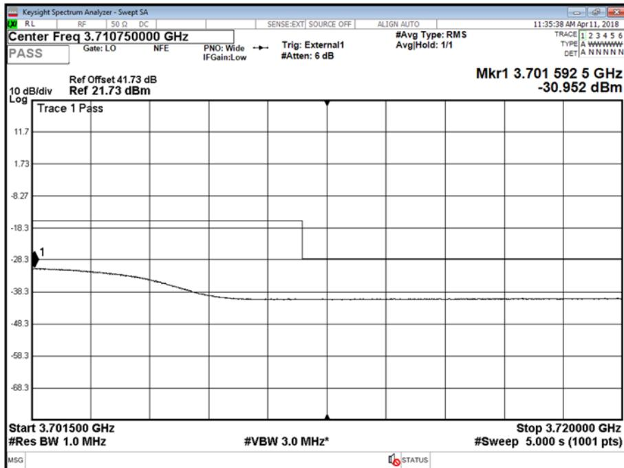
Antenna A - LTE Modulation 64QAM - LTE Carrier Bandwidth 20.0 MHz - Channel Position T - Band 2 - Range 3720 to 5000 MHz
