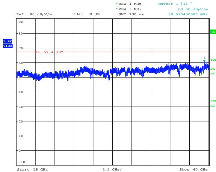
Antenna A - LTE Modulation - LTE Carrier Bandwidth 20MHz - Channel Position M - Band 6 - Range In Band
