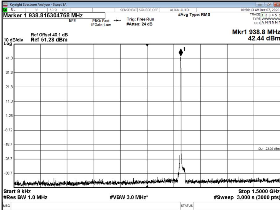
Antenna B - LTE + NB-IoT IB Modulation QPSK - LTE + NB-IoT IB Carrier Bandwidth 3.0 MHz + NB-IoT IB - Channel Position M - Band 2 - Range 1500 to 10000 MHz
