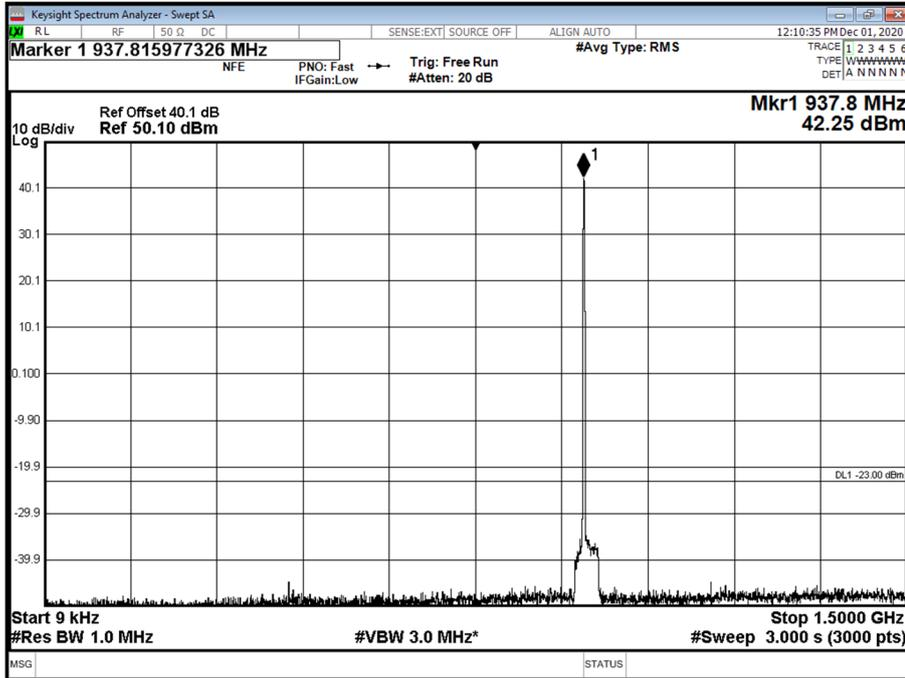
Antenna B - LTE-Modulation 16QAM - LTE Carrier Bandwidth 1.4 MHz - Channel Position M - Band 2 - Range 1500 to 10000 MHz
