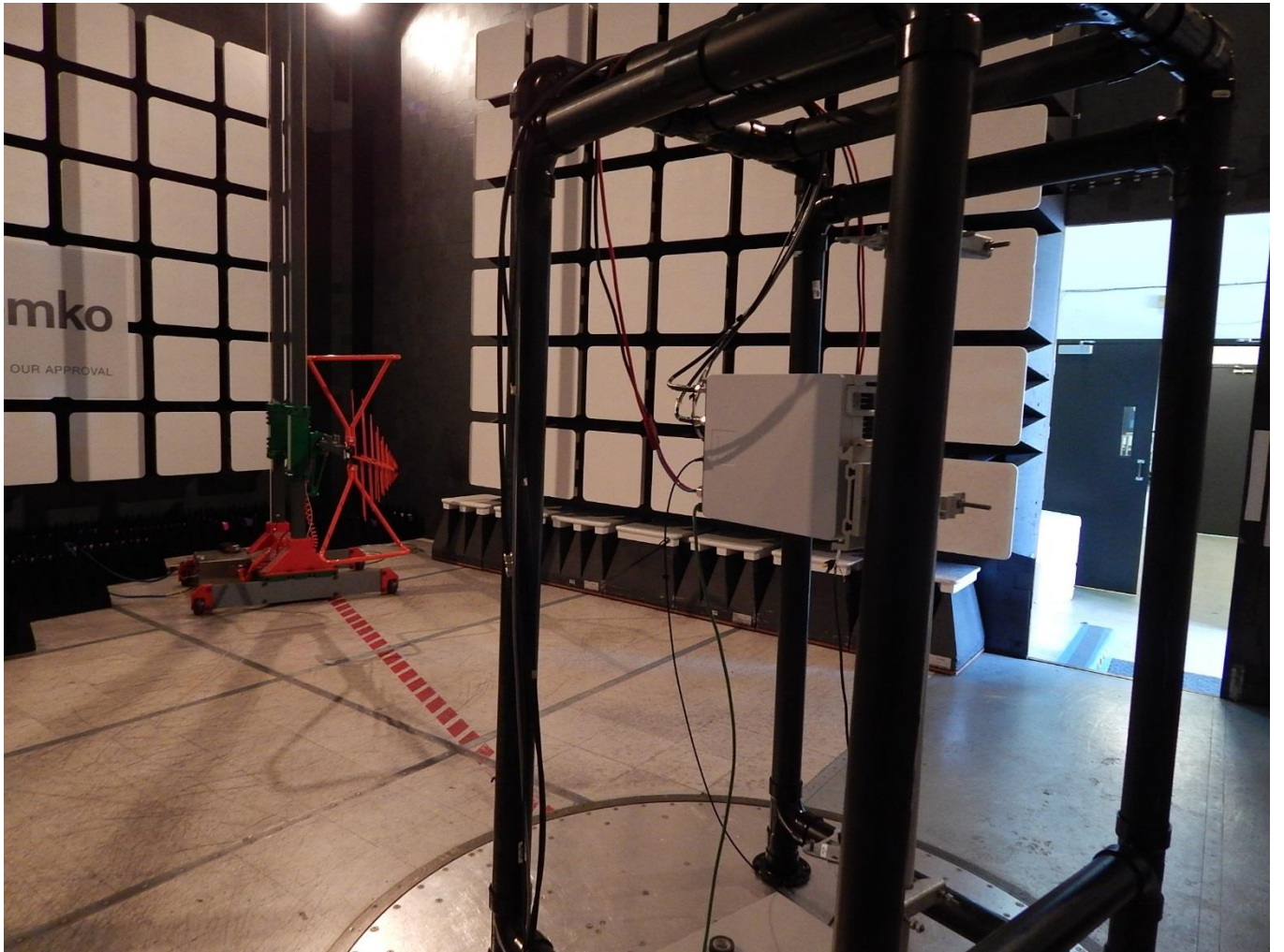
EUT Set-up for Radiated Compliance Testing
