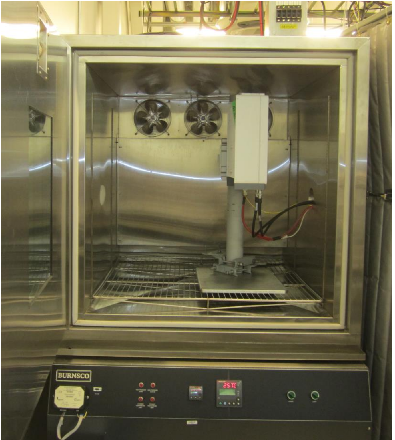
EUT Set-up for Radio Compliance Testing
