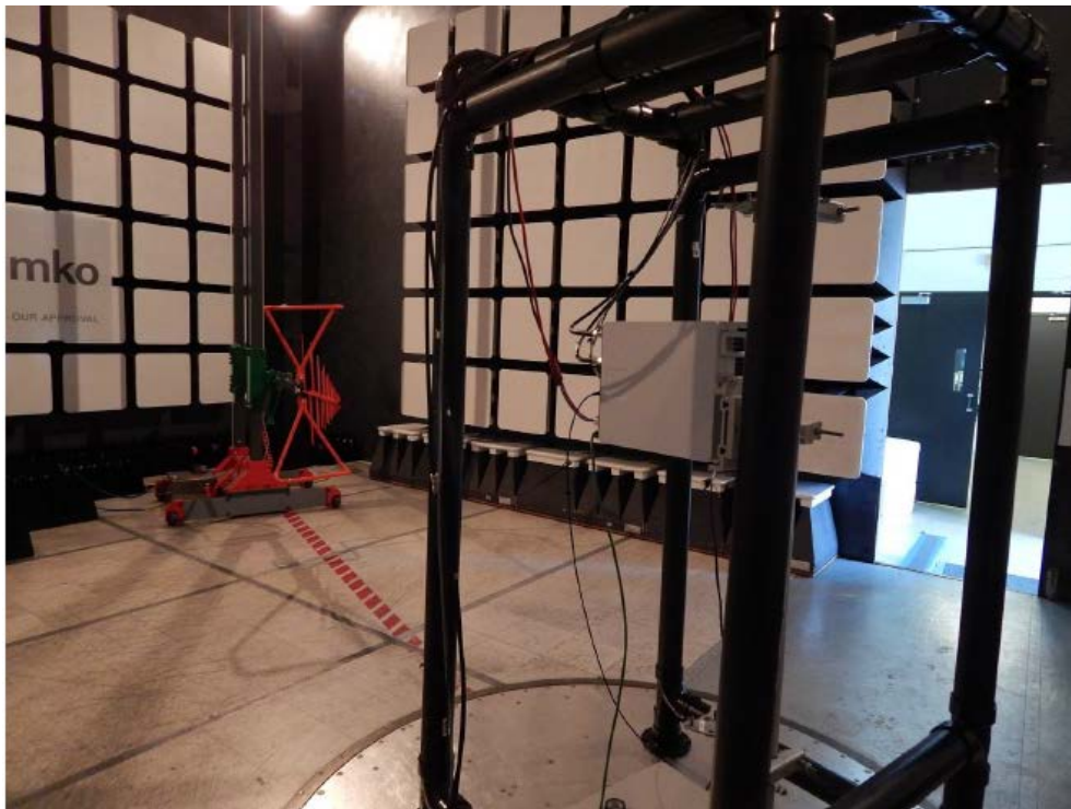
Figure 8.3-2: EUT Set-up for Radiated Compliance Testing
