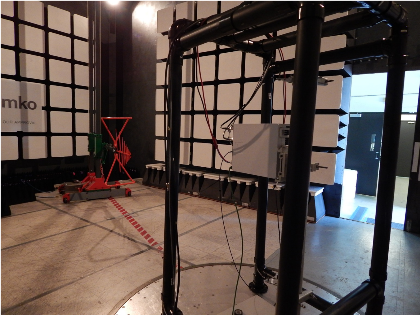
Figure 3.6-3: EUT Set-up for Radiated Compliance Testing
