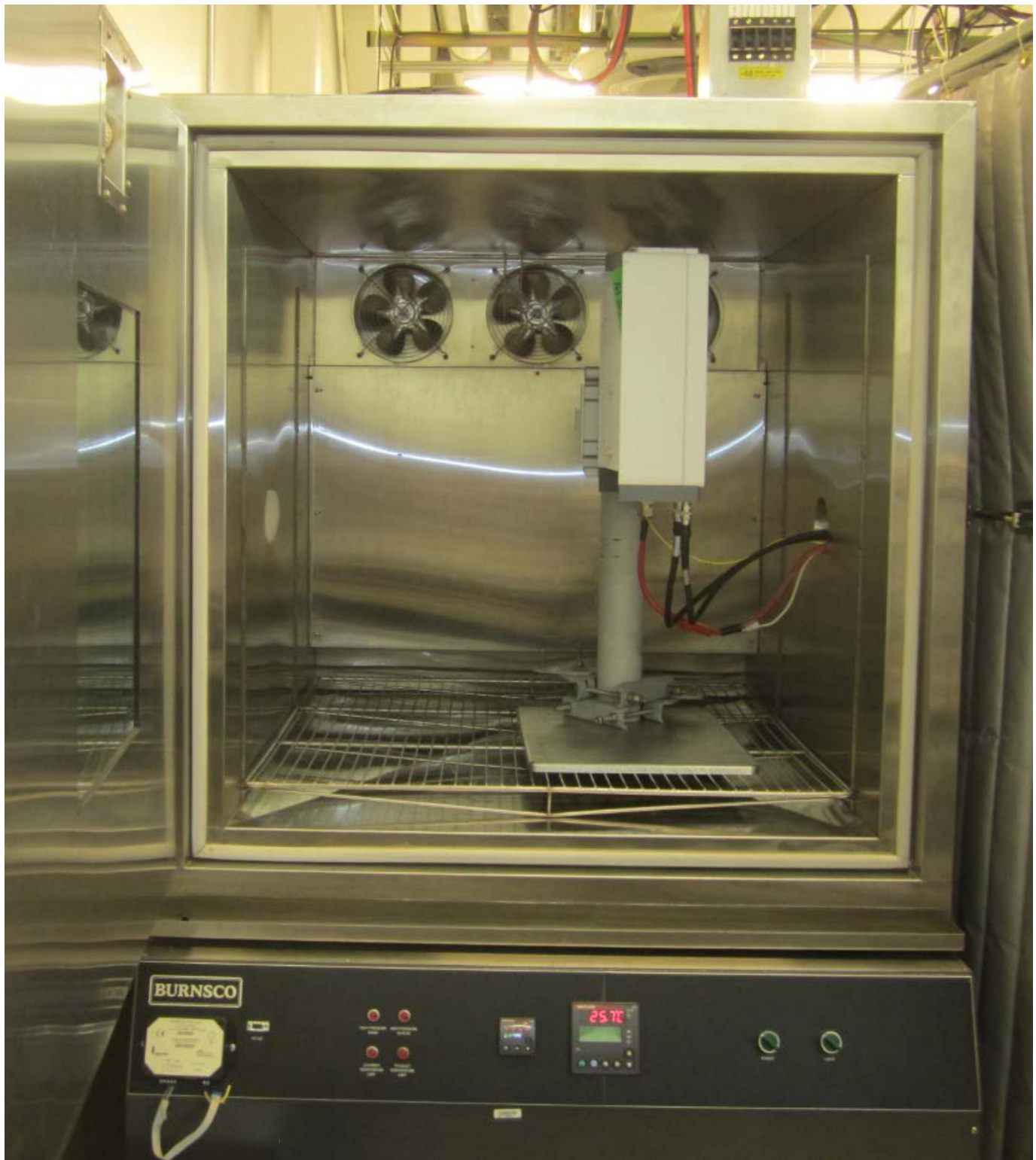
Figure 3.6-2: EUT Set-up for Radio Compliance Testing
