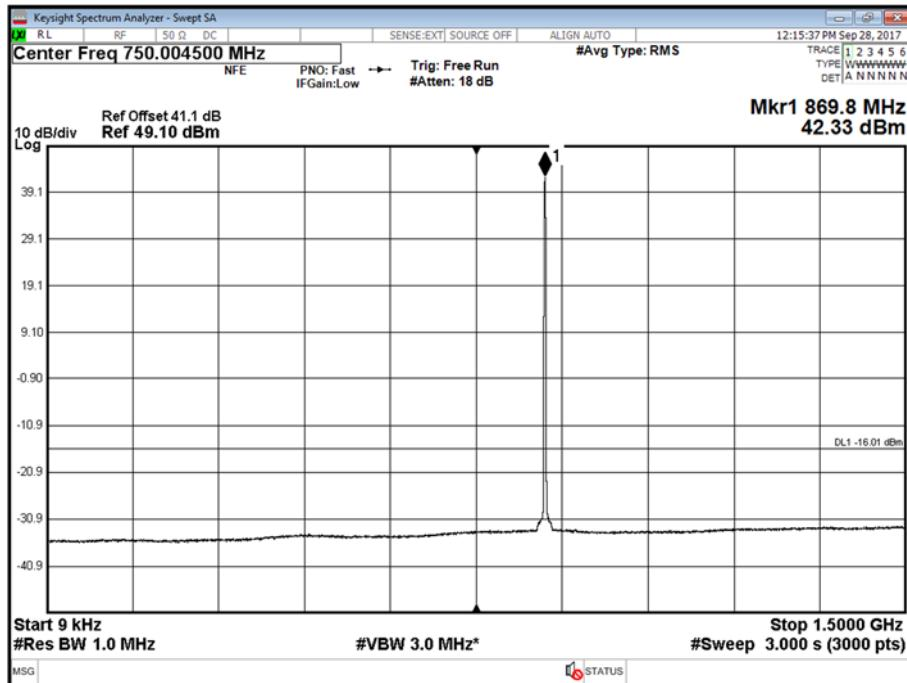
Antenna A - LTE Modulation QPSK - LTE Carrier Bandwidth 1.4 MHz - Channel Position B - Band 2 - Range 1500 to 9000 MHz
