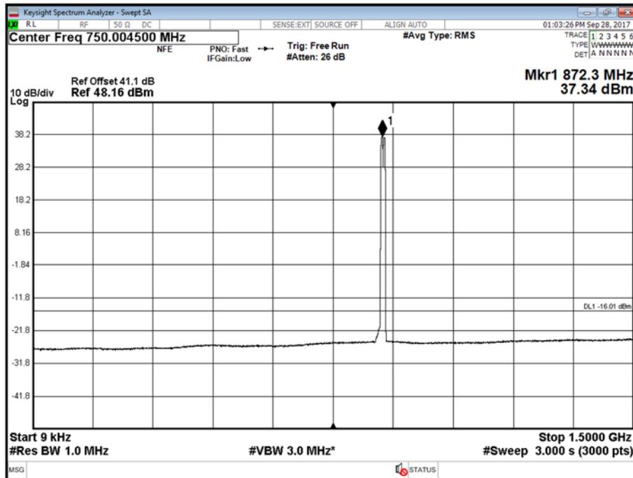
Antenna A - LTE Modulation QPSK - LTE Carrier Bandwidth 5 MHz - Channel Position M - Band 2 - Range 1500 to 9000 MHz
