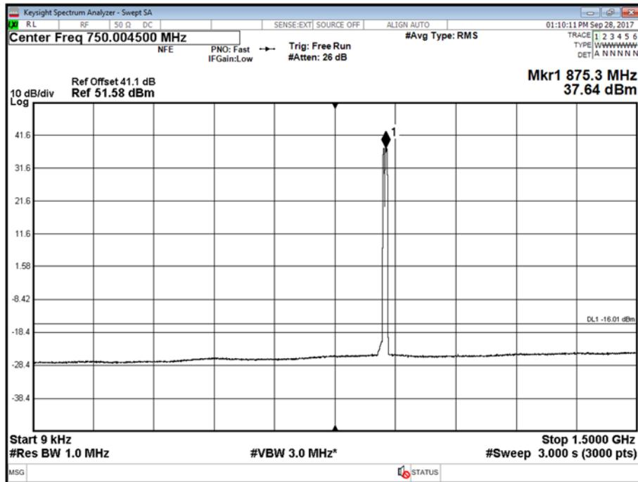
Antenna A - LTE Modulation QPSK - LTE Carrier Bandwidth 3.0 MHz - Channel Position M - Band 2 - Range 1500 to 9000 MHz
