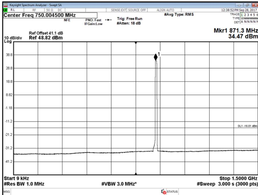
Antenna A - LTE Modulation QPSK - LTE Carrier Bandwidth 10.0 MHz - Channel Position M - Band 2 - Range 1500 to 9000 MHz
