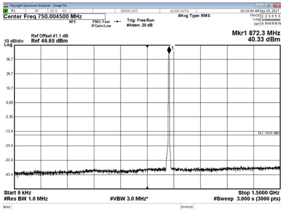
Antenna B - LTE Modulation QPSK - LTE Carrier Bandwidth 5.0 MHz - Channel Position B - Band 2 - Range 1500 to 9000 MHz
