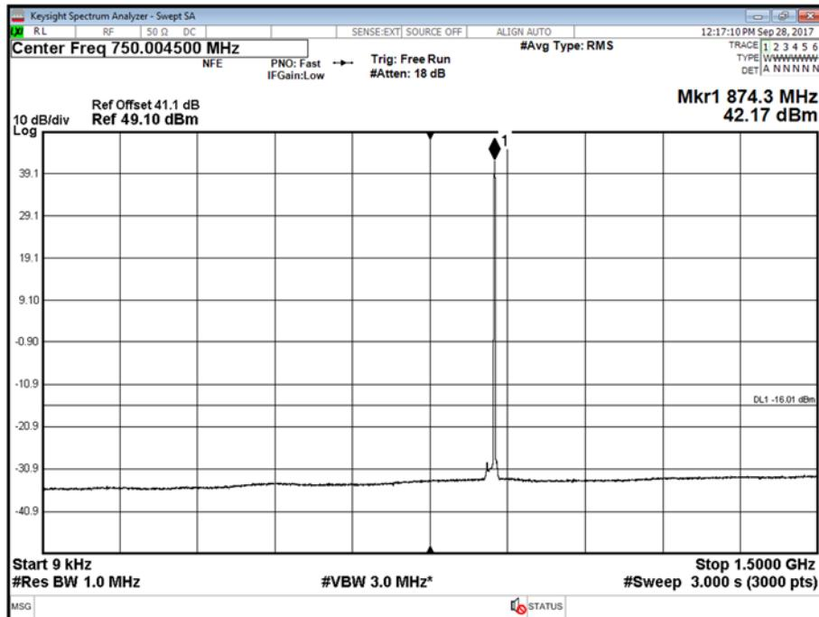
Antenna A - LTE Modulation QPSK - LTE Carrier Bandwidth 1.4 MHz - Channel Position M - Band 2 - Range 1500 to 9000 MHz
