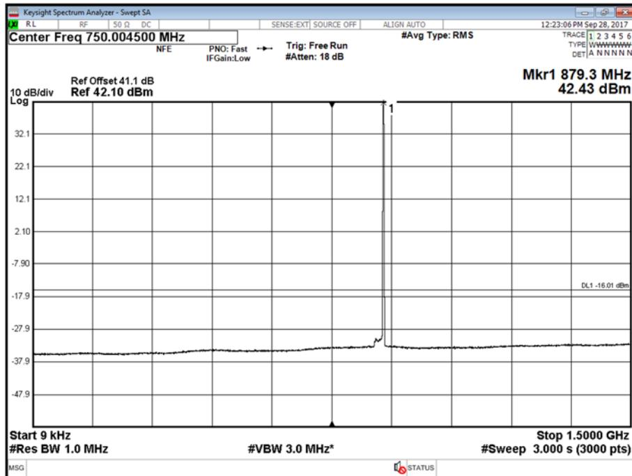
Antenna A - LTE Modulation QPSK - LTE Carrier Bandwidth 1.4 MHz - Channel Position T - Band 2 - Range 1500 to 9000 MHz
