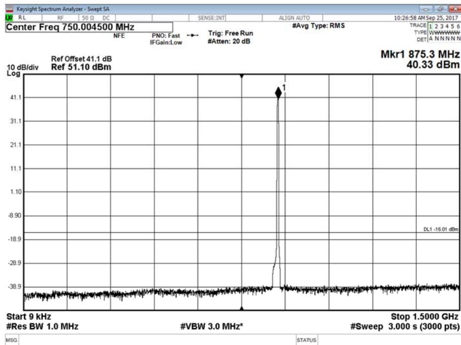
Antenna B - LTE Modulation QPSK - LTE Carrier Bandwidth 5.0 MHz - Channel Position M - Band 2 - Range 1500 to 9000 MHz
