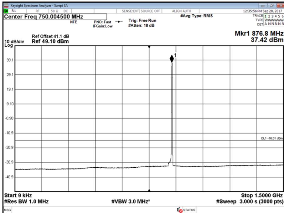
Antenna A - LTE Modulation QPSK - LTE Carrier Bandwidth 5.0 MHz - Channel Position T - Band 2 - Range 1500 to 9000 MHz
