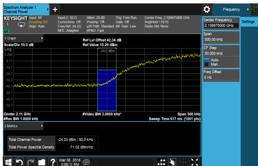
The channel power of 50kHz for 2109.975MHz is -24.03dBm, which is within the limit of -19.02.00dBm.
