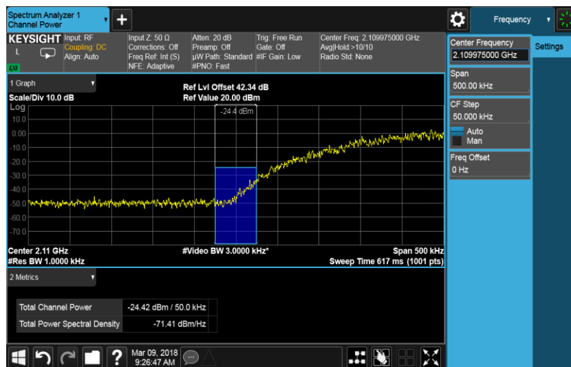
The channel power of 50kHz for 2109.975MHz is -24.42dBm, which is within the limit of -19.02dBm.
