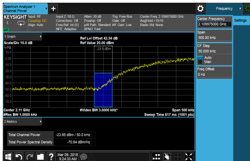
The channel power of 50kHz for 2109.975MHz is -23.85dBm, which is within the limit of -19.02dBm.
