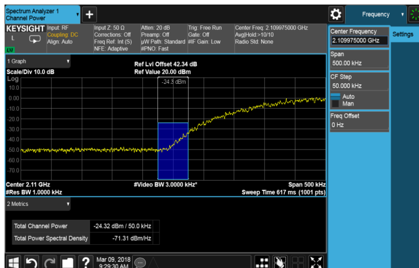
The channel power of 50kHz for 2109.975MHz is -24.32dBm, which is within the limit of -19.02dBm.
