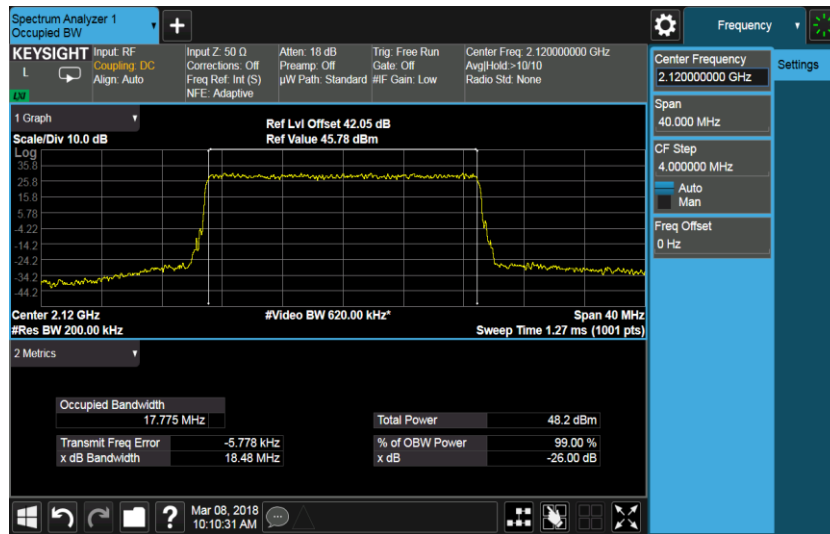
Port C, QPSK 20.0M Channel position B
