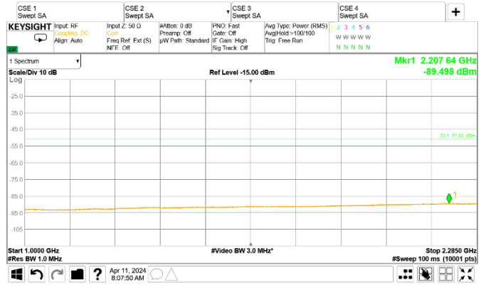
Figure 8.2-74: Conducted spurious emissions of NR 5 MHz mid channel, single carrier operation [1 GHz to 2.285 GHz]
