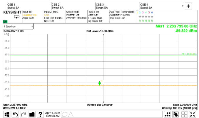
Figure 8.2-112: Conducted spurious emissions of NR 5 MHz, Contiguous Channels, two carrier operation [2.2875 GHz to 2.30 GHz]
