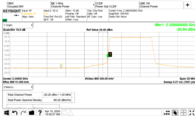
Figure 8.2-149: Conducted emission from the lower band edge
