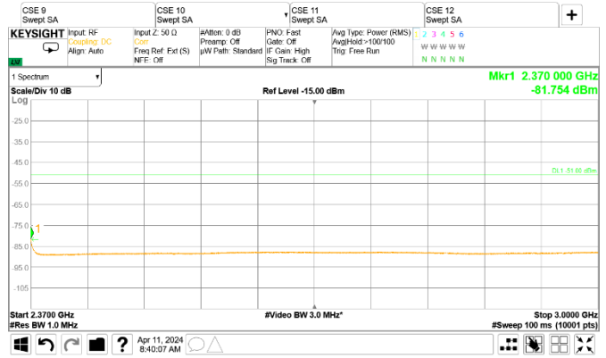
Figure 8.2-142: Conducted spurious emissions of Multi RAT operation, LTE 5 MHz + NR 5 MHz [2.70 GHz to 3 GHz]
