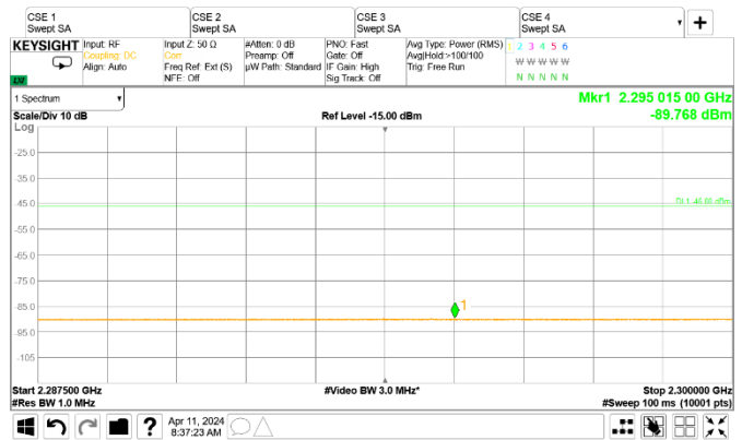
Figure 8.2-136: Conducted spurious emissions of Multi RAT operation, LTE 5 MHz + NR 5 MHz [2.2875 GHz to 2.30 GHz]
