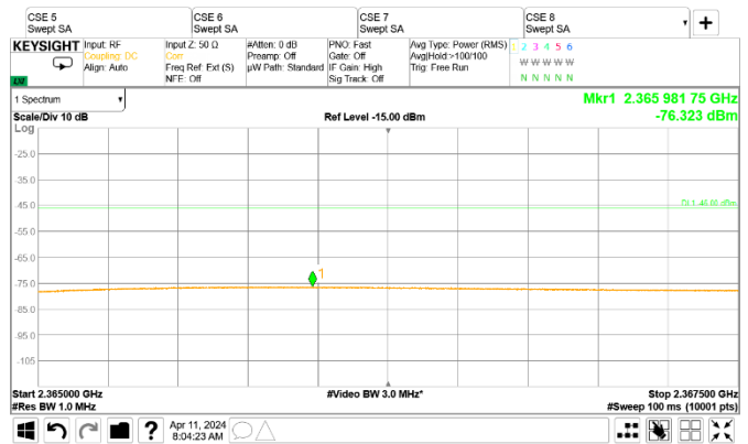
Figure 8.2-68: Conducted spurious emissions of NR 5 MHz low channel, single carrier operation [2.365 GHz to 2.3675 GHz]
