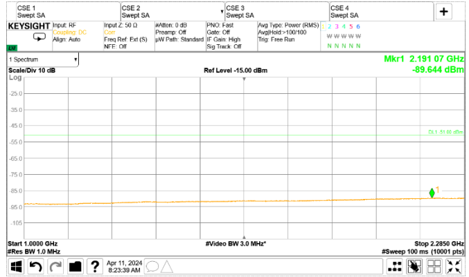
Figure 8.2-110: Conducted spurious emissions of NR 5 MHz, Contiguous Channels, two carrier operation [1 GHz to 2.285 GHz]
