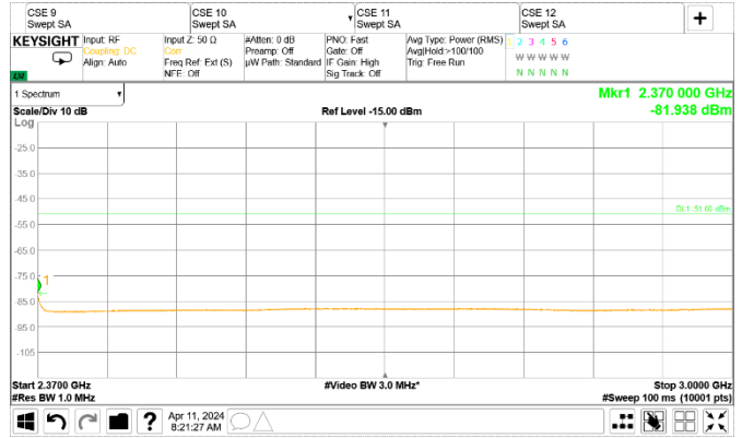
Figure 8.2-106: Conducted spurious emissions of NR 10 MHz, single carrier operation [2.70 GHz to 3 GHz]
