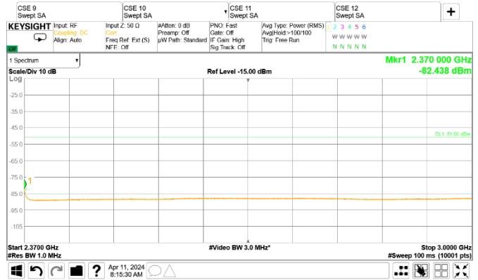
Figure 8.2-94: Conducted spurious emissions of NR 5 MHz top channel, single carrier operation [2.70 GHz to 3 GHz]
