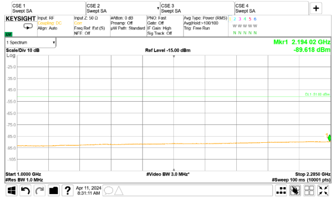
Figure 8.2-122: Conducted spurious emissions of Multi RAT operation, NR 5 MHz + LTE 5 MHz [1 GHz to 2.285 GHz]
