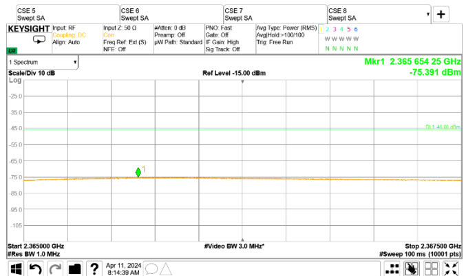
Figure 8.2-92: Conducted spurious emissions of NR 5 MHz top channel, single carrier operation [2.365 GHz to 2.3675 GHz]
