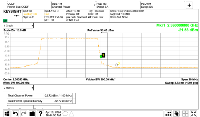
Figure 8.2-148: Conducted emission from the upper band edge
