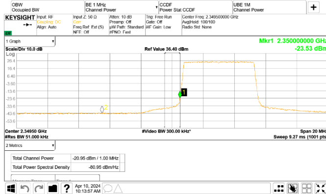
Figure 8.2-145: Conducted emission from the lower band edge
