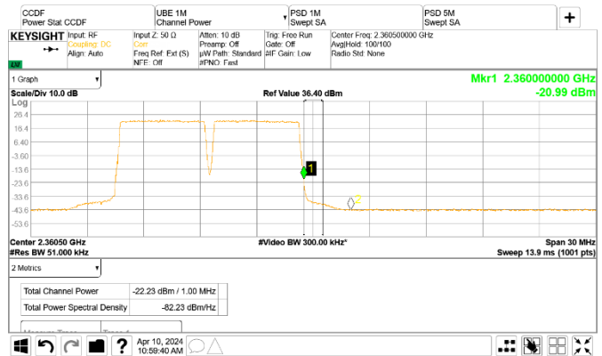
Figure 8.2-156: Conducted emission from the upper band edge
