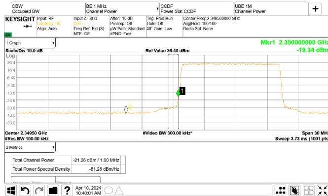
Figure 8.2-151: Conducted emission from the lower band edge
