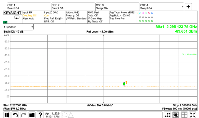
Figure 8.2-88: Conducted spurious emissions of NR 5 MHz top channel, single carrier operation [2.2875 GHz to 2.30 GHz]
