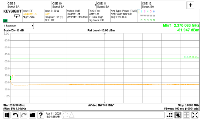
Figure 8.2-130: Conducted spurious emissions of Multi RAT operation, NR 5 MHz + LTE 5 MHz [2.70 GHz to 3 GHz]
