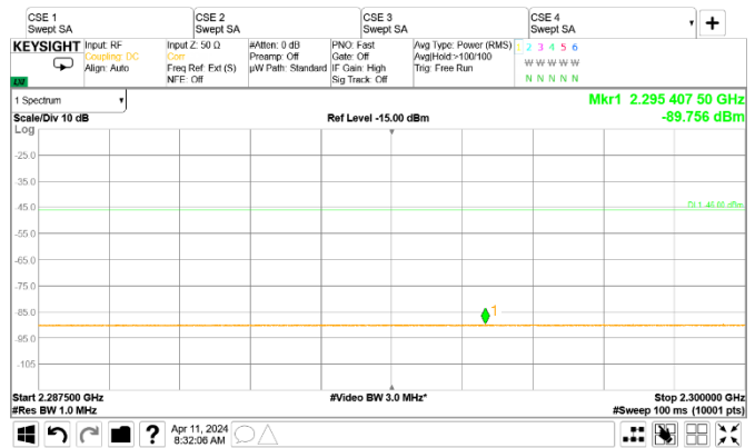
Figure 8.2-124: Conducted spurious emissions of Multi RAT operation, NR 5 MHz + LTE 5 MHz [2.2875 GHz to 2.30 GHz]
