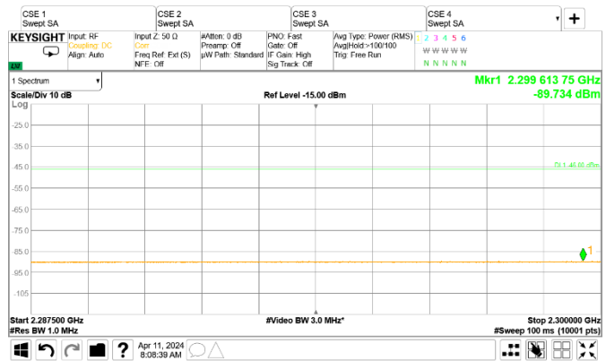
Figure 8.2-76: Conducted spurious emissions of NR 5 MHz mid channel, single carrier operation [2.2875 GHz to 2.30 GHz]
