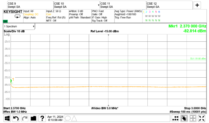
Figure 8.2-82: Conducted spurious emissions of NR 5 MHz mid channel, single carrier operation [2.70 GHz to 3 GHz]
