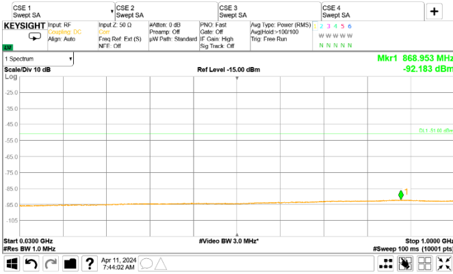
Figure 8.2-37: Conducted spurious emissions of LTE 10 MHz, single carrier operation [30 MHz to 1 GHz]
