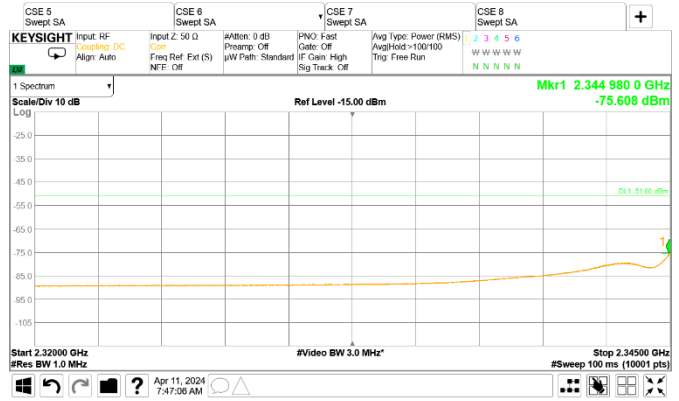
Figure 8.2-42: Conducted spurious emissions of LTE 10 MHz, single carrier operation [2.32 GHz to 2.345 GHz]
