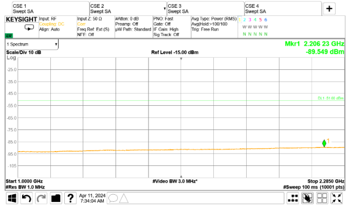
Figure 8.2-14: Conducted spurious emissions of LTE 5 MHz mid channel, single carrier operation [1 GHz to 2.285 GHz]
