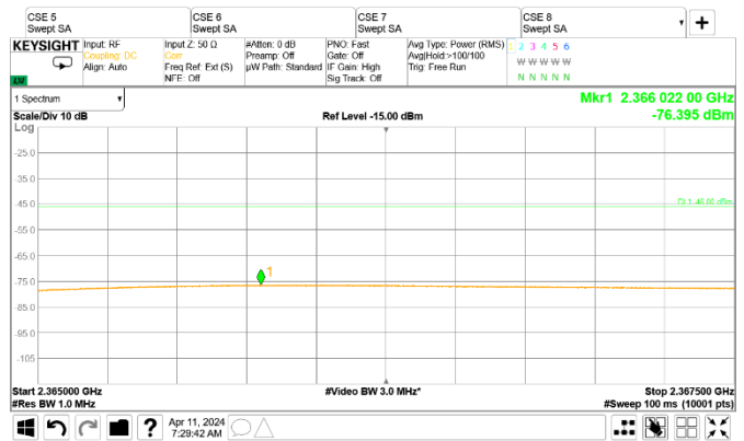
Figure 8.2-8: Conducted spurious emissions of LTE 5 MHz low channel, single carrier operation [2.365 GHz to 2.3675 GHz]
