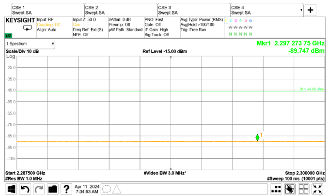
Figure 8.2-16: Conducted spurious emissions of LTE 5 MHz mid channel, single carrier operation [2.2875 GHz to 2.30 GHz]
