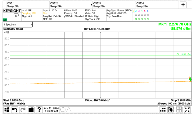
Figure 8.2-38: Conducted spurious emissions of LTE 10 MHz, single carrier operation [1 GHz to 2.285 GHz]
