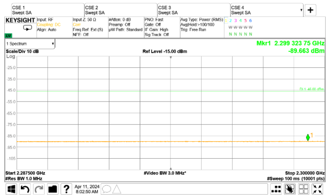
Figure 8.2-64: Conducted spurious emissions of NR 5 MHz low channel, single carrier operation [2.2875 GHz to 2.30 GHz]
