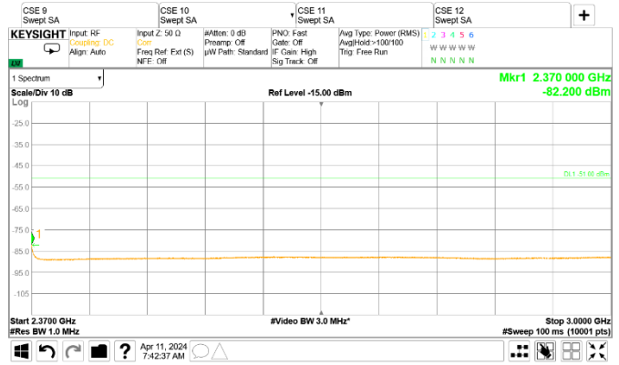
Figure 8.2-34: Conducted spurious emissions of LTE 5 MHz top channel, single carrier operation [2.70 GHz to 3 GHz]
