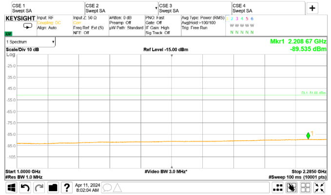
Figure 8.2-62: Conducted spurious emissions of NR 5 MHz low channel, single carrier operation [1 GHz to 2.285 GHz]
