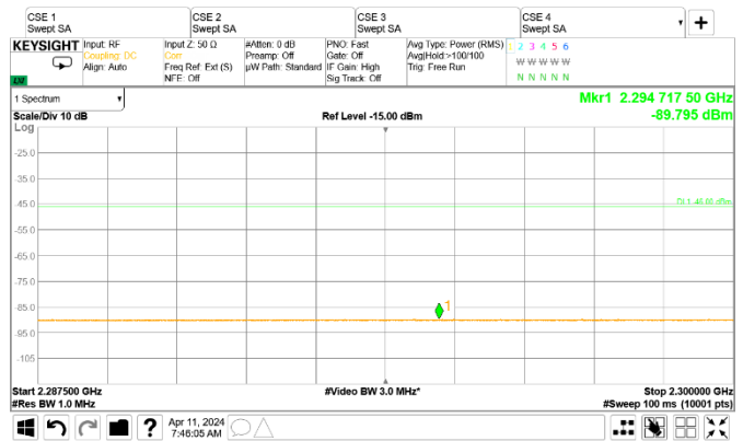
Figure 8.2-40: Conducted spurious emissions of LTE 10 MHz, single carrier operation [2.2875 GHz to 2.30 GHz]
