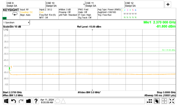
Figure 8.2-58: Conducted spurious emissions of LTE 5 MHz, Contiguous Channels, two carrier operation [2.70 GHz to 3 GHz]
