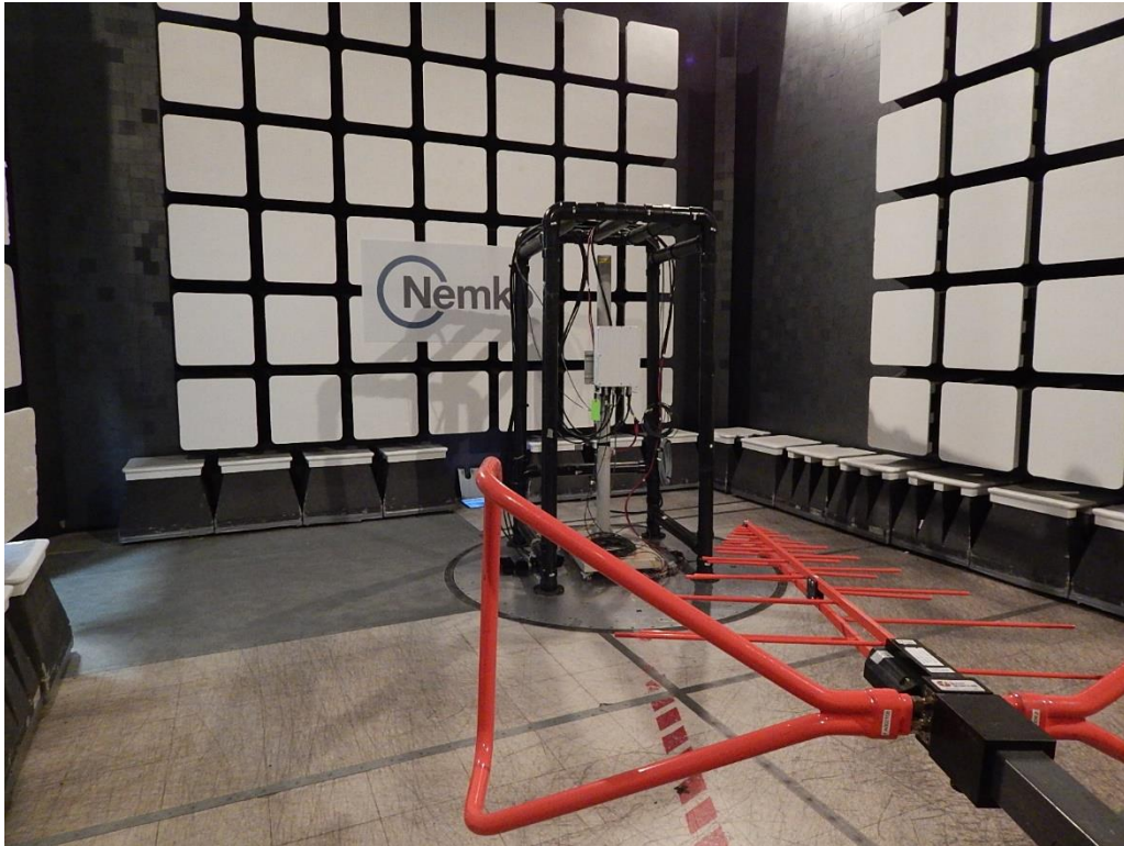
Figure 3.5-3: EUT Set-up photo for Radiated Emissions [30 MHz to 1000 MHz]
