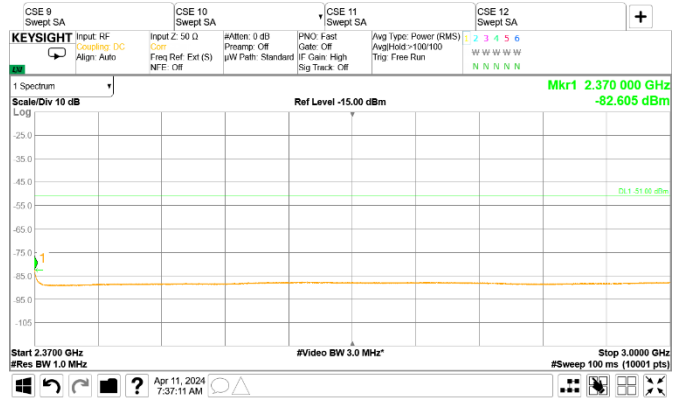
Figure 8.2-22: Conducted spurious emissions of LTE 5 MHz mid channel, single carrier operation [2.70 GHz to 3 GHz]
