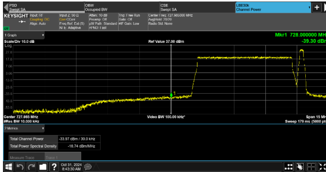
Figure 8.2-199: Conducted emission at the lower band edge
