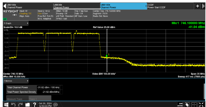
Figure 8.2-182: Conducted emission 100 kHz away from the upper band edge
