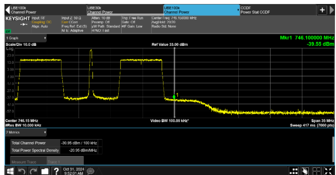
Figure 8.2-214: Conducted emission 100 kHz away from the upper band edge
