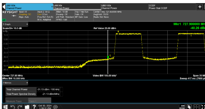
Figure 8.2-160: Conducted emission 100 kHz away from the lower band edge
