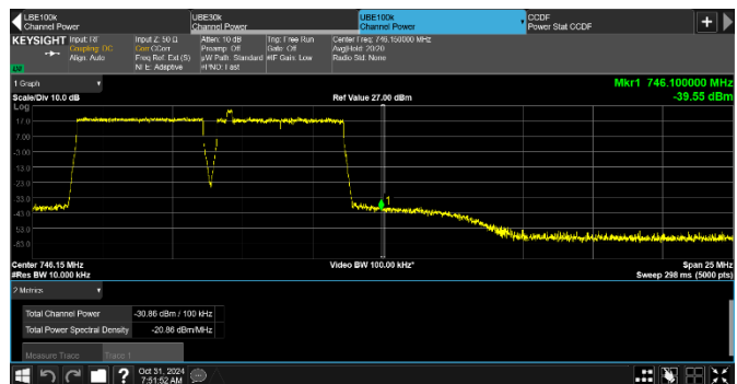
Figure 8.2-174: Conducted emission 100 kHz away from the band edge
