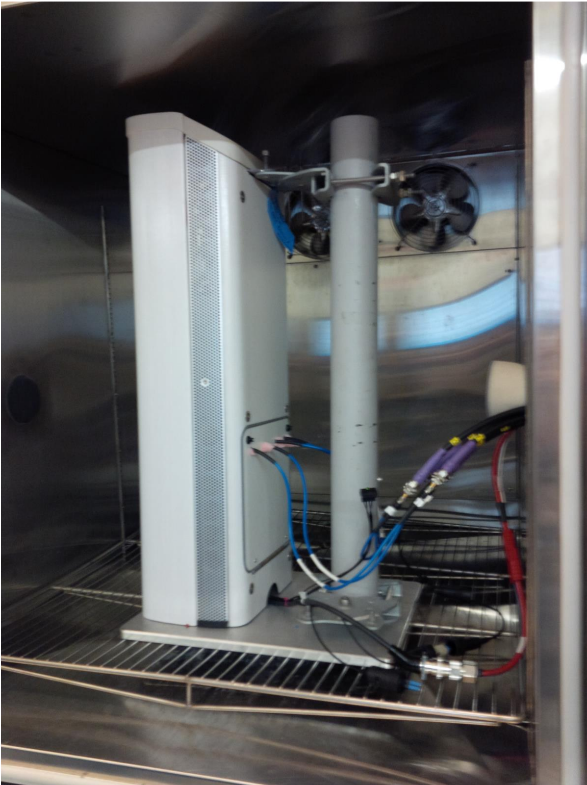
Figure 2: EUT in a thermal test chamber
