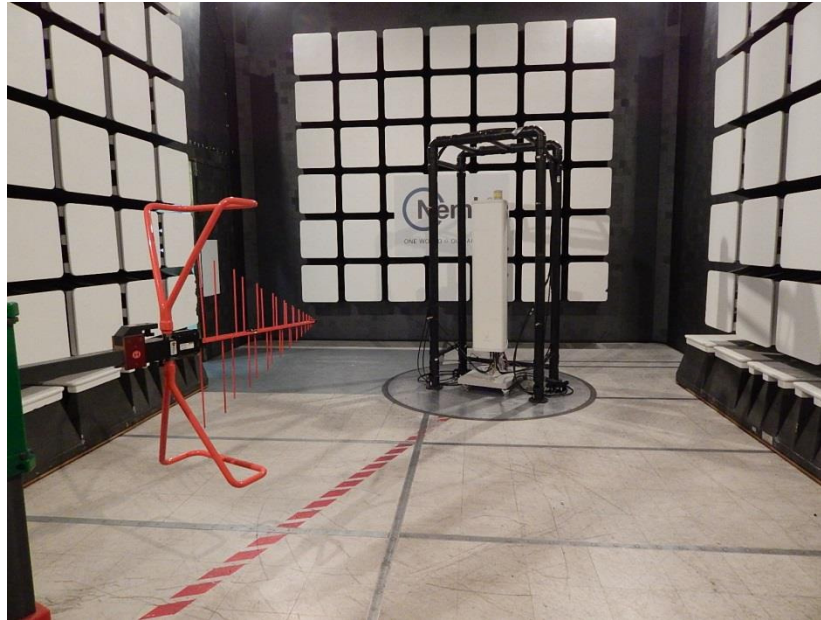
Figure 8.1-37: Setup photo – 30 to 1000 MHz
