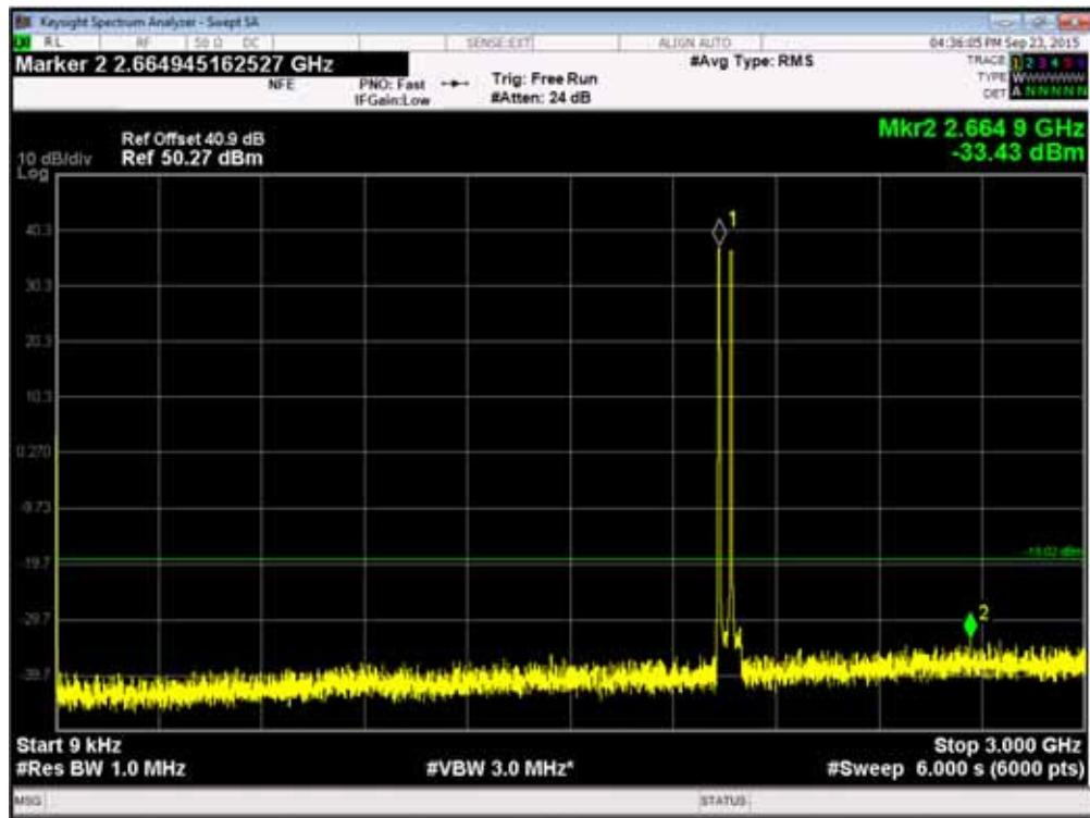
Channel Position B<sub>RFBW</sub> - WCDMA 16QAM / LTE QPSK: Bandwidth 5.0 MHz - 3GHz - 10GHz
