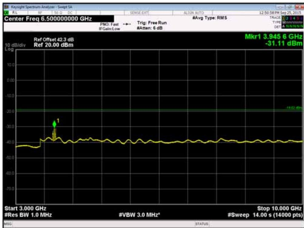
Channel Position  $T_{RFBW}$  - WCDMA 16QAM / LTE QPSK: Bandwidth 5.0 MHz - 10GHz - 20GHz
