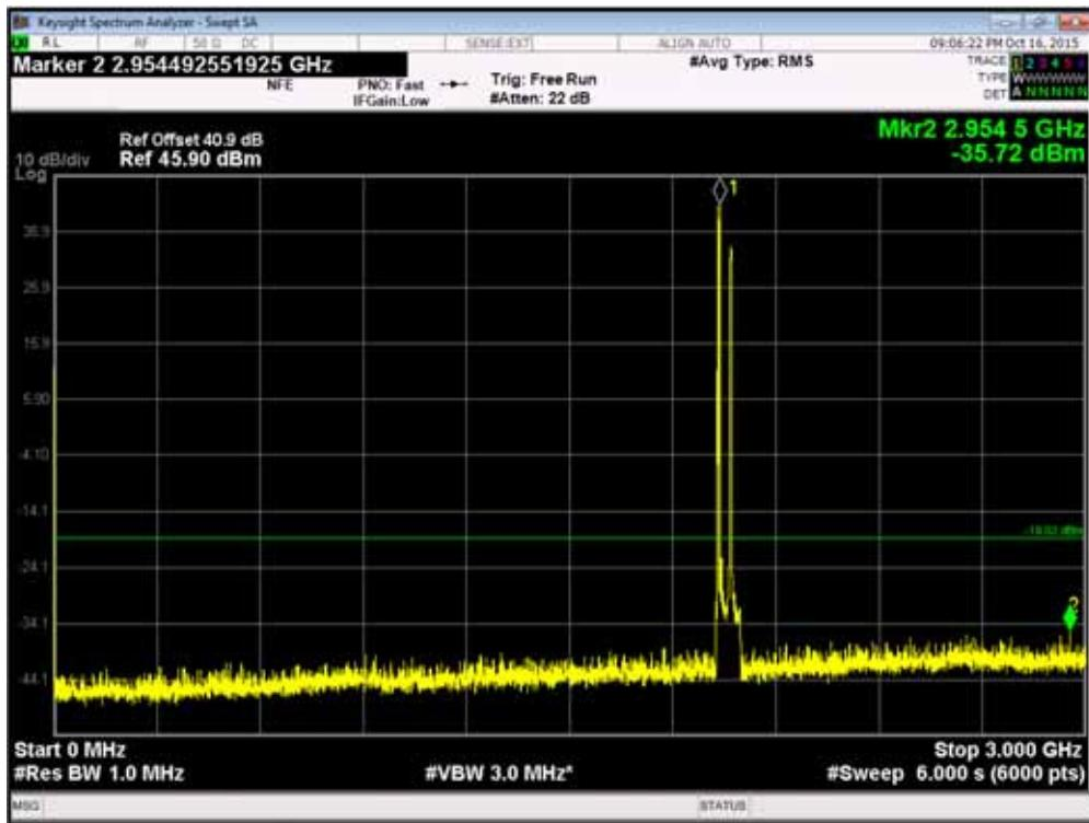
Channel Position  $B_{RFBW}$  - GSM GMSK / WCDMA 16QAM: Bandwidth 5.0 MHz - 3GHz - 10GHz
