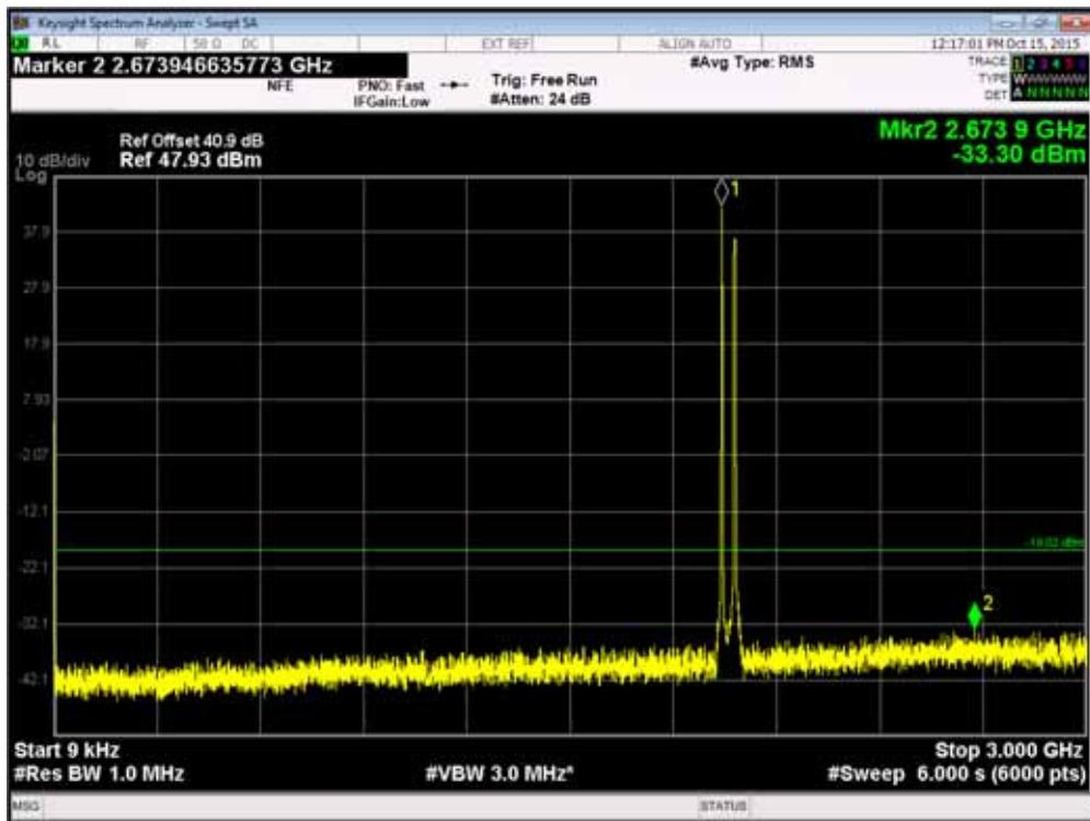
Channel Position M<sub>RFBW</sub> - GSM GMSK / LTE QPSK: Bandwidth 5.0 MHz - 3GHz - 10GHz
