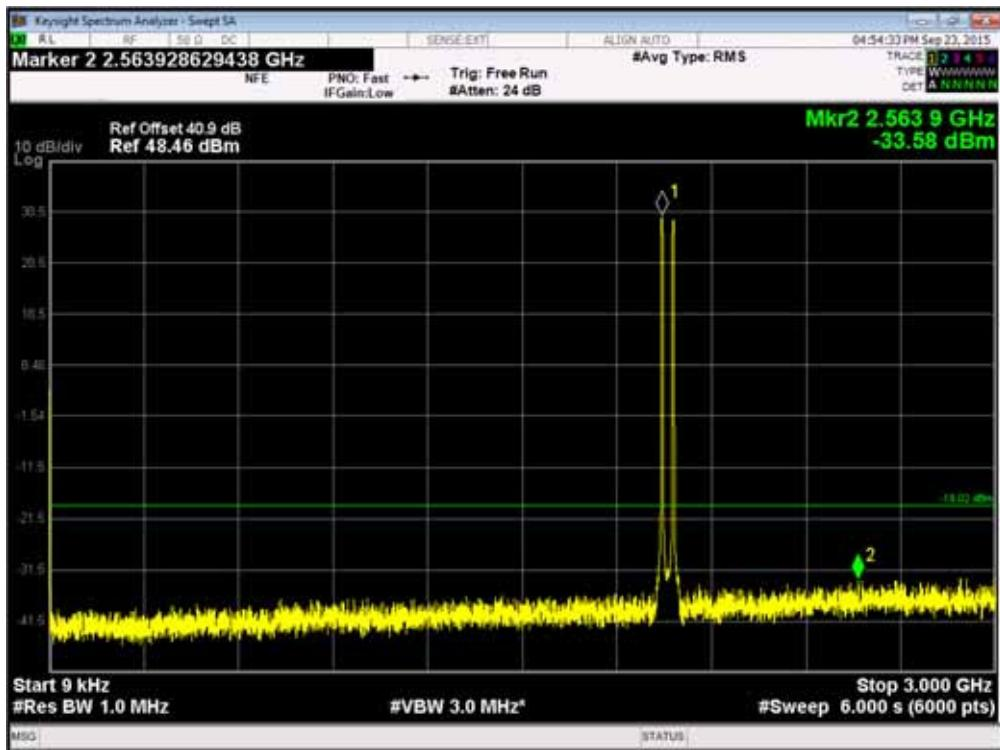
Channel Position M<sub>RFBW</sub> - WCDMA 16QAM / LTE QPSK: Bandwidth 5.0 MHz - 3GHz - 10GHz
