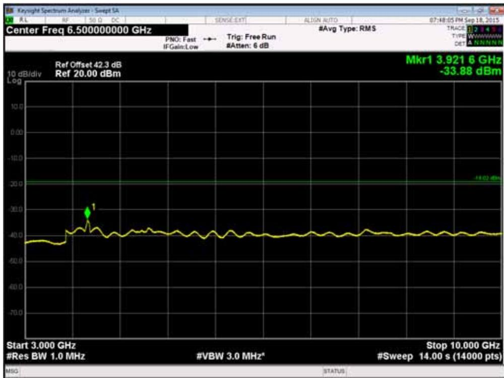
Channel Position M<sub>RFBW</sub> - QPSK / Bandwidth 20.0MHz - 10GHz - 20GHz
