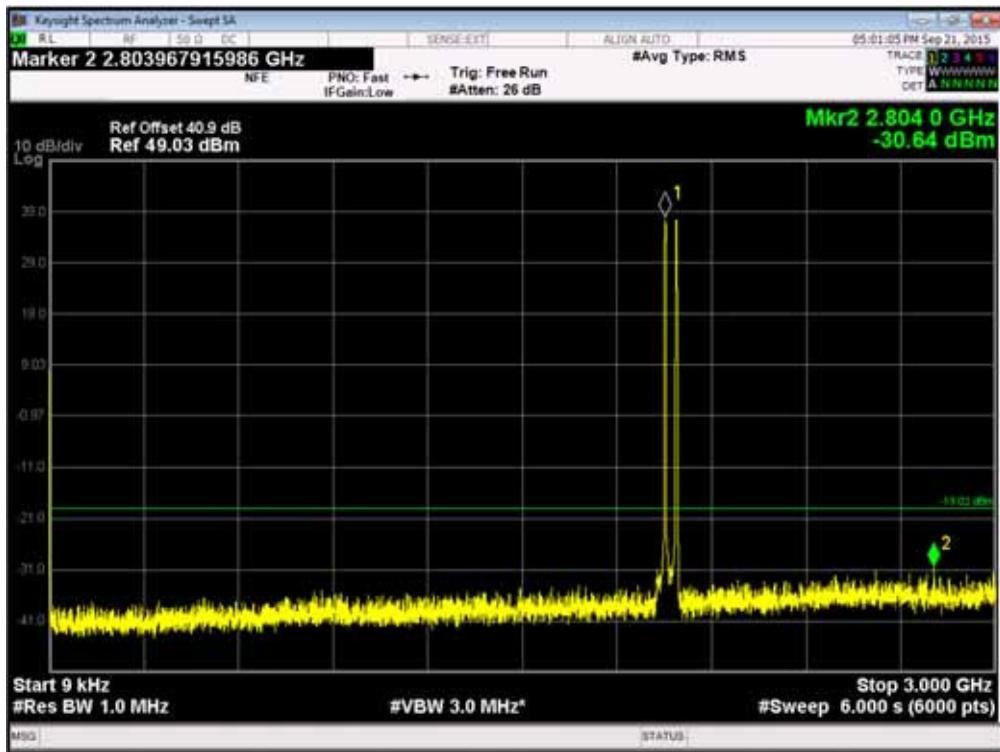
Channel Position  $T_{RFBW}$  - 16QAM / Bandwidth 5.0MHz - 10GHz
