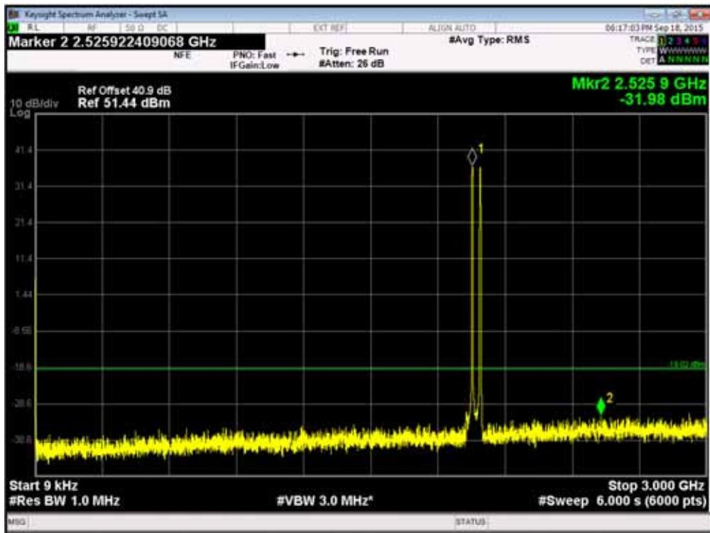
Channel Position  $T_{RFBW}$  - QPSK / Bandwidth 5.0MHz - 3GHz - 10GHz
