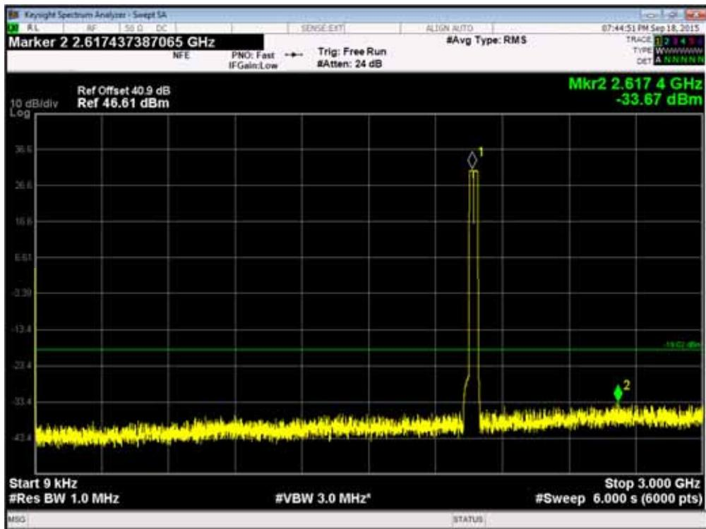
Channel Position  $T_{RFBW}$  - QPSK / Bandwidth 20.0MHz - 3GHz - 10GHz
