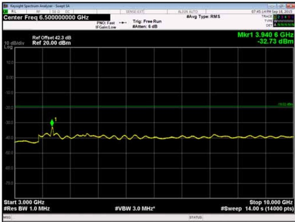
Channel Position  $T_{RFBW}$  - QPSK / Bandwidth 20.0MHz - 10GHz - 20GHz
