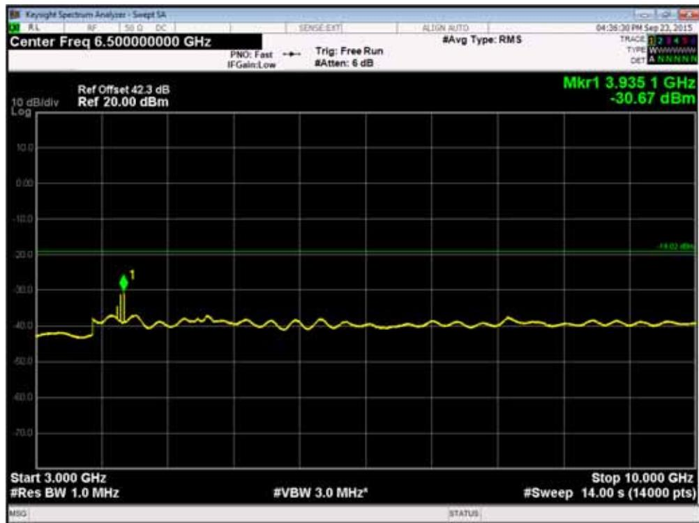
Channel Position B<sub>RFBW</sub> - WCDMA 16QAM / LTE QPSK: Bandwidth 5.0 MHz - 10GHz - 20GHz
