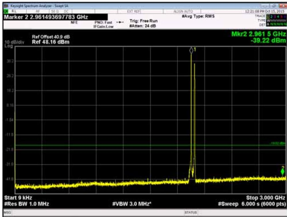
Channel Position  $T_{RFBW}$  - GSM GMSK / LTE QPSK: Bandwidth 5.0 MHz - 3GHz - 10GHz
