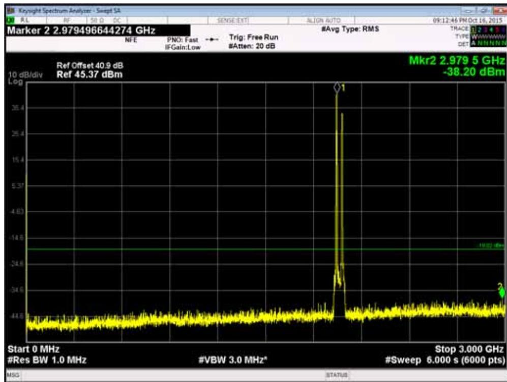
Channel Position M<sub>RFBW</sub> - GSM GMSK / WCDMA 16QAM: Bandwidth 5.0 MHz - 3GHz - 10GHz
