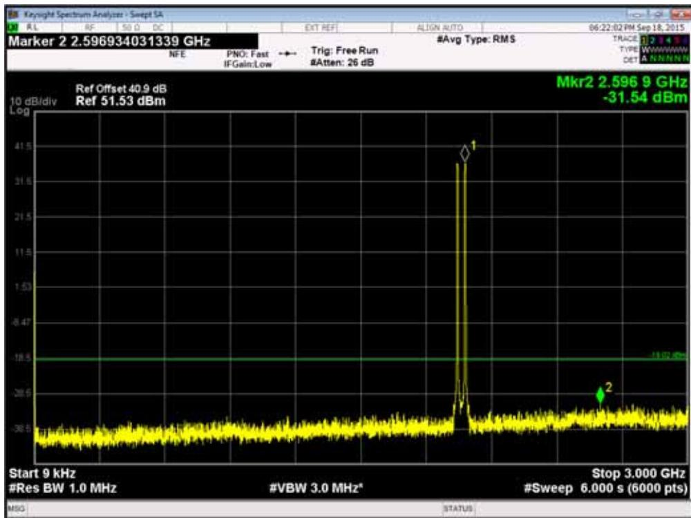
Channel Position M<sub>RFBW</sub> - QPSK / Bandwidth 5.0MHz - 3GHz - 10GHz
