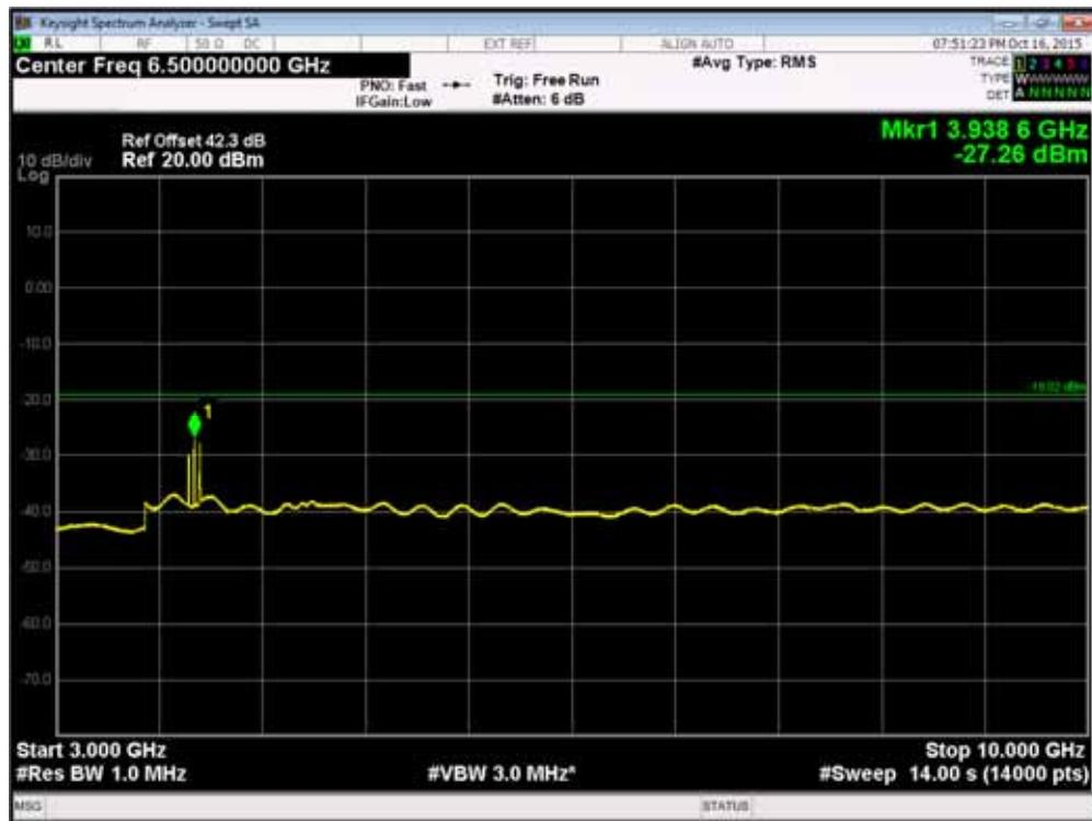
Channel Position  $T_{RFBW}$  - GSM GMSK / WCDMA 16QAM: Bandwidth 5.0 MHz - 10GHz - 20GHz
