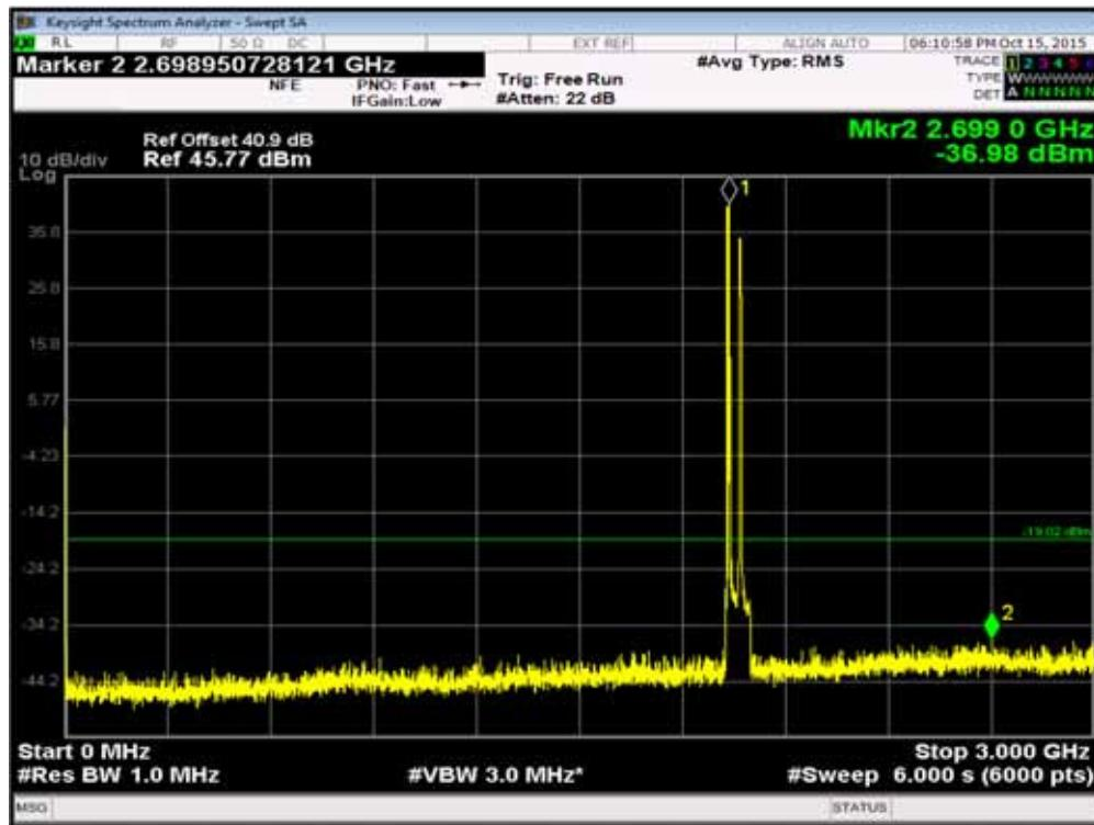
Channel Position B<sub>RFBW</sub> - GSM GMSK / LTE QPSK: Bandwidth 5.0 MHz - 3GHz - 10GHz
