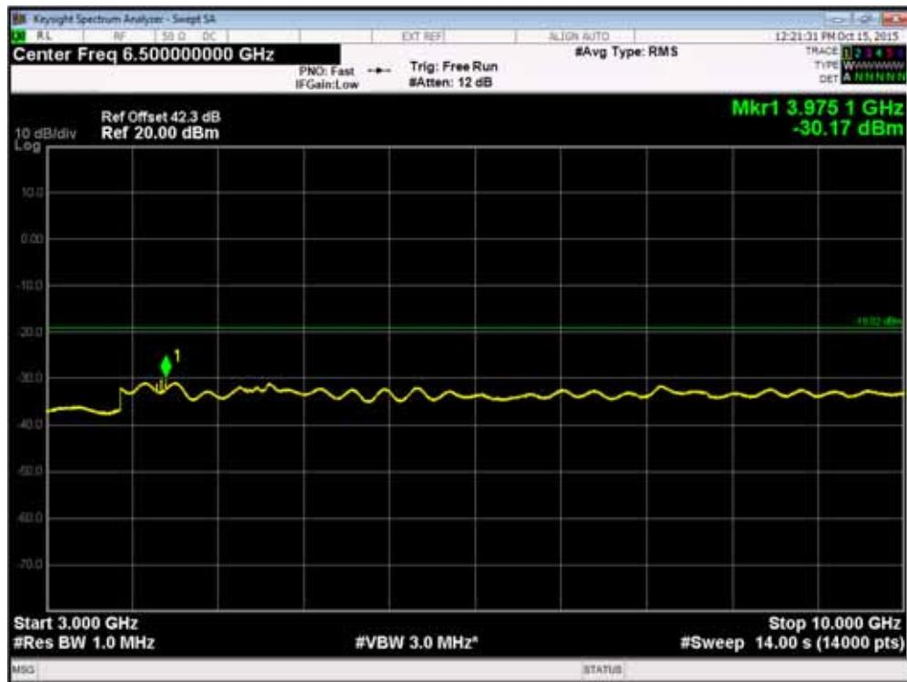
Channel Position  $T_{RFBW}$  - GSM GMSK / LTE QPSK: Bandwidth 5.0 MHz - 10GHz - 20GHz
