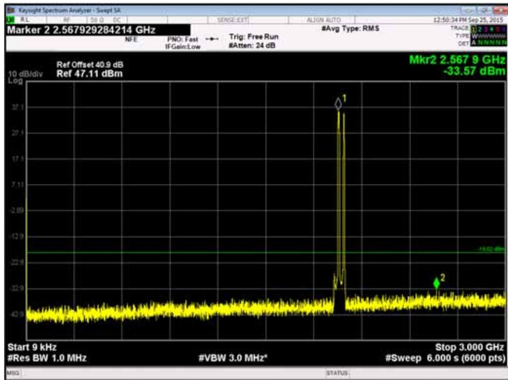
Channel Position  $T_{RFBW}$  - WCDMA 16QAM / LTE QPSK: Bandwidth 5.0 MHz - 3GHz - 10GHz
