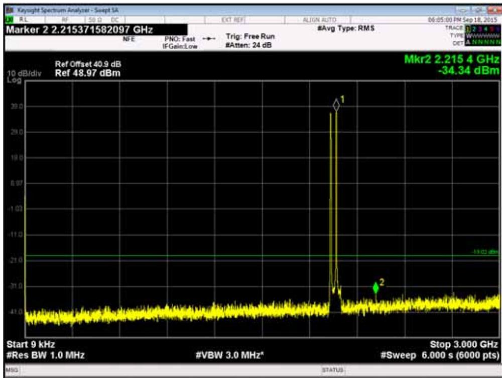
Channel Position B<sub>RFBW</sub> - QPSK / Bandwidth 5.0 MHz - 3GHz - 10GHz
