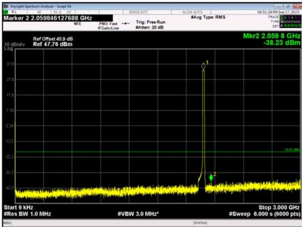
Channel Position T - QPSK / Bandwidth 20.0MHz - 3GHz - 10GHz
