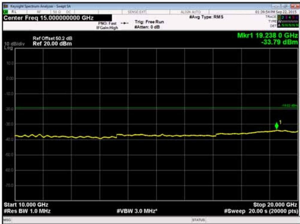
Channel Position  $T_{RFBW}$  - 16QAM / Bandwidth 5.0MHz - 9GHz
