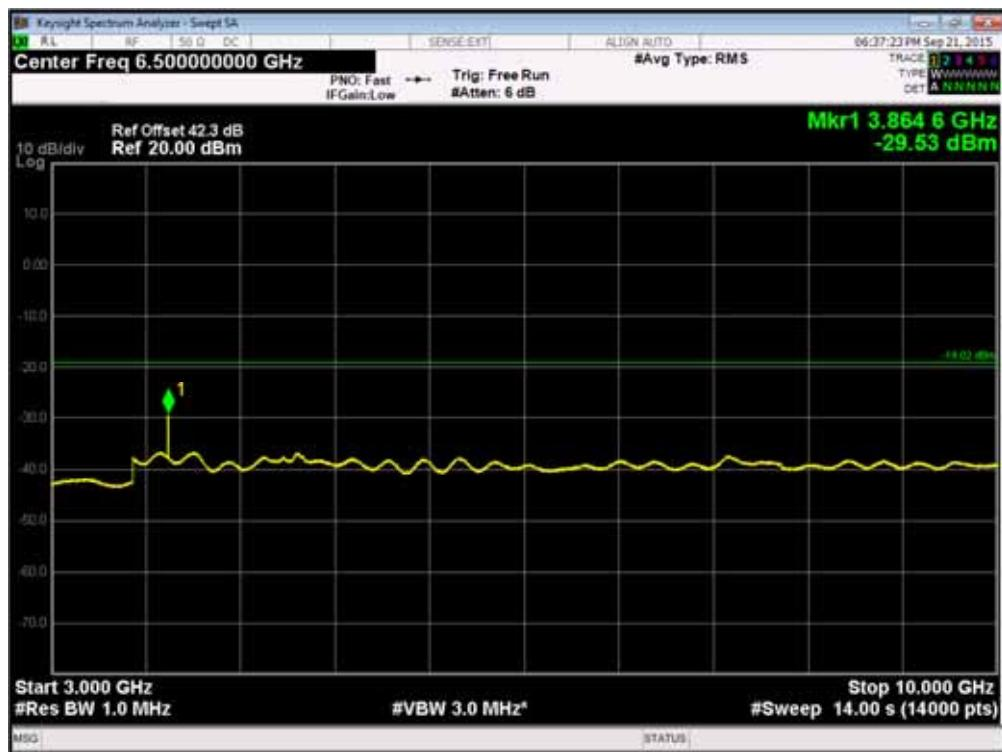
Channel Position B - 16QAM / Bandwidth 5.0MHz - 10GHz - 20GHz
