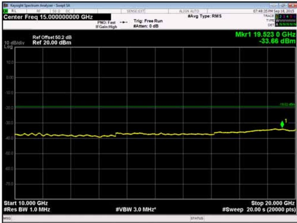
Channel Position T<sub>RFBW</sub> - QPSK / Bandwidth 20.0MHz - 9kHz - 3GHz
