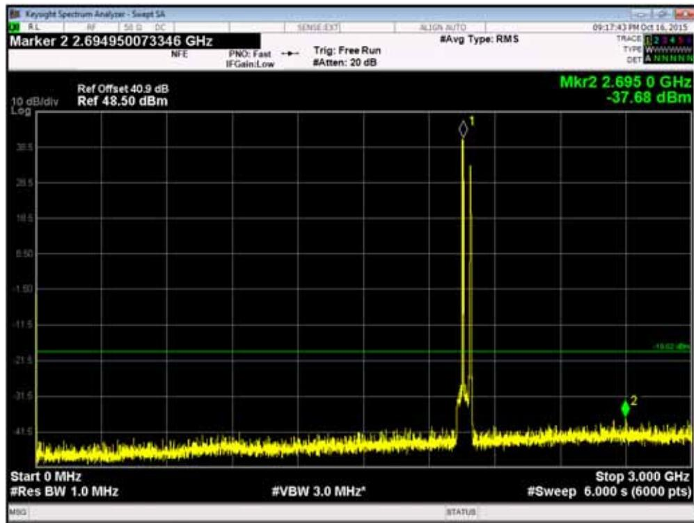
Channel Position  $T_{RFBW}$  - GSM GMSK / WCDMA 16QAM: Bandwidth 5.0 MHz - 3GHz - 10GHz
