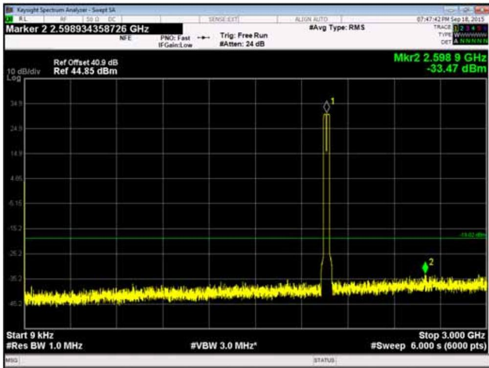
Channel Position M<sub>RFBW</sub> - QPSK / Bandwidth 20.0MHz - 3GHz - 10GHz
