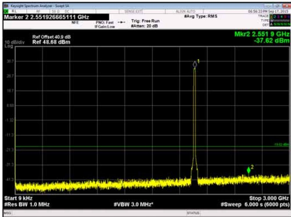
Channel Position M - QPSK / Bandwidth 20.0MHz - 3GHz - 10GHz
