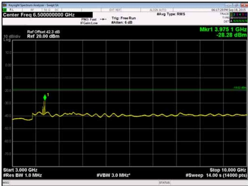
Channel Position  $T_{RFBW}$  - QPSK / Bandwidth 5.0MHz - 10GHz - 20GHz
