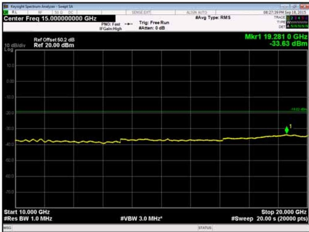
Channel Position  $T_{RFBW}$  - QPSK / Bandwidth 5.0MHz - 9kHz - 3GHz
