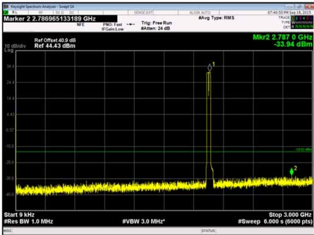
Channel Position B<sub>RFBW</sub> - QPSK / Bandwidth 20.0MHz - 3GHz - 10GHz
