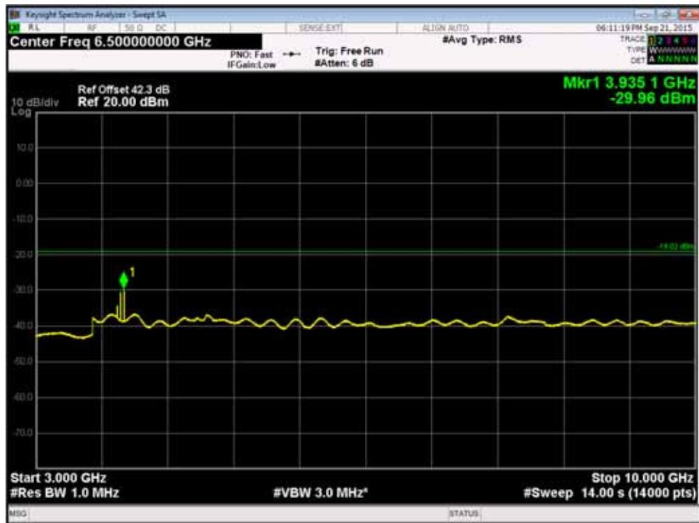
Channel Position B<sub>RFBW</sub> - 16QAM / Bandwidth 5.0MHz - 10GHz - 20GHz
