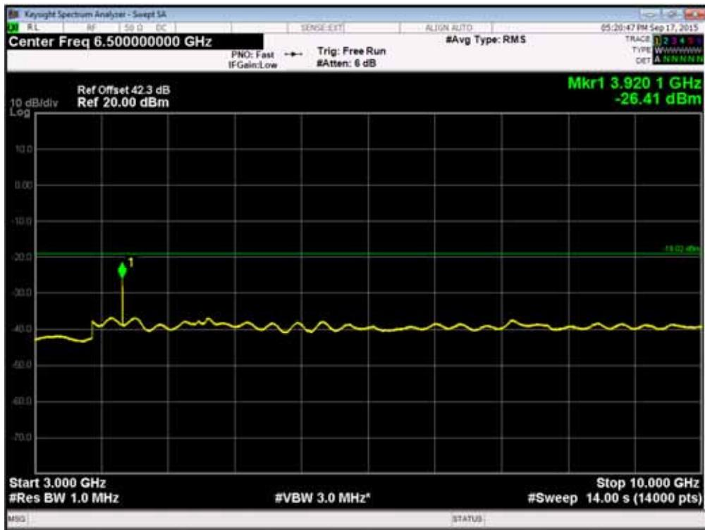
Channel Position M - QPSK / Bandwidth 5.0MHz - 10GHz - 20GHz
