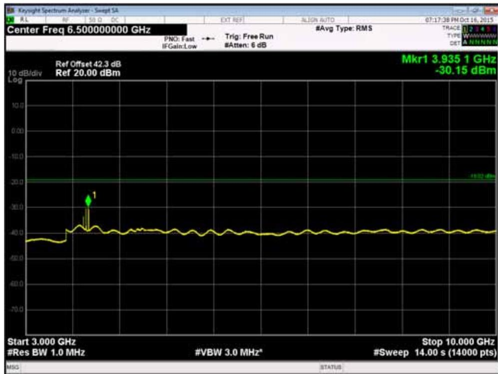
Channel Position  $B_{RFBW}$  - GSM GMSK / WCDMA 16QAM: Bandwidth 5.0 MHz - 10GHz - 20GHz
