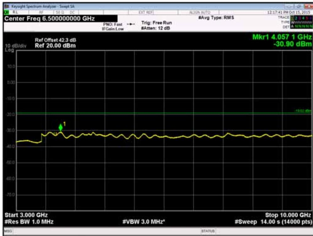
Channel Position M<sub>RFBW</sub> - GSM GMSK / LTE QPSK: Bandwidth 5.0 MHz - 10GHz - 20GHz
