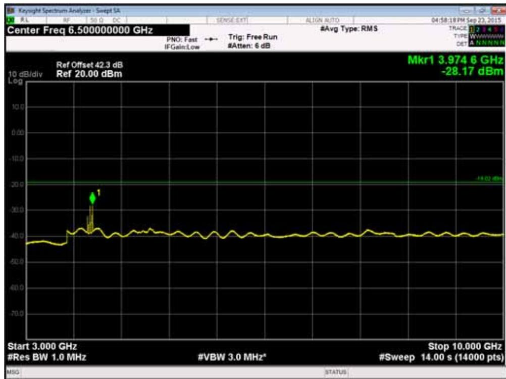
Channel Position  $T_{RFBW}$  - WCDMA 16QAM / LTE QPSK: Bandwidth 5.0 MHz - 10GHz - 20GHz
