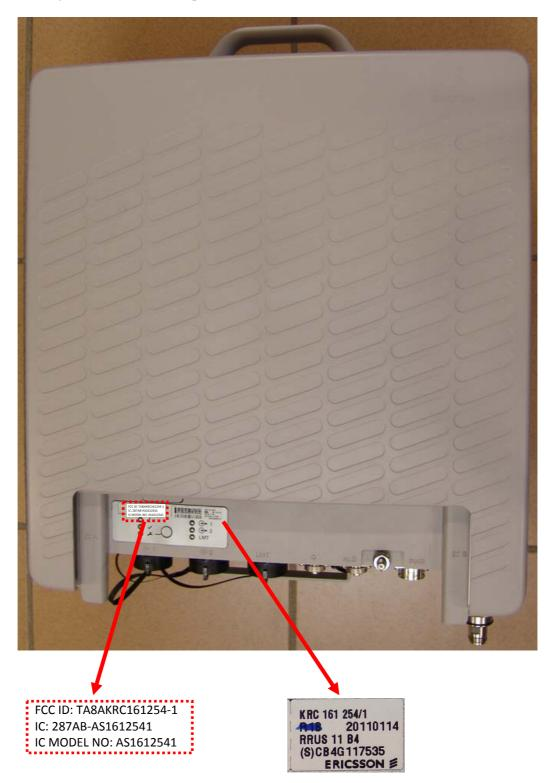
Note: The product label of the tested sample shows revision R1B instead of correct revision R1C. The hardware tested was modified to reflect R1C revision status.
