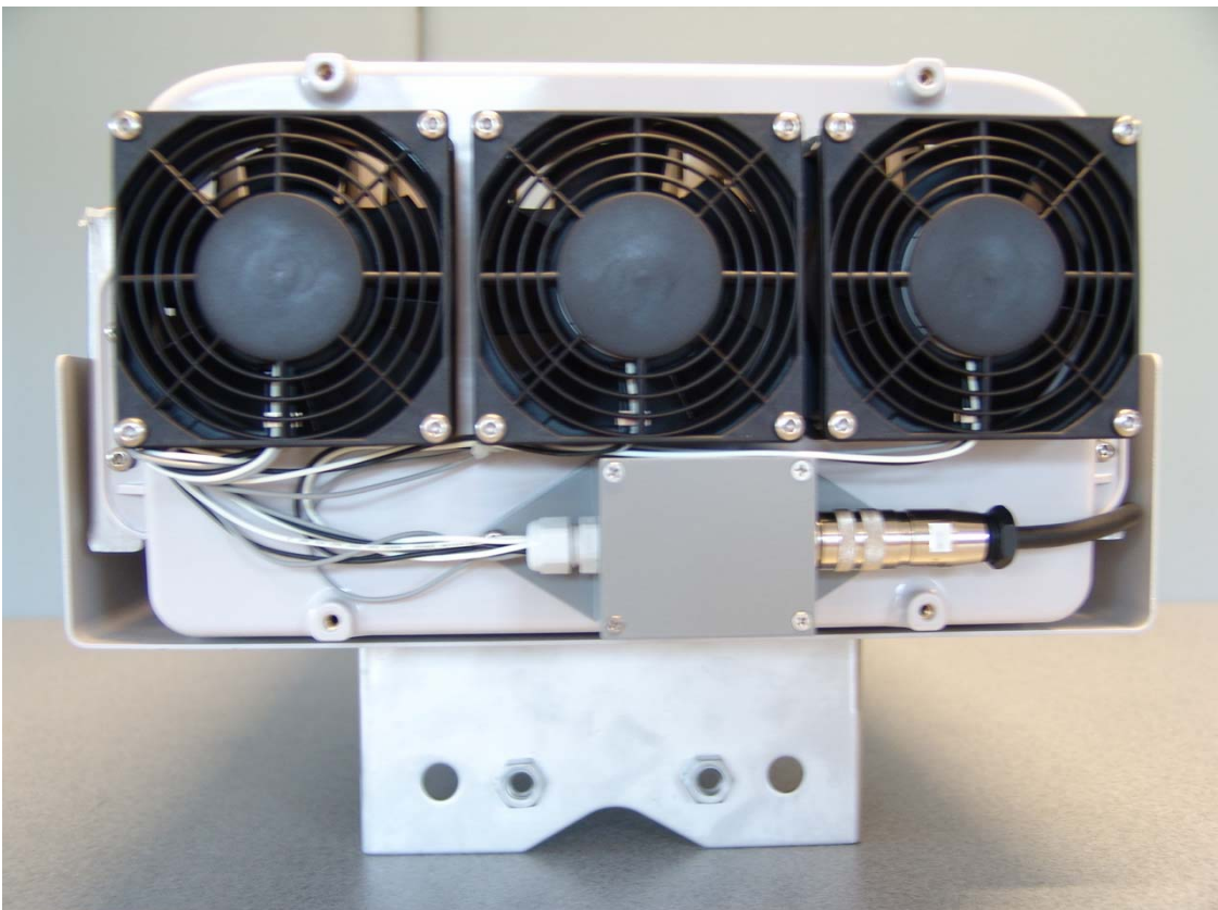
View on top side fan units (solar cover removed)
