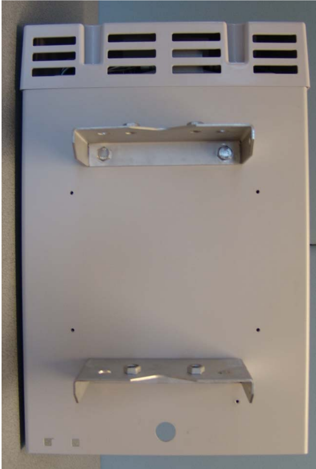
Rear side, DC-configuration (PSU and ACCU removed)
