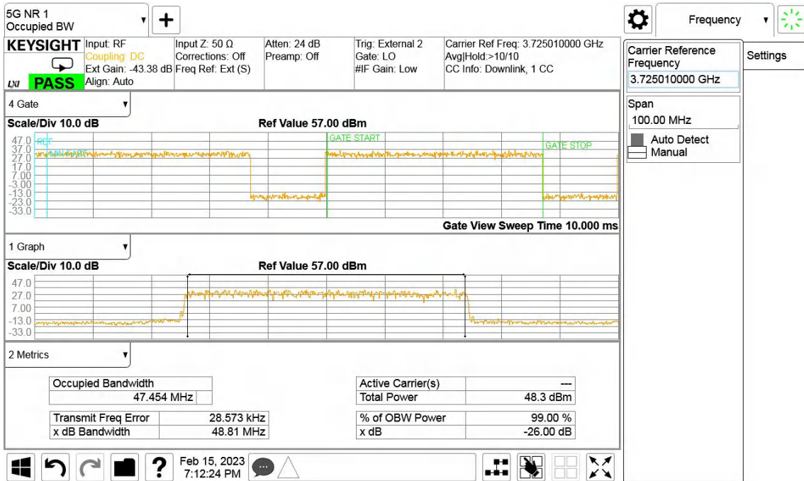
QPSK, 50MHz, Channel position B, B77D
