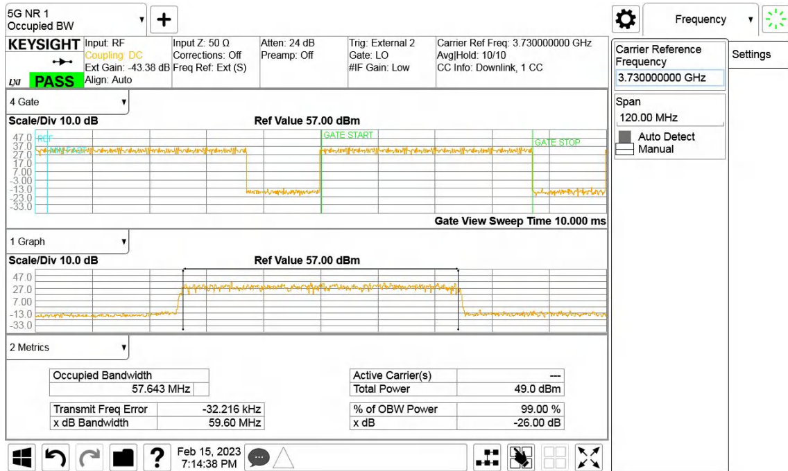
QPSK, 60MHz, Channel position B, B77D
