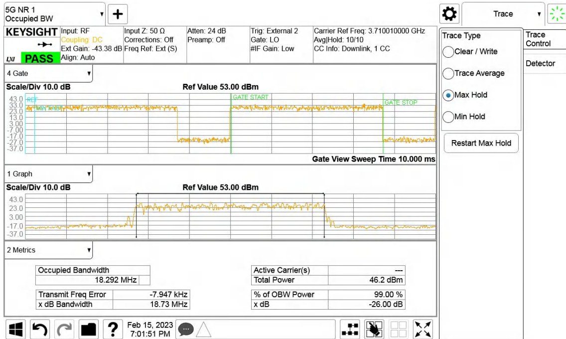
QPSK, 20MHz, Channel position B, B77D
