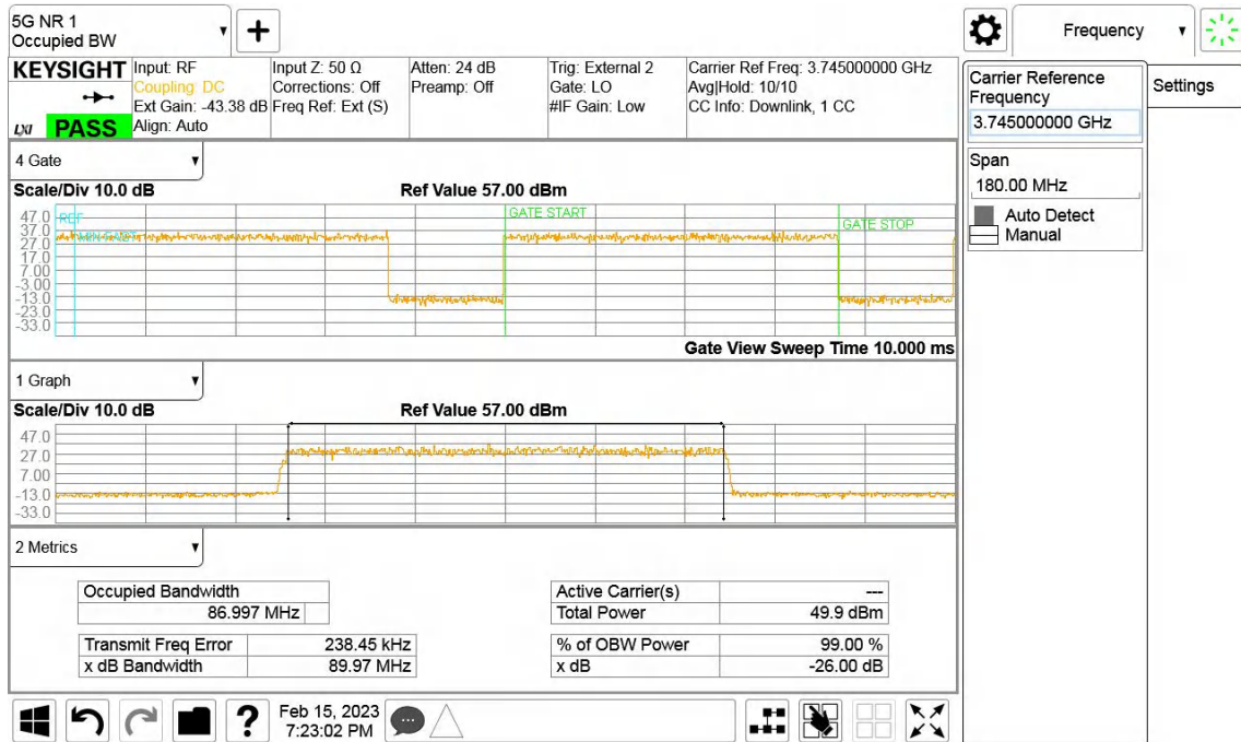
QPSK, 90MHz, Channel position B, B77D
