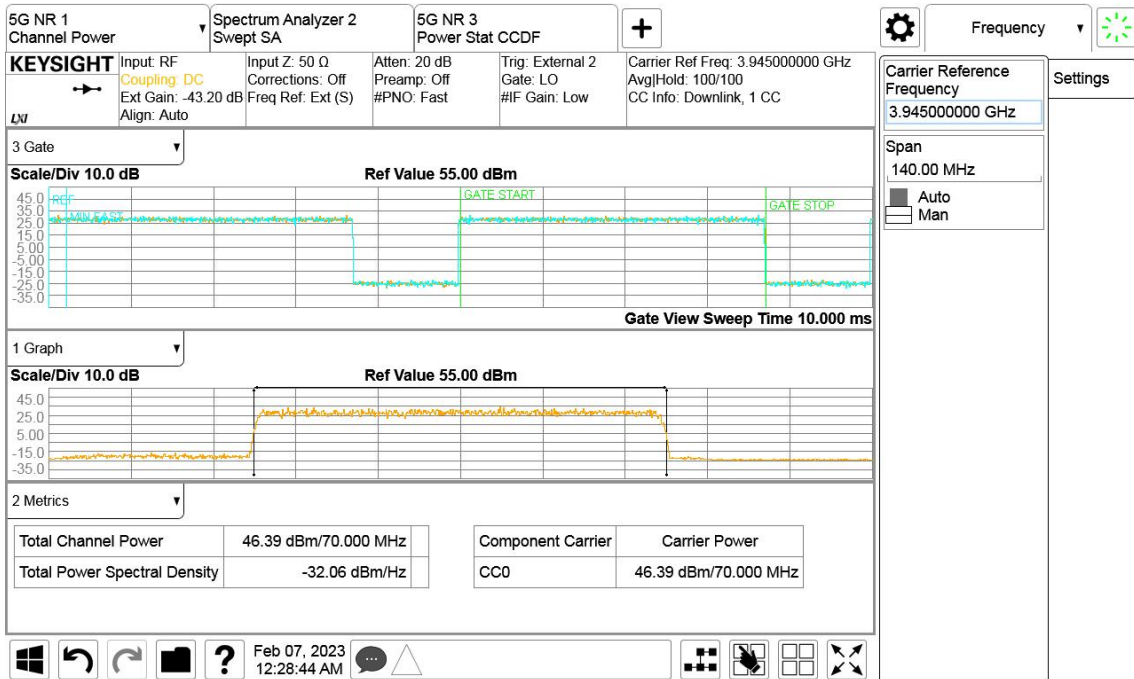
B77D,Power, Port B, NR-1C, 64QAM, 70MHz, Channel position H
