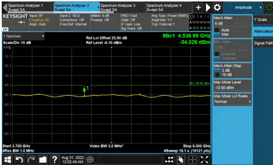
Channel Position T, 3700MHz to 6GHz
