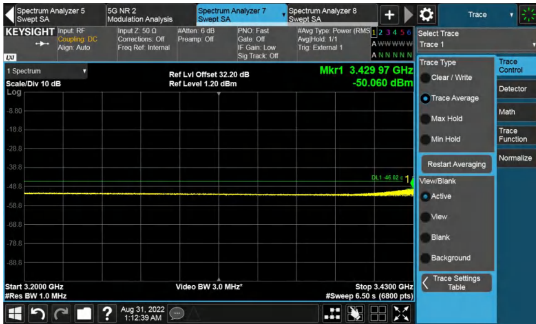
Channel Position T, 3200MHz to 3430MHz
