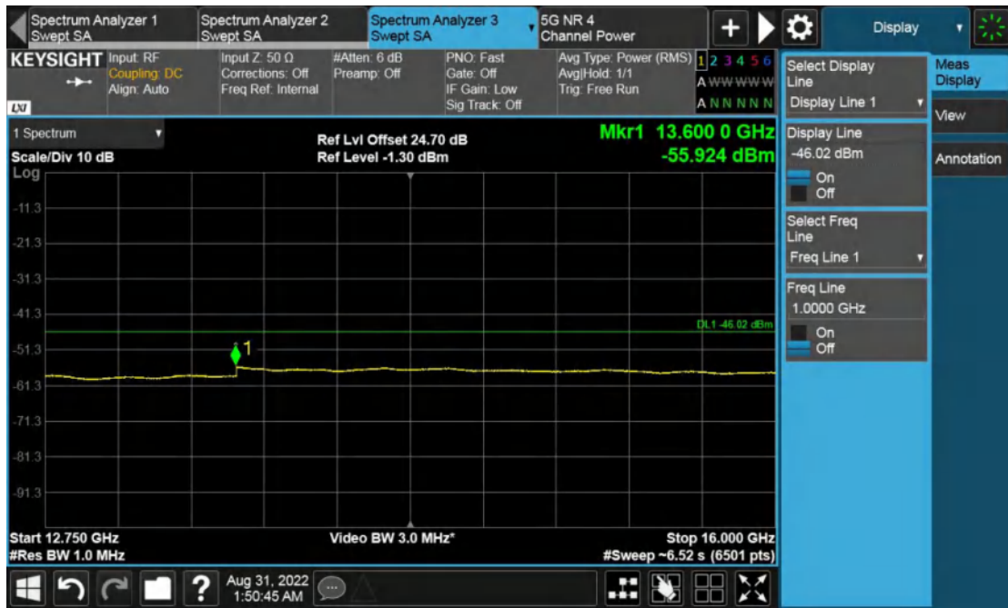
Channel Position T, 12.75GHz to 16GHz
