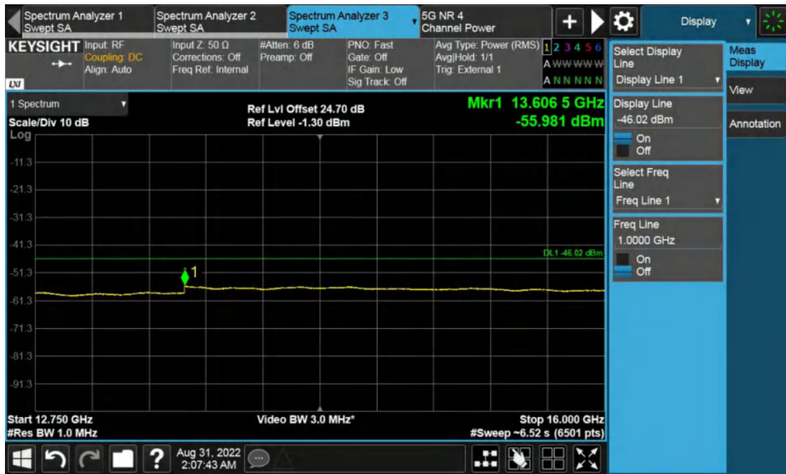
Channel Position M, 12.75GHz to 16GHz
