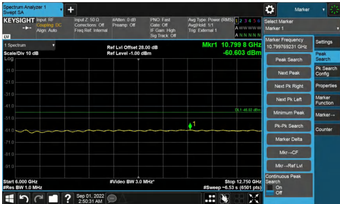
Channel Position T, 6GHz to 12.75GHz
