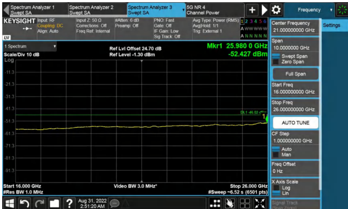
Channel Position B, 16GHz to 26GHz
