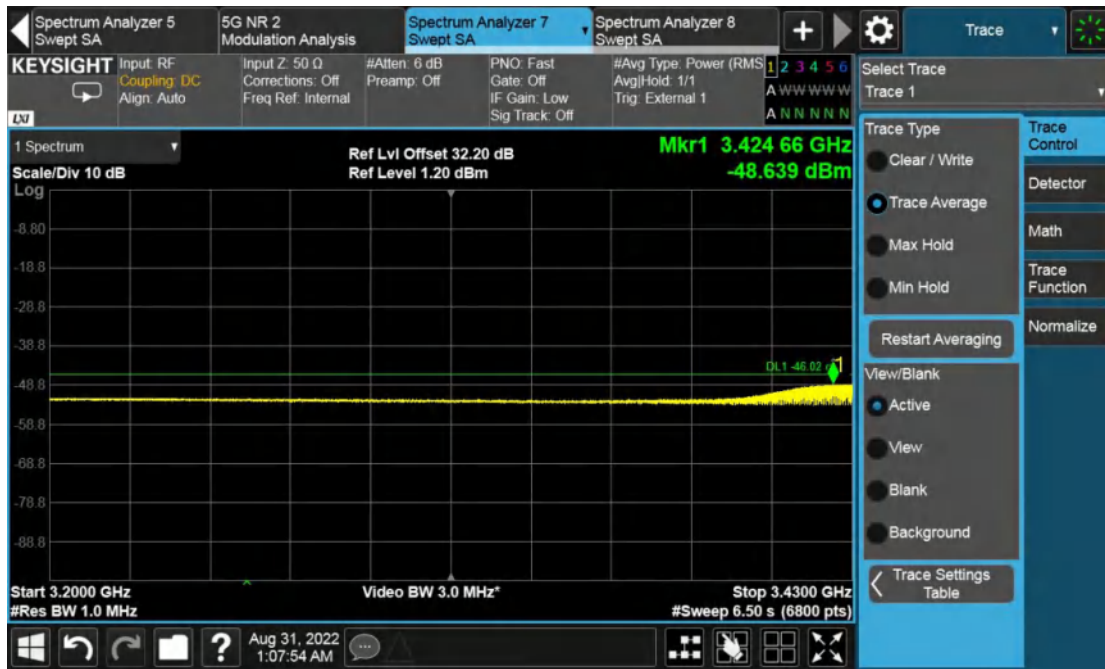
Channel Position B, 3200MHz to 3430MHz
