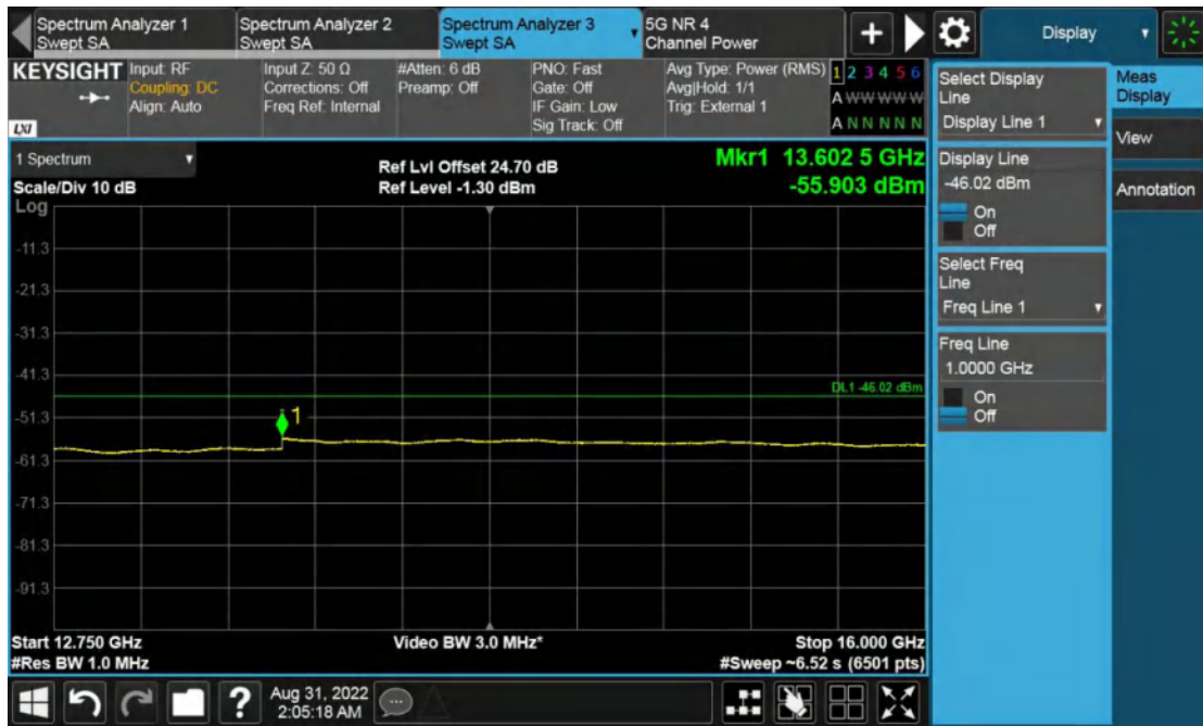
Channel Position B, 12.75GHz to 16GHz
