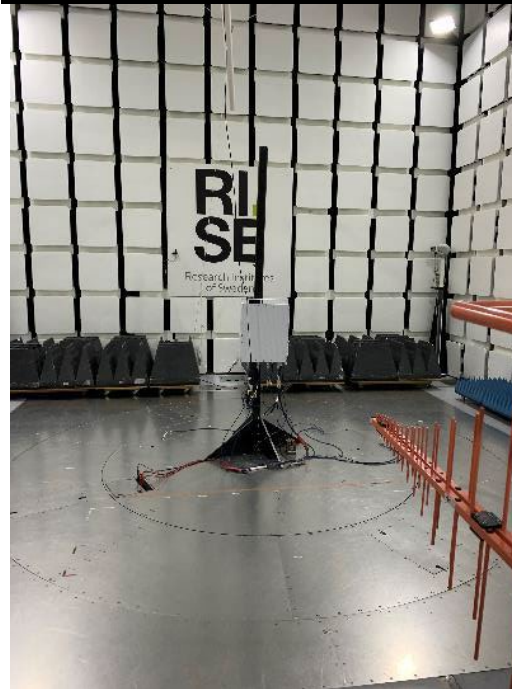
Test setup 30-1000 MHz:
