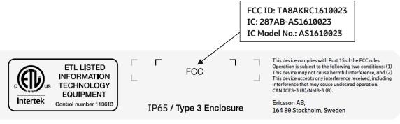
Below picture shows where the labels are placed on the radio.
