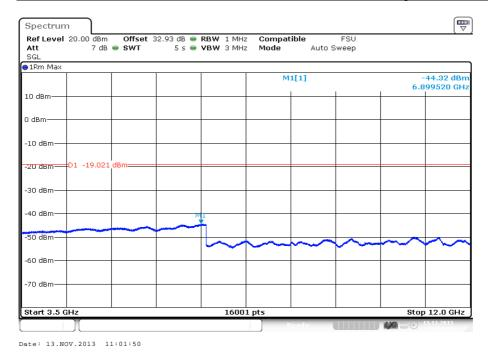
Channel Position M - Carrier Bandwidth 20.0 MHz - Band 3 - Range 12000 to 20000 MHz
