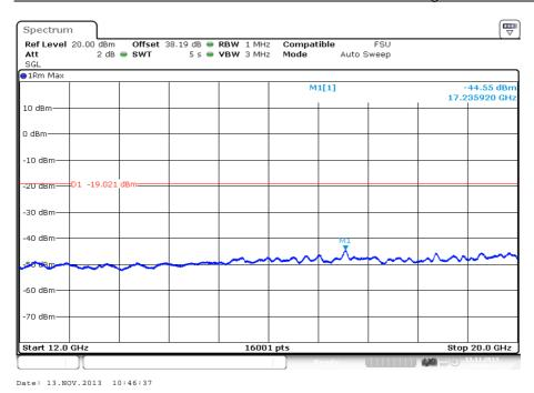
Channel Position T - Carrier Bandwidth 20.0 MHz - Band 1 - Range 0.009 to 3500 MHz
