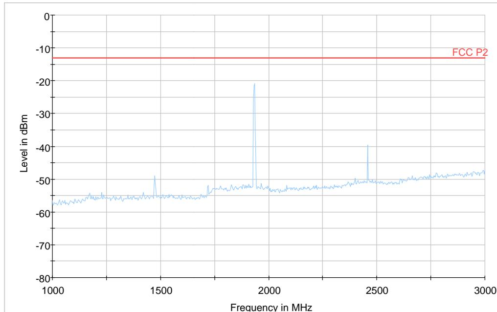
Note: The emission between 1930 and 1990 MHz are the carrier frequencies and shall be ignored in the context.
