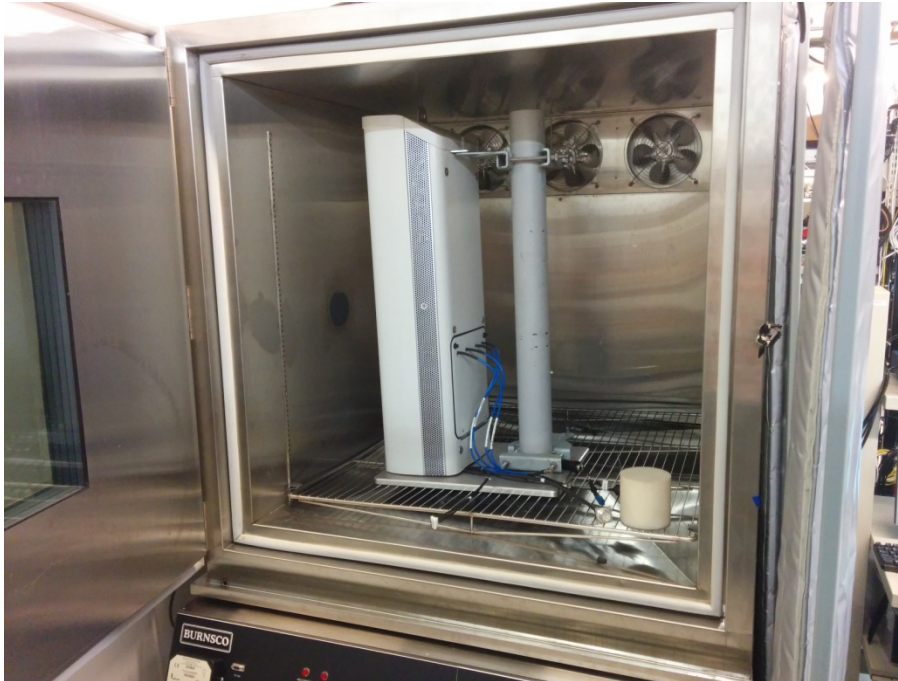
Lab Testing – Base Station in Temperature Chamber
