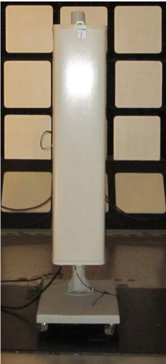
Figure 1: AIR 32 B4A B2P Test Platform for ARUS 32 B4 EMC testing and compliance assessment
