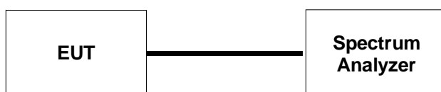
Picture 19: Test setup for spurious conducted emission measurement
