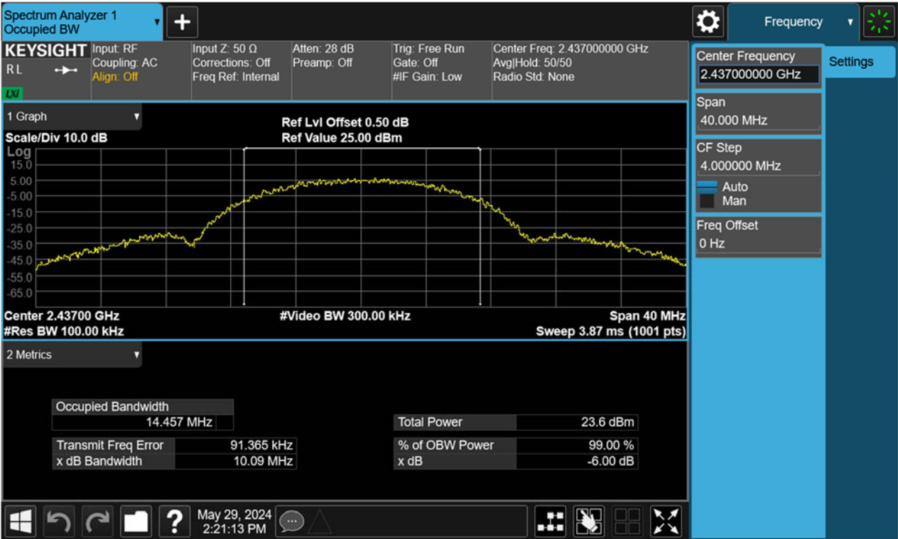
Figure 2: 6dB Bandwidth, 802.11b, 2437MHz
