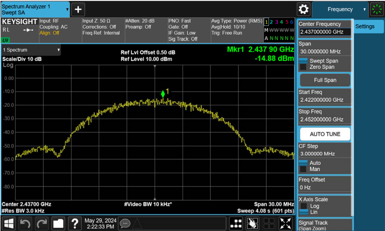
Figure 14: Power Spectral Density, 802.11b, 2437MHz
