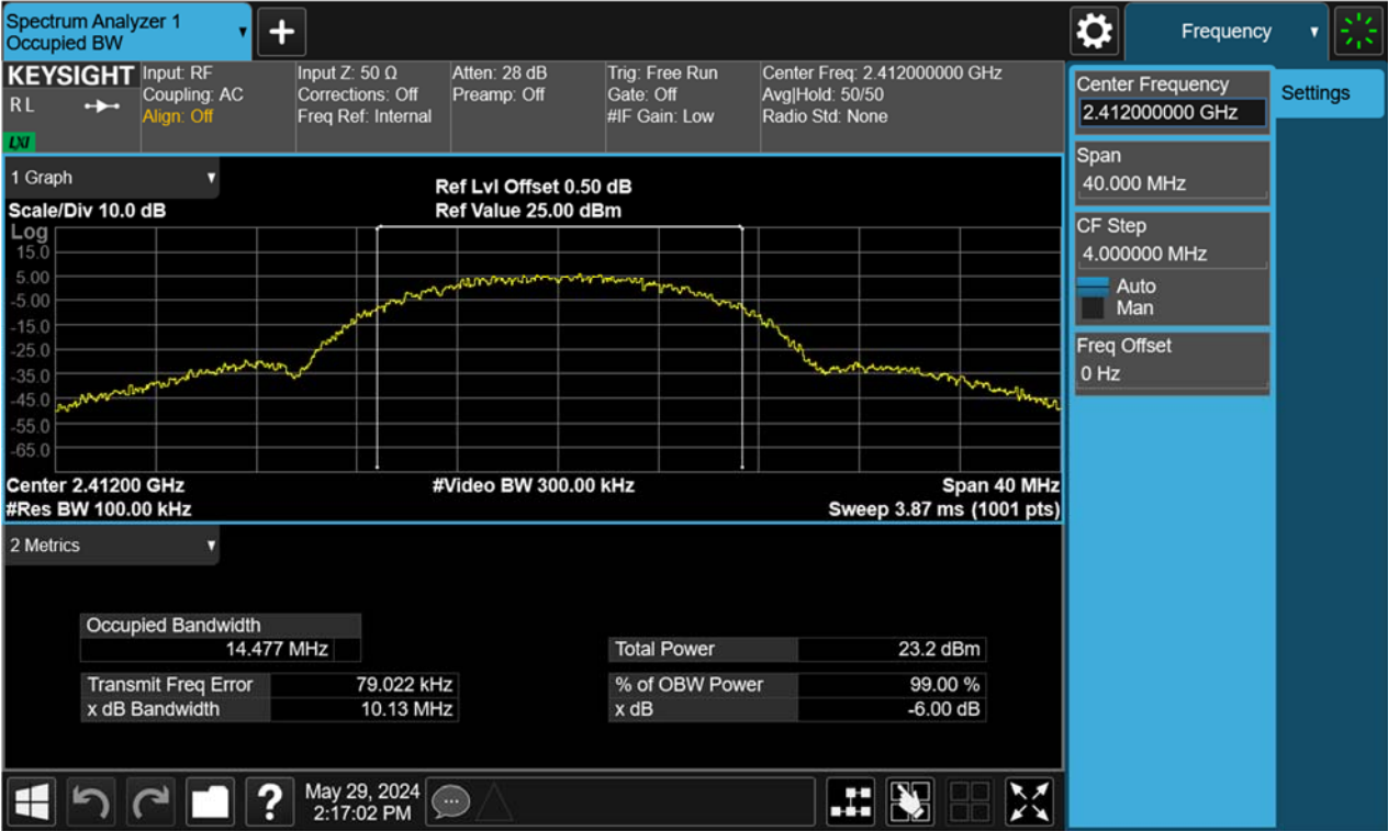
Figure 2: 6dB Bandwidth, 802.11b, 2437MHz
