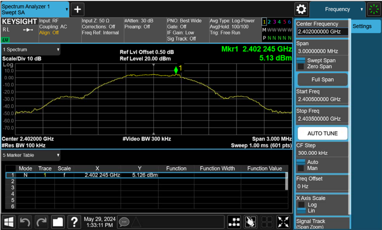
Figure 67: Conducted Spurious Emission & Authorized-band band-edge, 2402MHz, BLE-1Mbps Carrier Level
