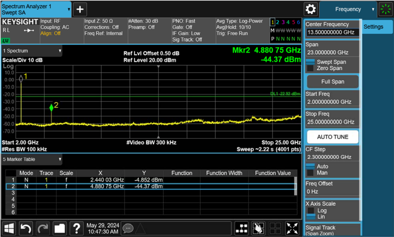
Figure 66: Conducted Spurious Emission & Authorized-band band-edge, 2480MHz, BLE-2Mbps Carrier Level
