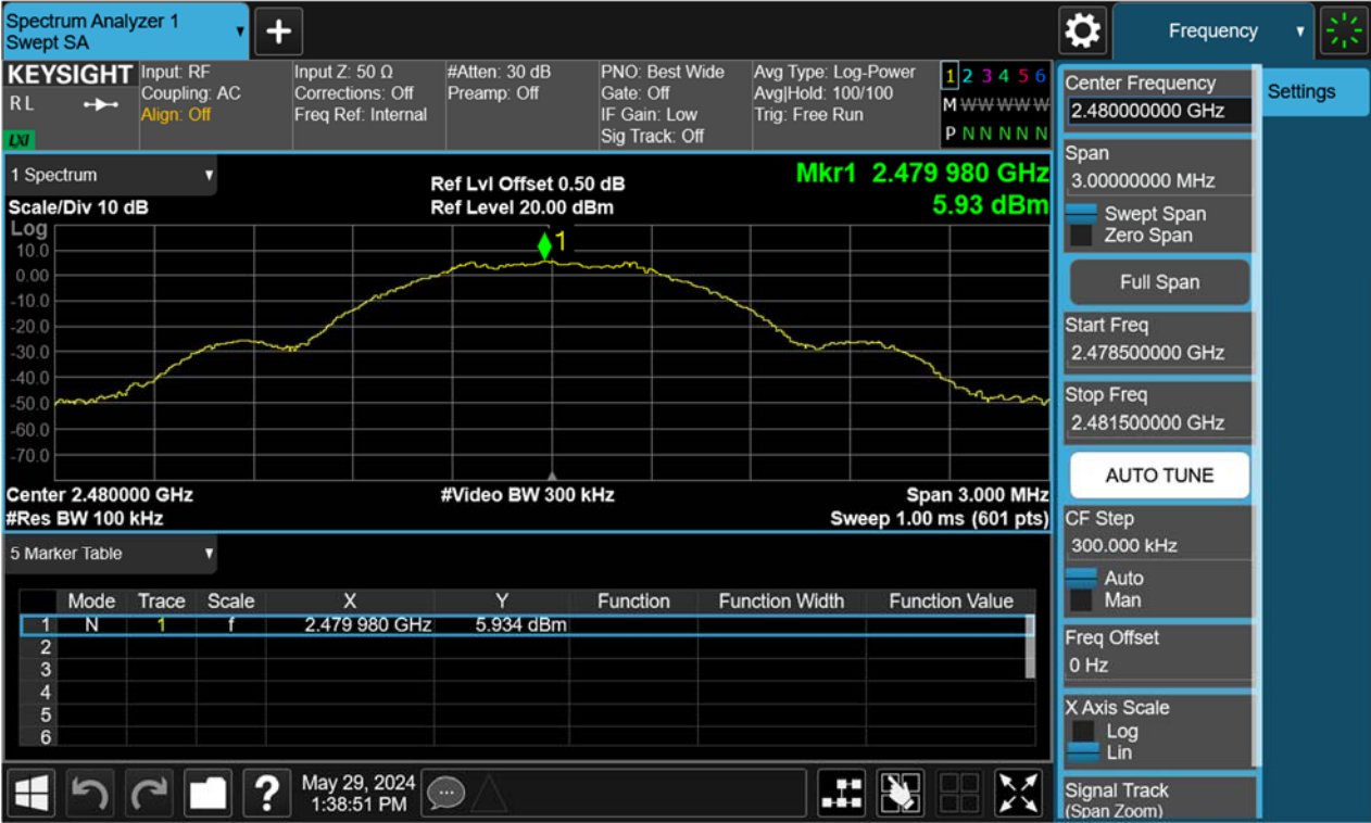
Figure 69: Conducted Spurious Emission & Authorized-band band-edge, 2480MHz, BLE-1Mbps Carrier Level
