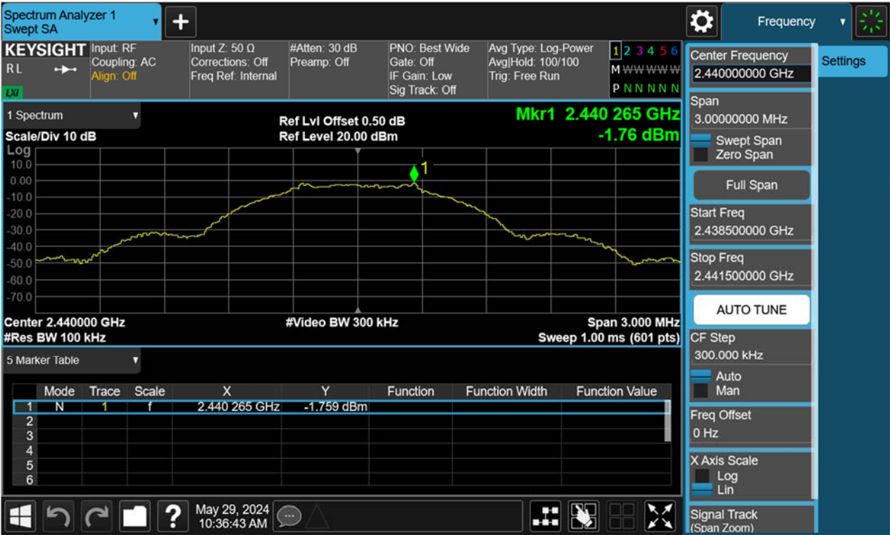
Figure 62: Conducted Spurious Emission & Authorized-band band-edge, 2440MHz, BLE-1Mbps Carrier Level
