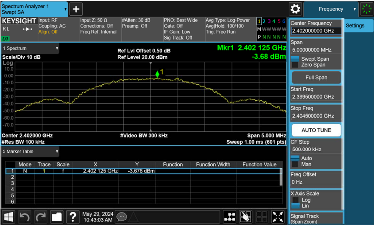
Figure 64: Conducted Spurious Emission & Authorized-band band-edge, 2402MHz, BLE-2Mbps Carrier Level
