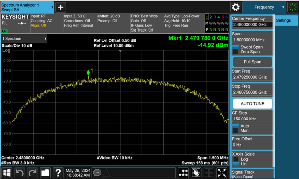
Figure 46: Power Spectral Density, 2402MHz, BLE-2Mbps
