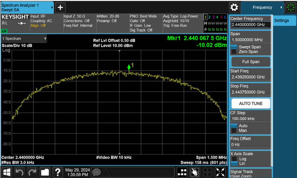
Figure 50: Power Spectral Density, 2440MHz, BLE-1Mbps
