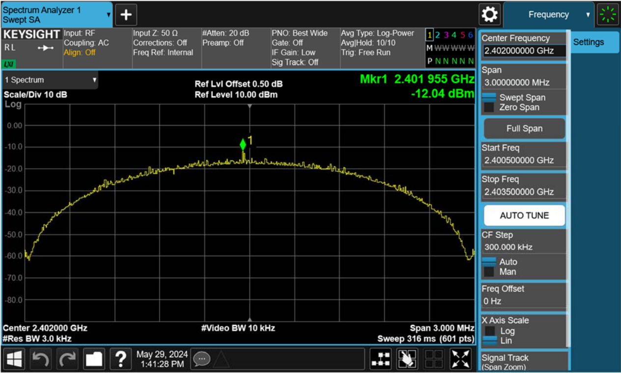
Figure 52: Power Spectral Density, 2402MHz, BLE-2Mbps
