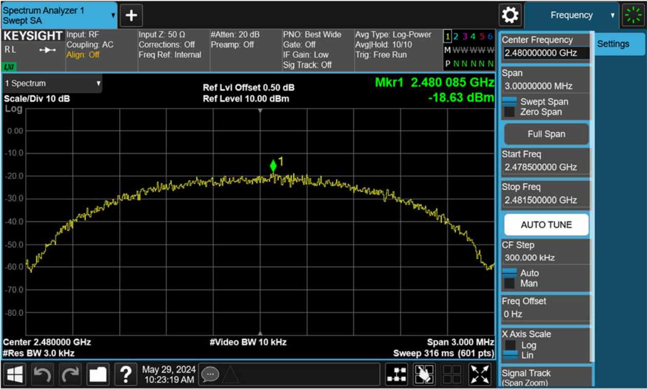
Figure 42: Power Spectral Density, 2480MHz, BLE-2Mbps
