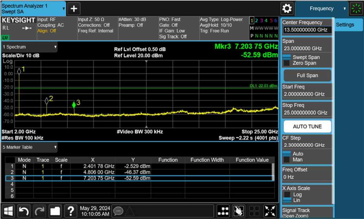
Figure 56: Conducted Spurious Emission & Authorized-band band-edge, 2440MHz, BLE-1Mbps Carrier Level
