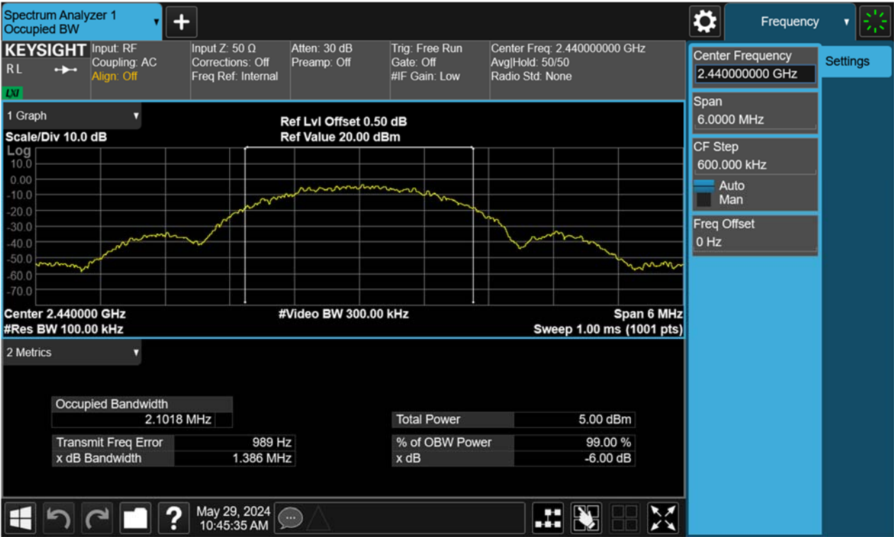
Figure 30: 6dB Bandwidth, 2480MHz, BLE-2Mbps
