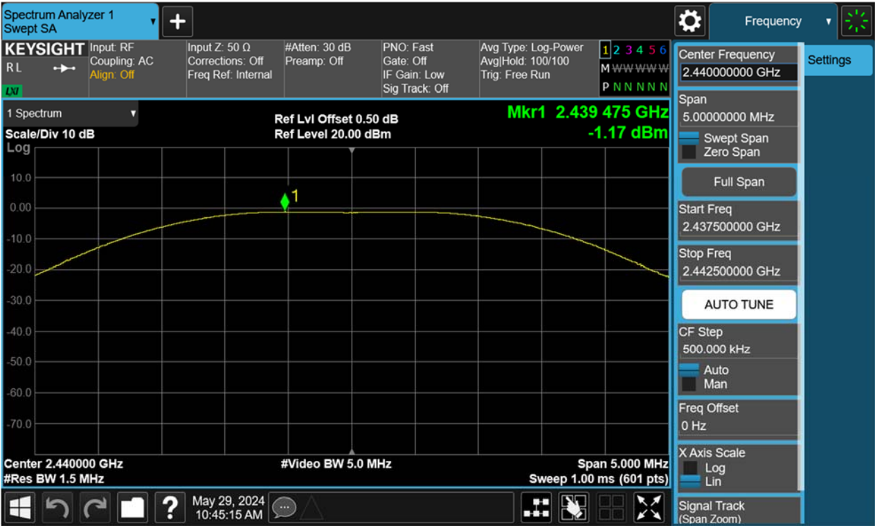
Figure 12: Peak Output Power, 2480MHz, BLE-2Mbps
