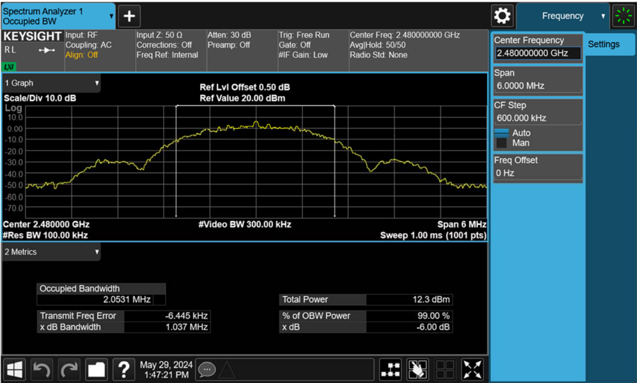
Figure 36: 6dB Bandwidth, 2480MHz, BLE-2Mbps
