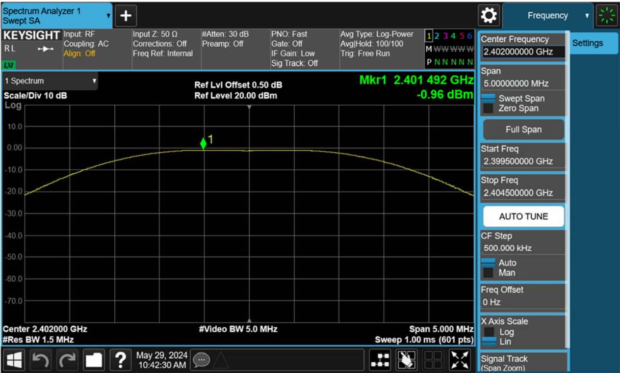
Figure 10: Peak Output Power, 2402MHz, BLE-2Mbps
