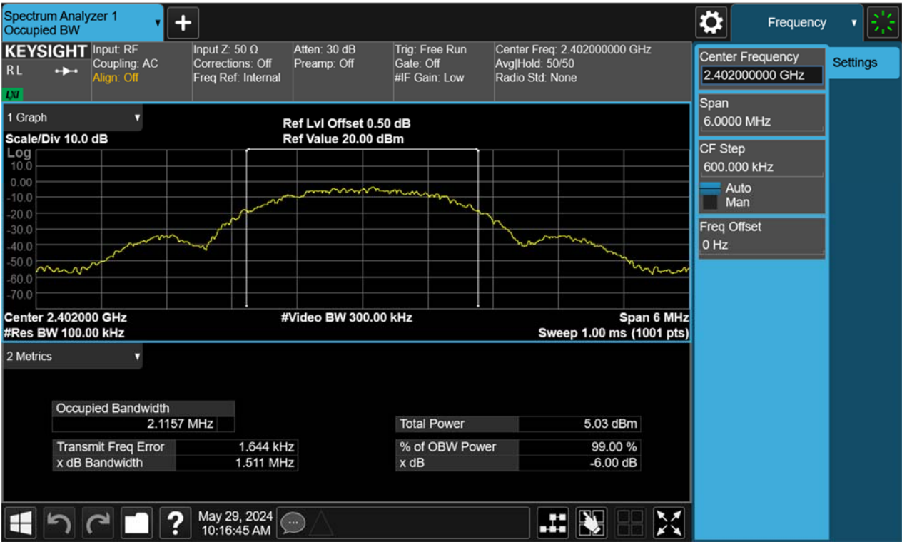
Figure 22: 6dB Bandwidth, 2402MHz, BLE-2Mbps
