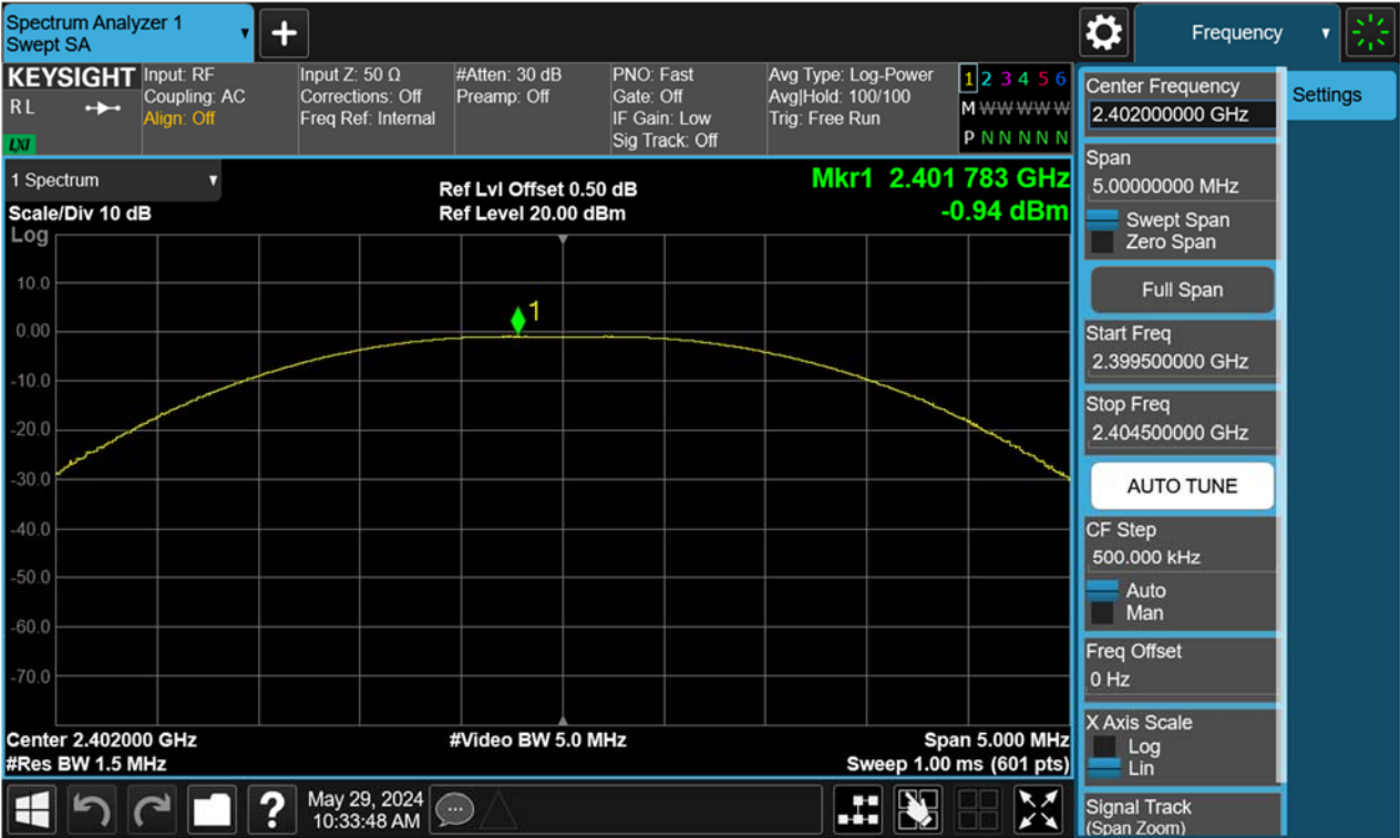
Figure 8: Peak Output Power, 2440MHz, BLE-1Mbps
