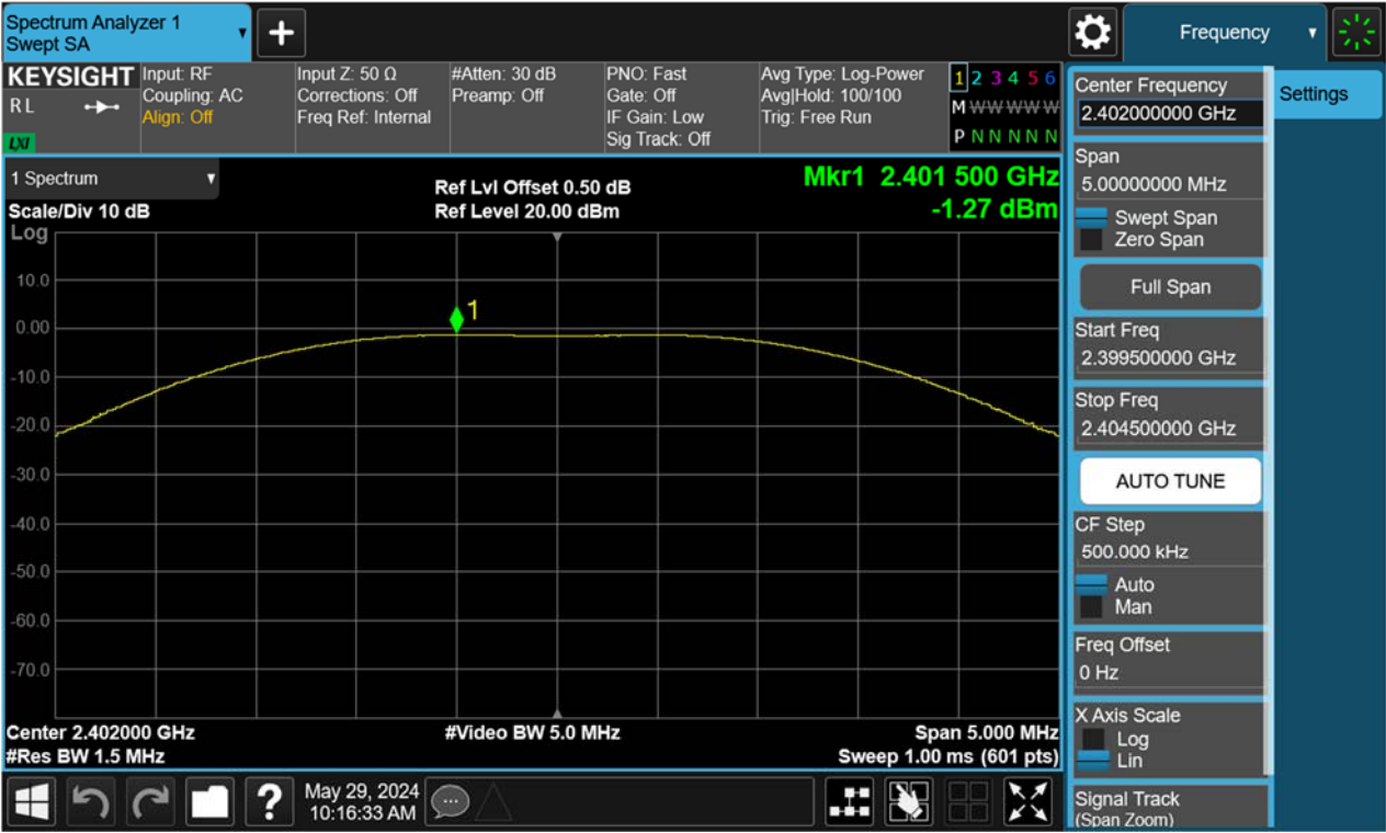
Figure 4: Peak Output Power, 2402MHz, BLE-2Mbps
