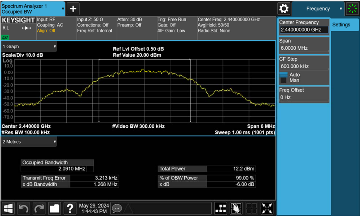
Figure 36: 6dB Bandwidth, 2480MHz, BLE-2Mbps
