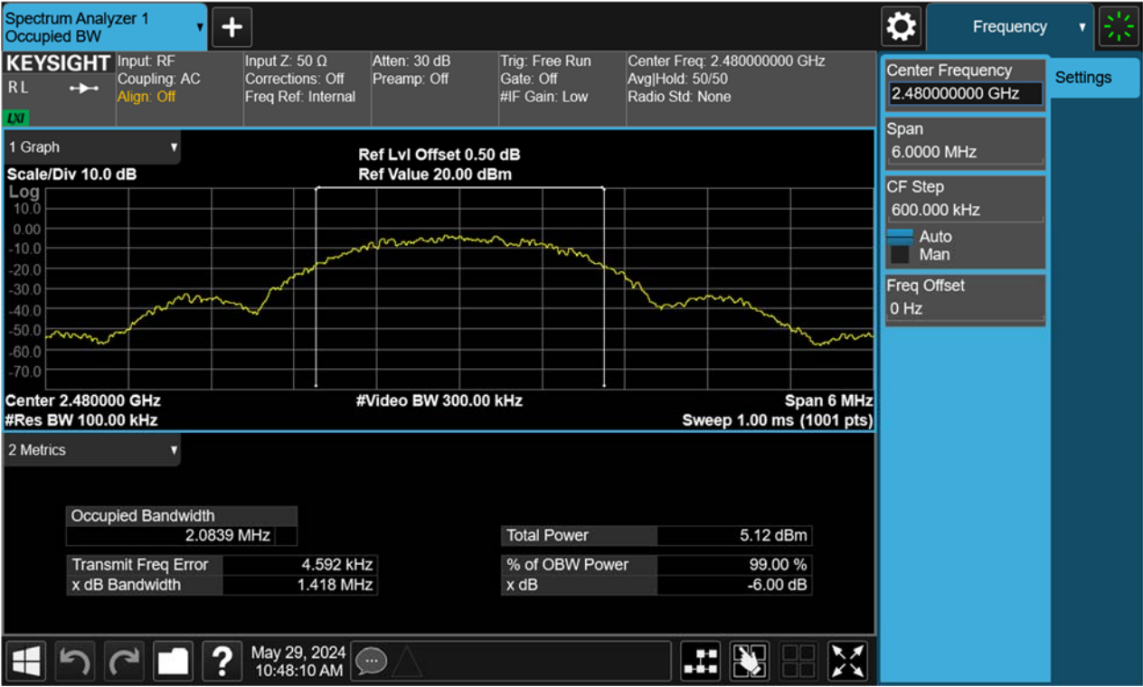
Figure 30: 6dB Bandwidth, 2480MHz, BLE-2Mbps
