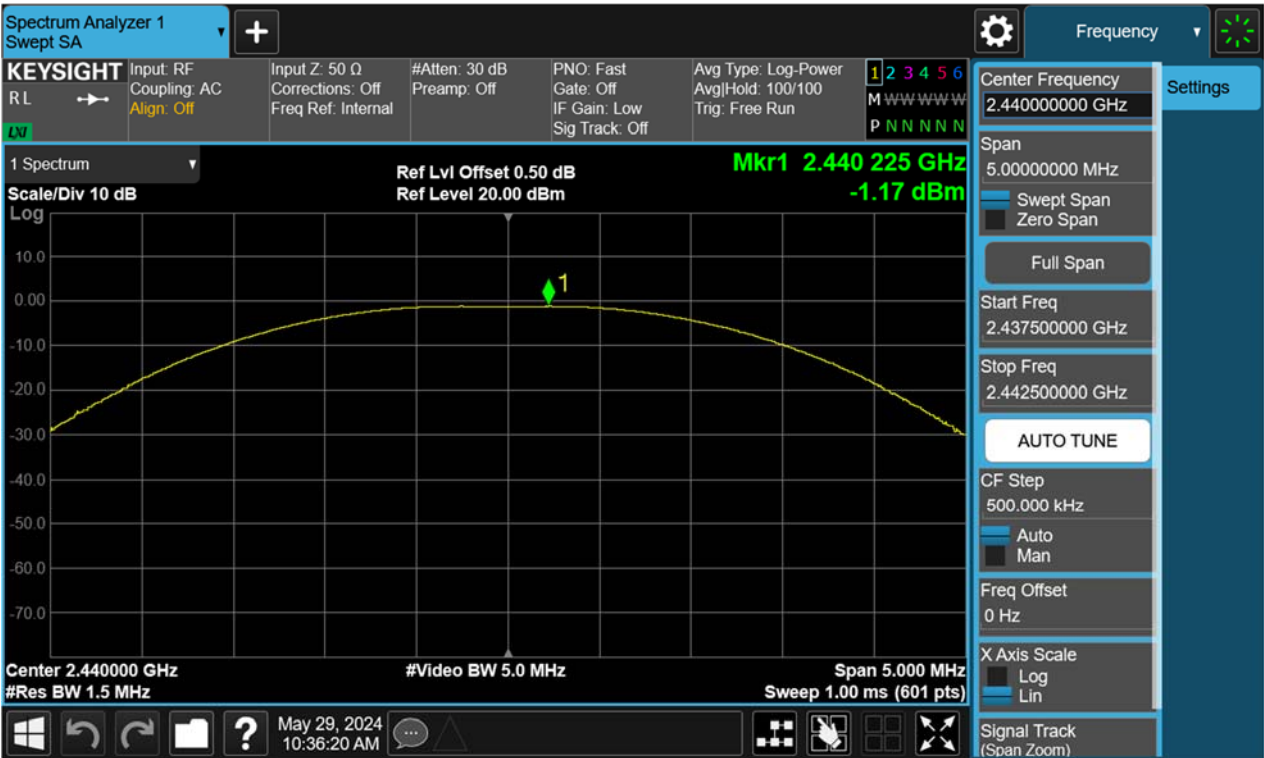
Figure 8: Peak Output Power, 2440MHz, BLE-1Mbps
