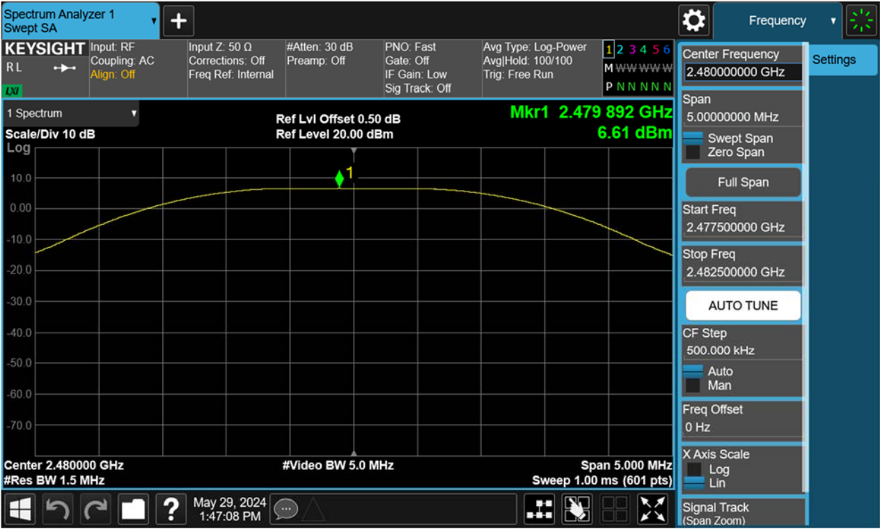
Figure 18: Peak Output Power, 2480MHz, BLE-2Mbps
