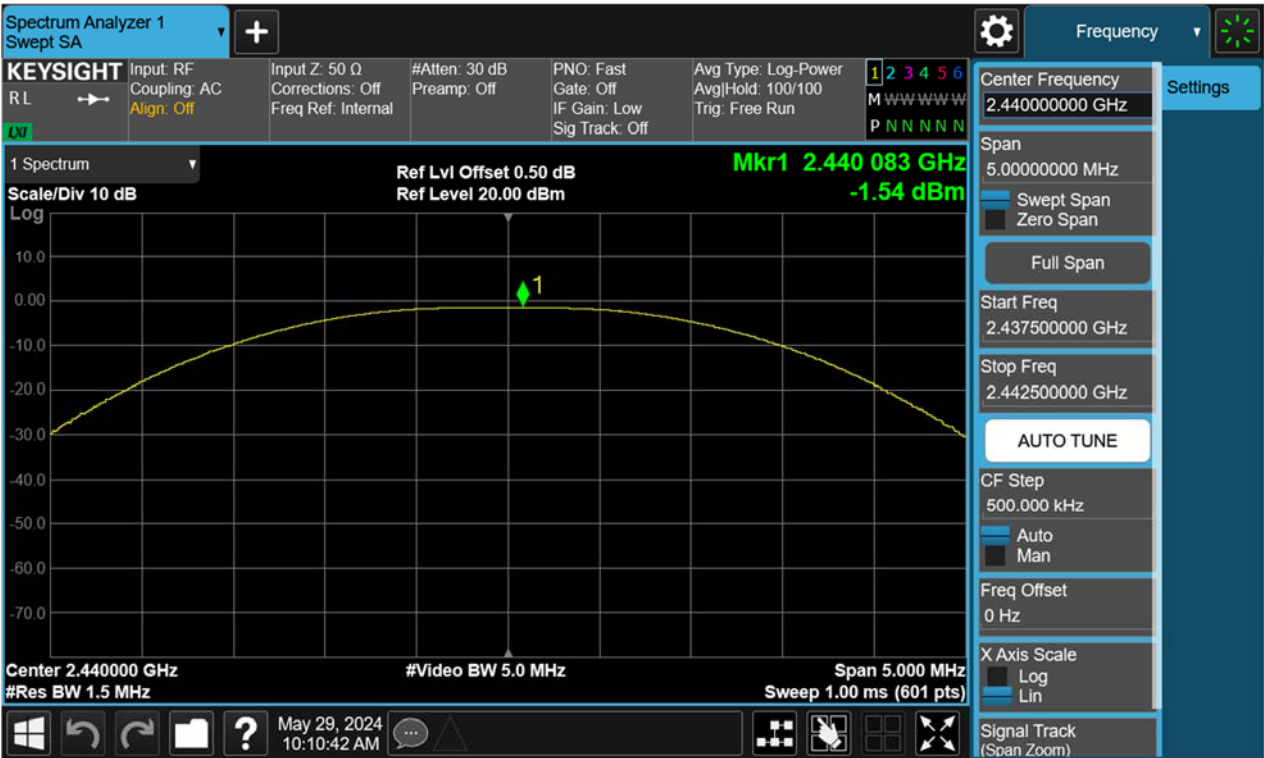
Figure 2: Peak Output Power, 2440MHz, BLE-1Mbps
