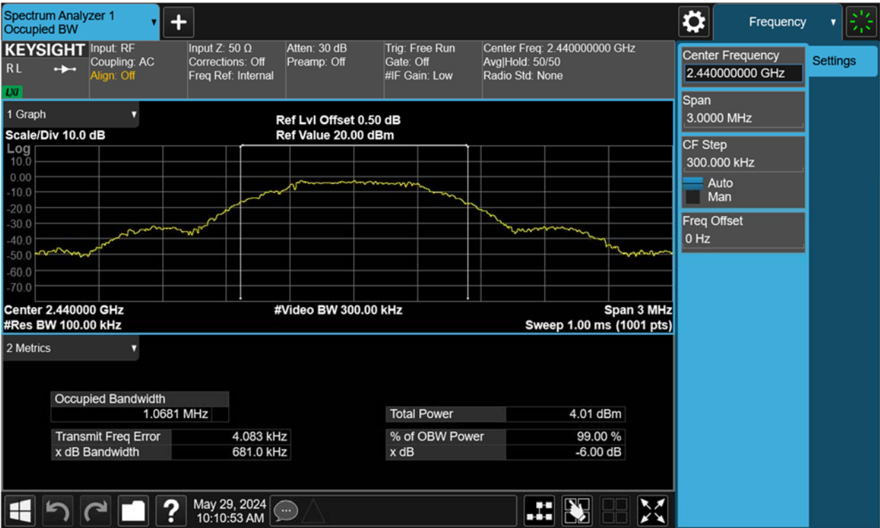
Figure 20: 6dB Bandwidth, 2440MHz, BLE-1Mbps
