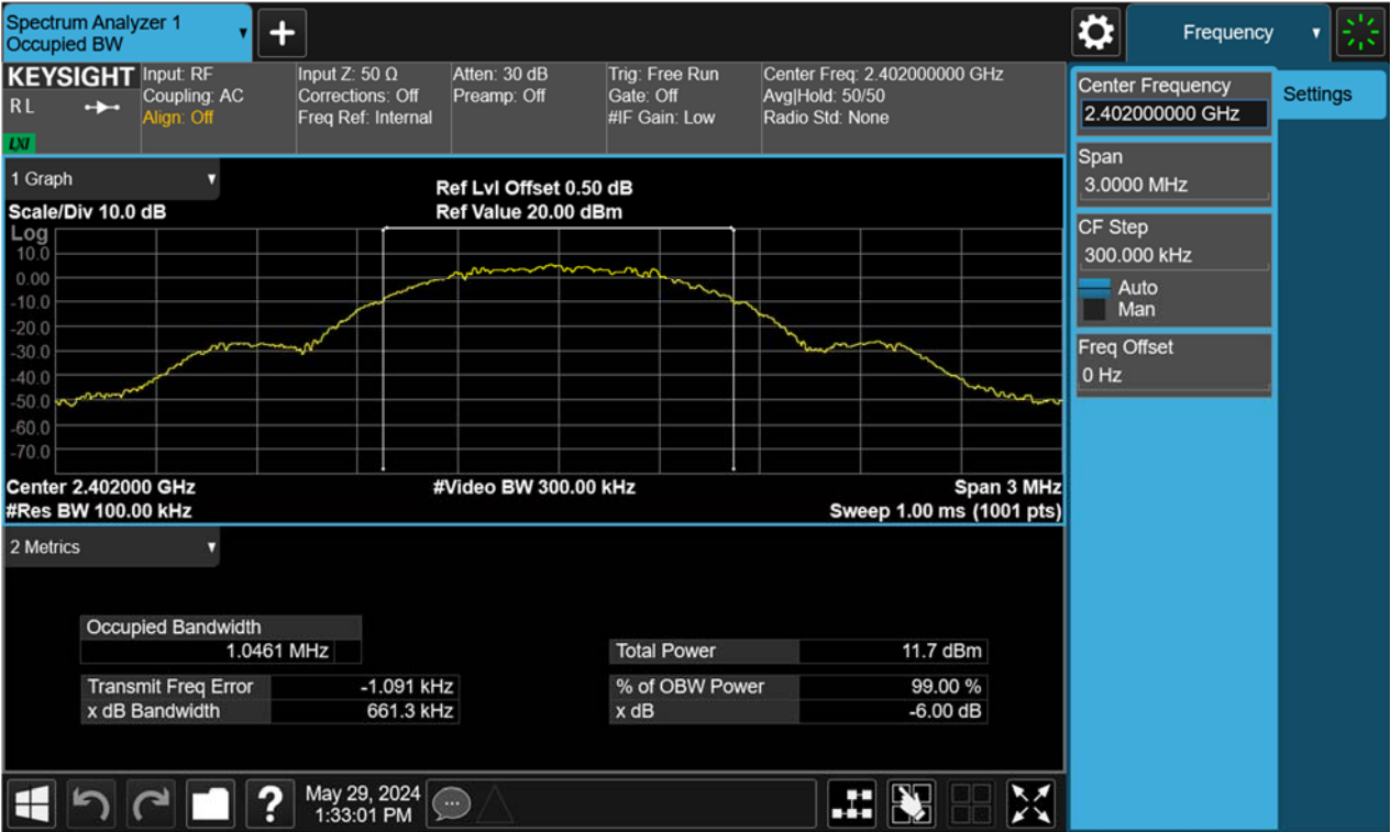
Figure 32: 6dB Bandwidth, 2440MHz, BLE-1Mbps
