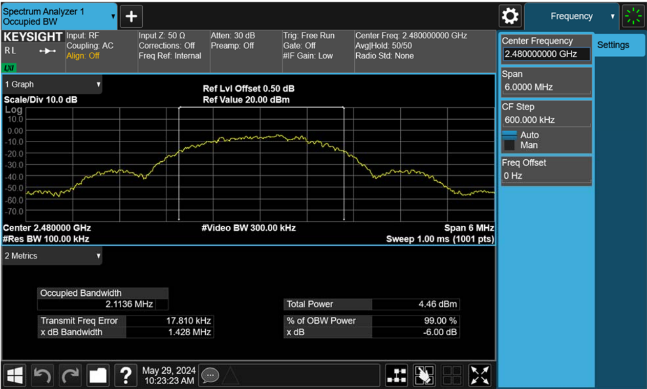
Figure 24: 6dB Bandwidth, 2480MHz, BLE-2Mbps
