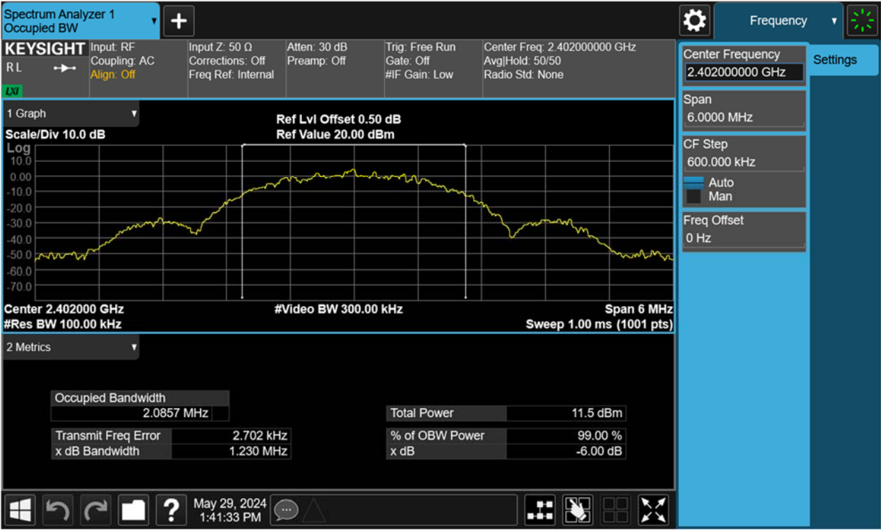
Figure 34: 6dB Bandwidth, 2402MHz, BLE-2Mbps
