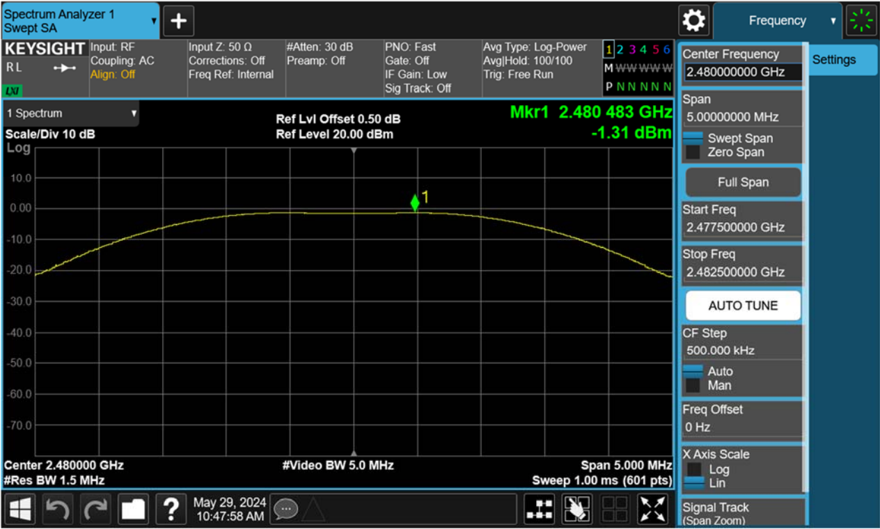
Figure 12: Peak Output Power, 2480MHz, BLE-2Mbps
