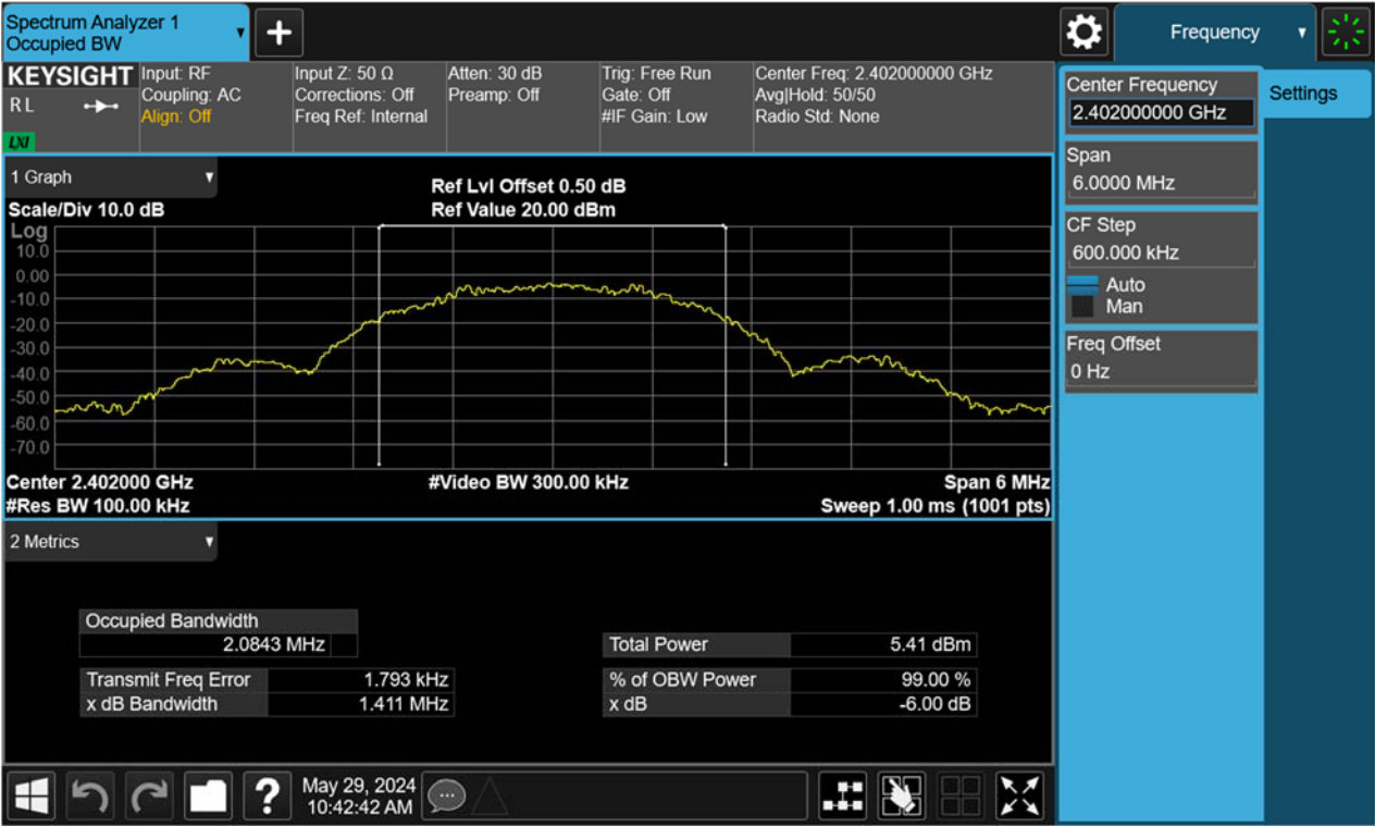
Figure 28: 6dB Bandwidth, 2402MHz, BLE-2Mbps
