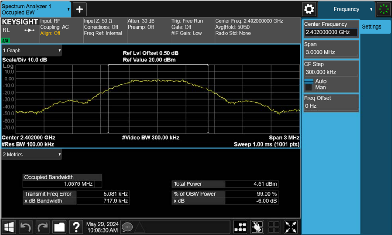
Figure 20: 6dB Bandwidth, 2440MHz, BLE-1Mbps
