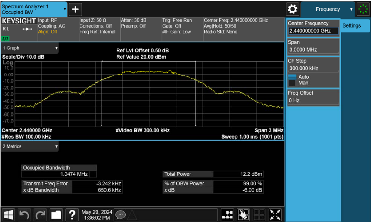
Figure 32: 6dB Bandwidth, 2440MHz, BLE-1Mbps
