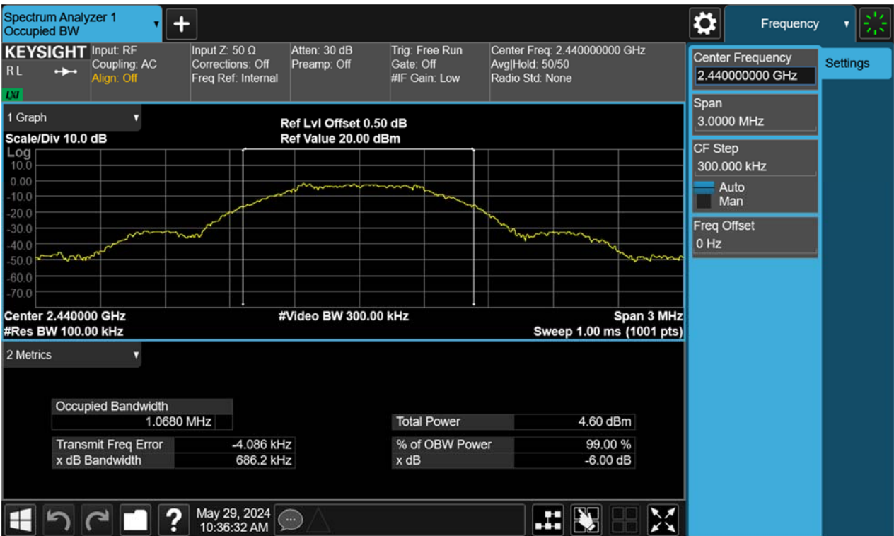
Figure 26: 6dB Bandwidth, 2440MHz, BLE-1Mbps
