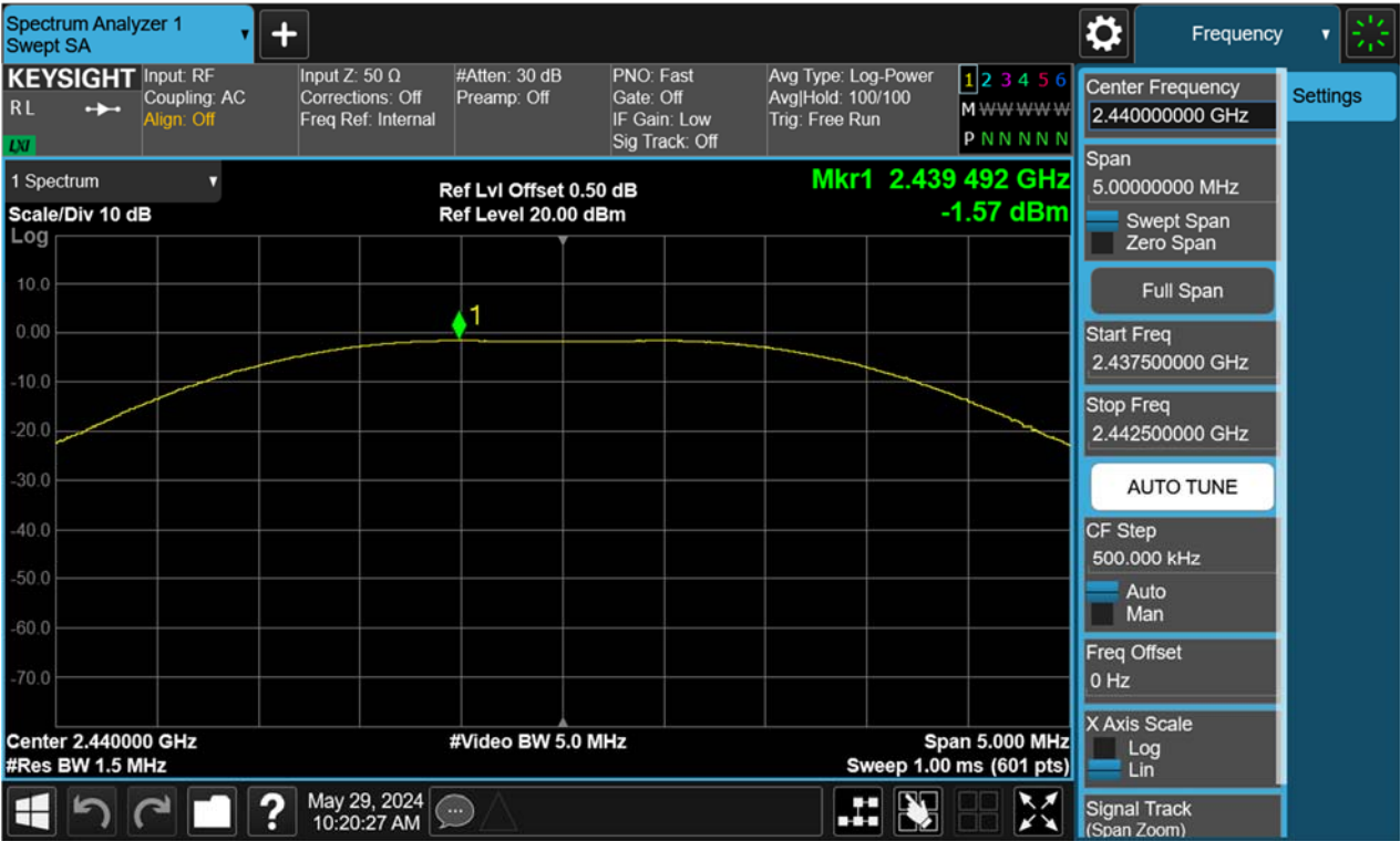
Figure 6: Peak Output Power, 2480MHz, BLE-2Mbps
