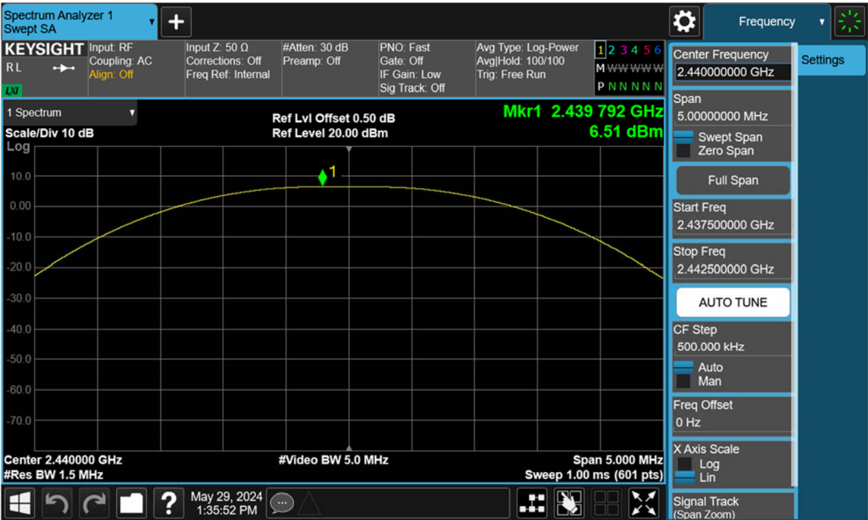
Figure 14: Peak Output Power, 2440MHz, BLE-1Mbps
