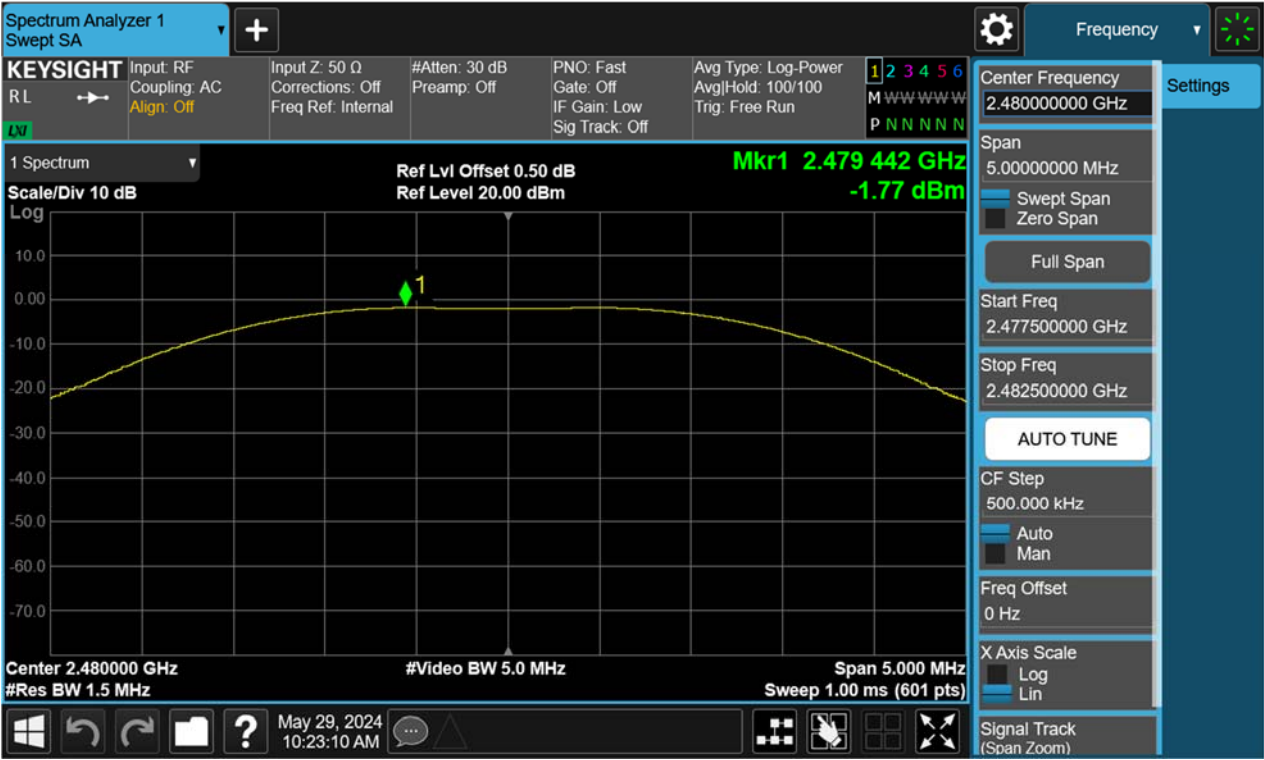
Figure 6: Peak Output Power, 2480MHz, BLE-2Mbps
