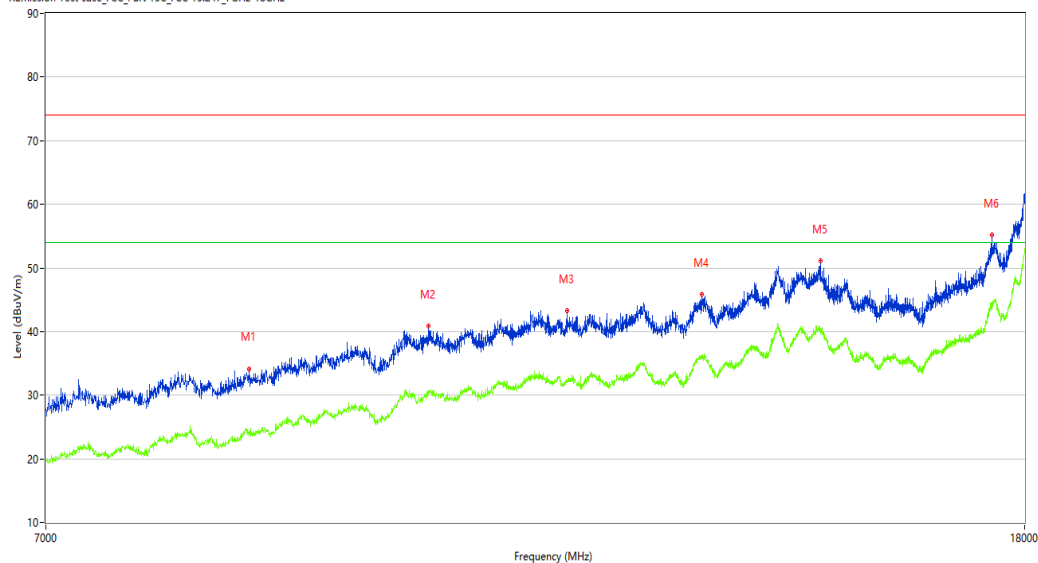
REmission Test case_FCC_Part 15C_FCC 15.247_7GHz-18GHz
