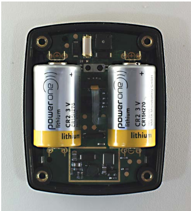
Figure 3.1. Battery polarity and replacement
