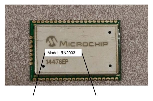
Model number will be laser etched on RF shield on top of PCB assembly.
